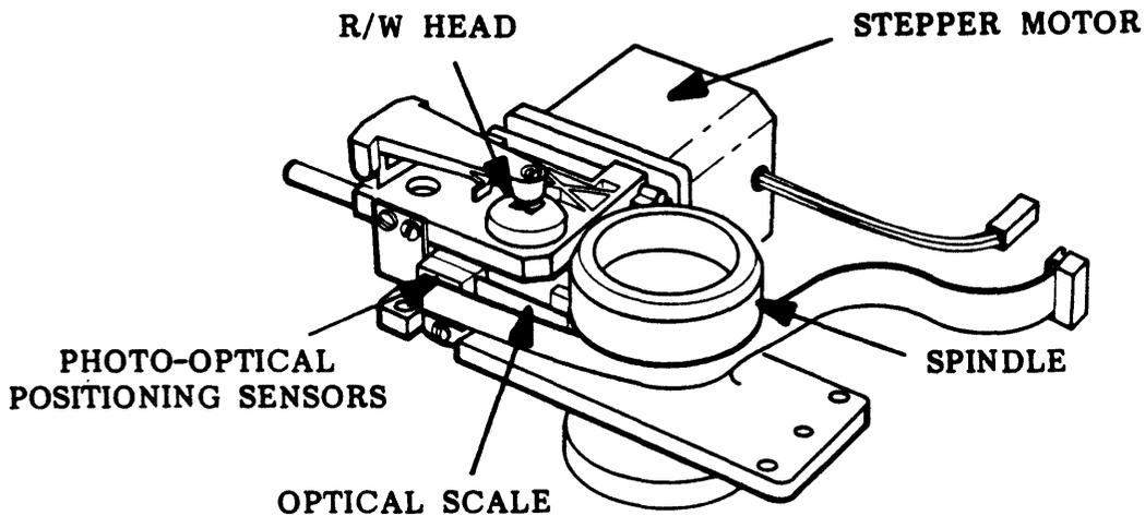
Since the stepper motor is controlled by the on-board microprocessor a number of stepping techniques are possible with appropriate firmware. This also facilitates easy system integration. The Amlyn device can operate in three modes of operation, all user transparent.
