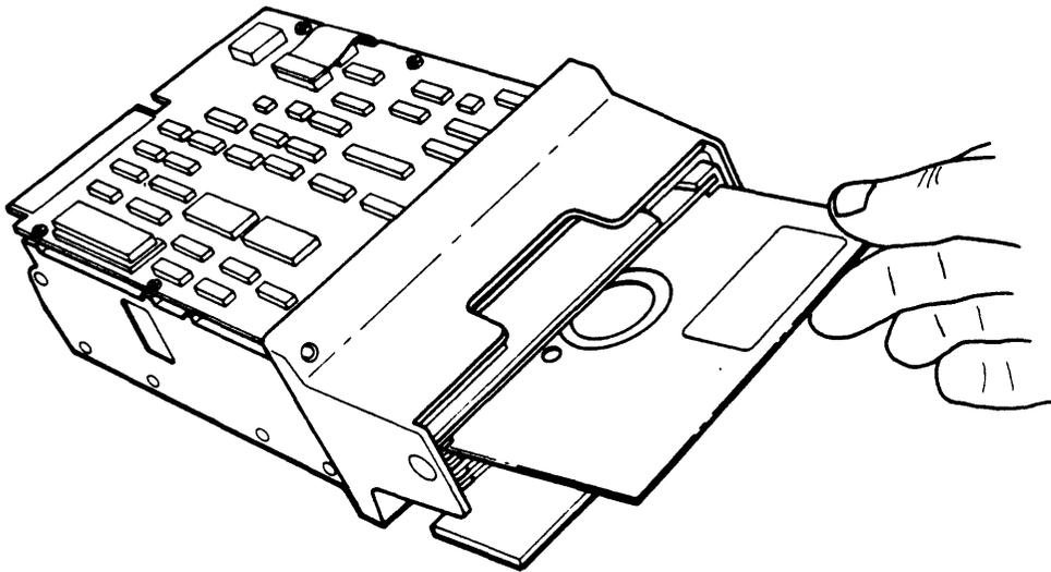
To reliably achieve a track density of 170 tracks-per-inch each diskette is pre-recorded with a "reference track" located outside of track 0. See Figure 4. The reference track serves as a known point from which all data tracks are located. Since the reference track is located on the diskette and subsequently travels with it, interchangeability of diskettes between units is assured without the need for a track 0 sensor and alignment, or any head adjustment.
