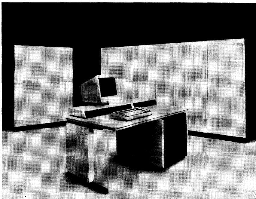
*The Amdahl 580 Series of high-performance mainframes includes the single-processor 5860, shown here, with twice the power of Amdahl's 470V/8, the attached-processor 5870, with 70 percent more power than the 5860, and the dual-processor 5880, with 3.5 times the 470V/8's performance. The systems have from 16 to 32 megabytes of main memory, 16 to 32 channels, and improved price/performance over the IBM 3081.*
