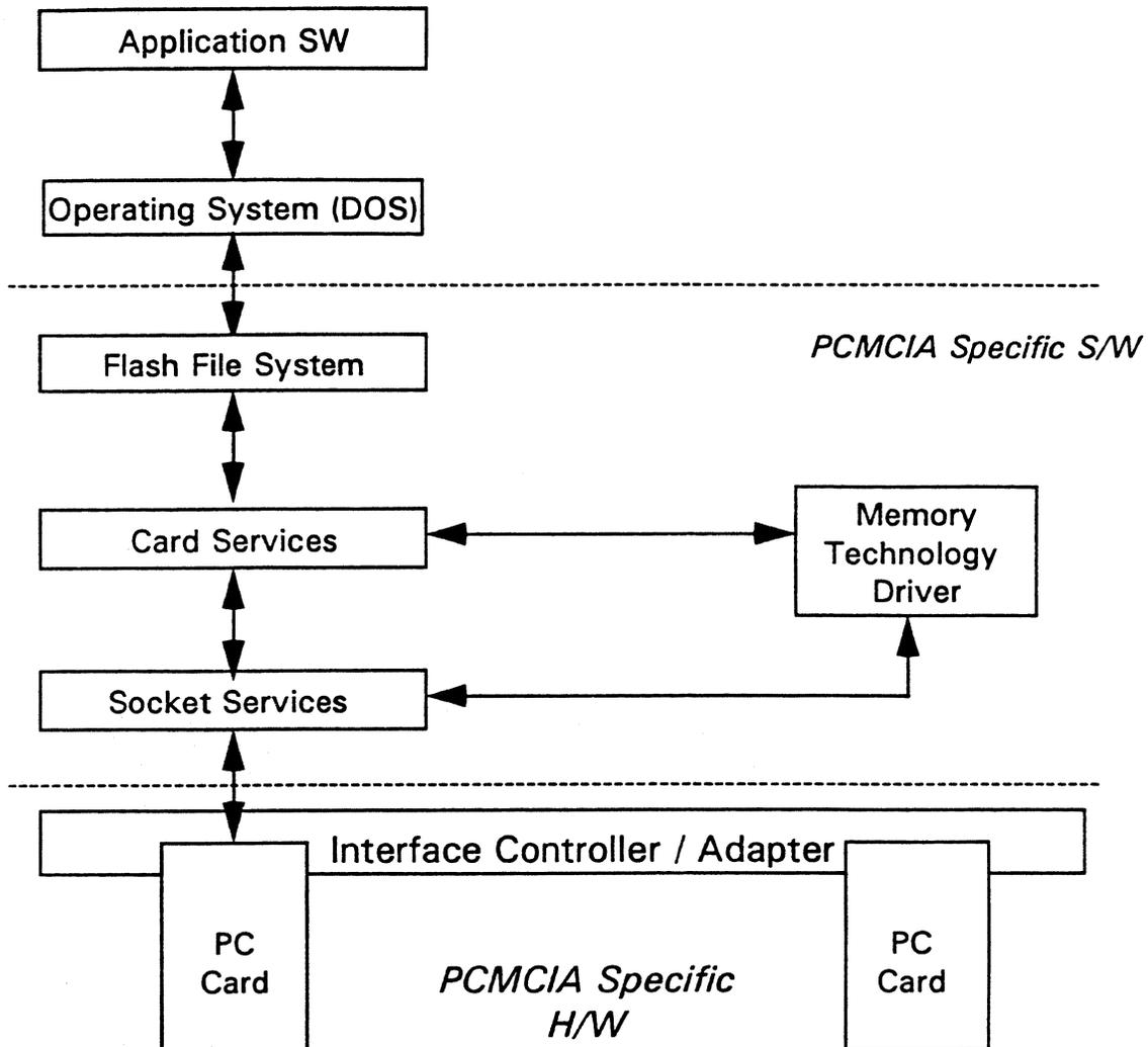
**Figure 4.2 The PCMCIA Hardware and Software Layers**
