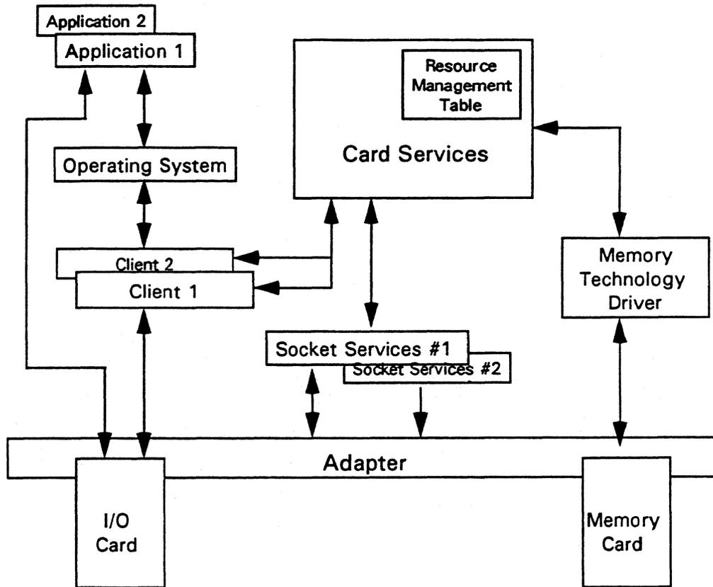
Figure 7.5 Card Services Software Architecture
