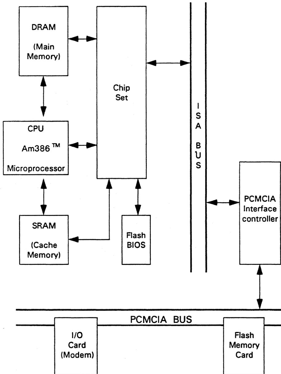
Figure 6.2 PC-AT Block Diagram with PCMCIA Support
