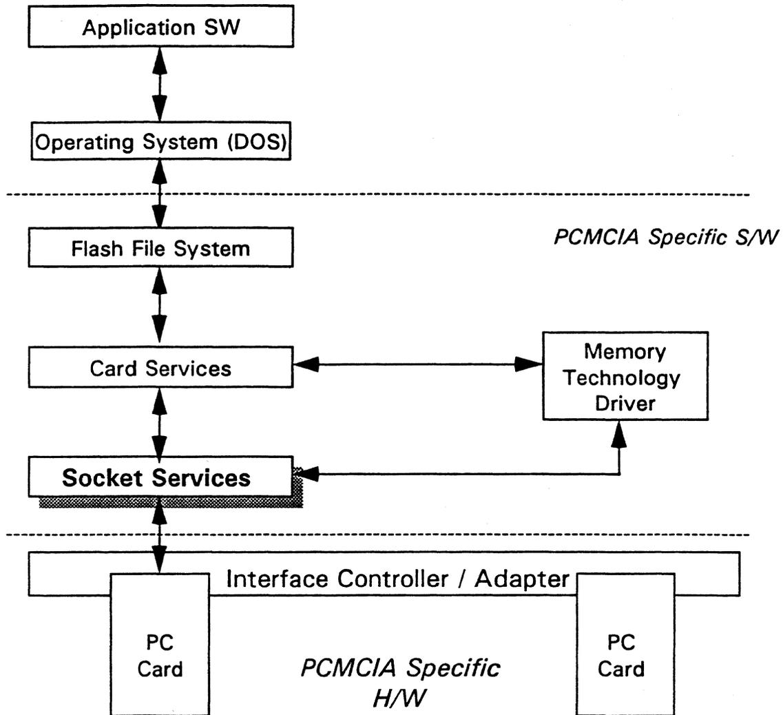
Figure 6.4 The PCMCIA Layers: Focus on Socket Services
