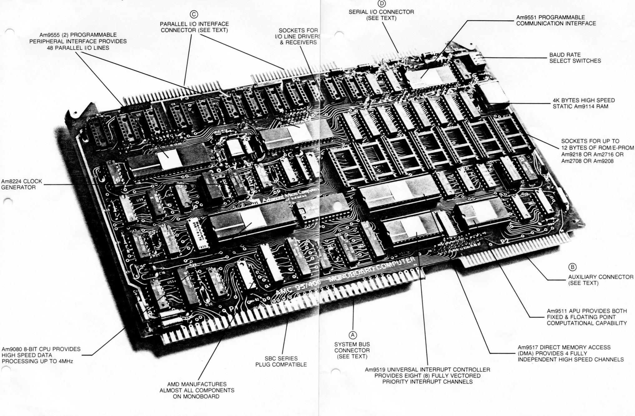
Am9555 (2) PROGRAMMABLE PERIPHERAL INTERFACE PROVIDES 48 PARALLEL I/O LINES
