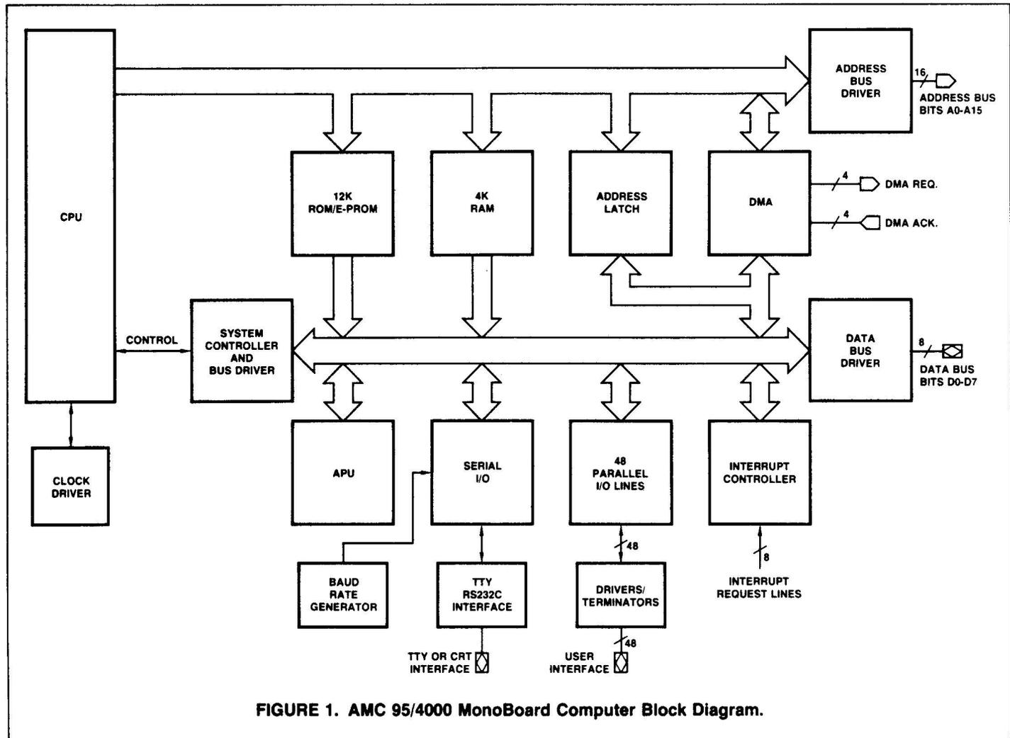
FIGURE 1. AMC 95/4000 MonoBoard Computer Block Diagram.
