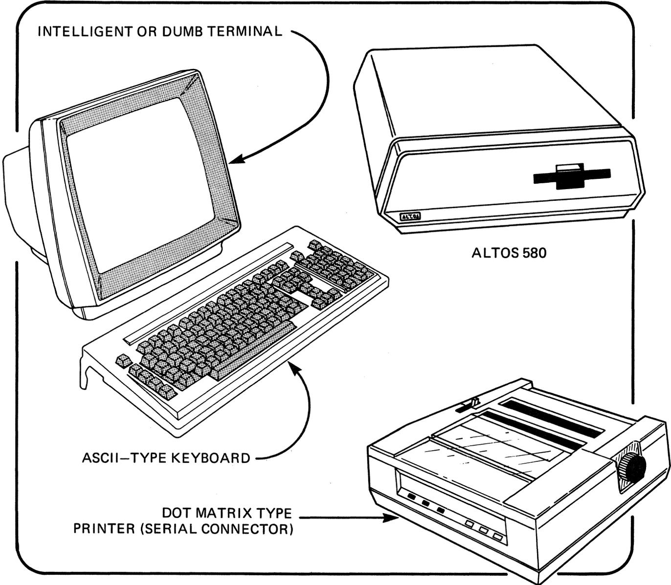
**Figure 1-1: Typical Altos 580 with Terminal(s), Printer**
