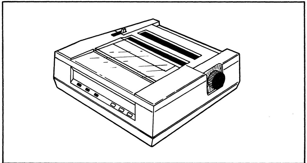
Print quality may or may not be important. If you are producing text that is to be "camera ready" for printing, you need a letter-quality printer. (Characters are produced by one stroke of a letter template against the ribbon as on a typewriter.) If you simply need readable copy, which can also be high quality, a dot-matrix printer is a less expensive option. (Characters are produced by a series of points that press against that ribbon to make up the letter.)
