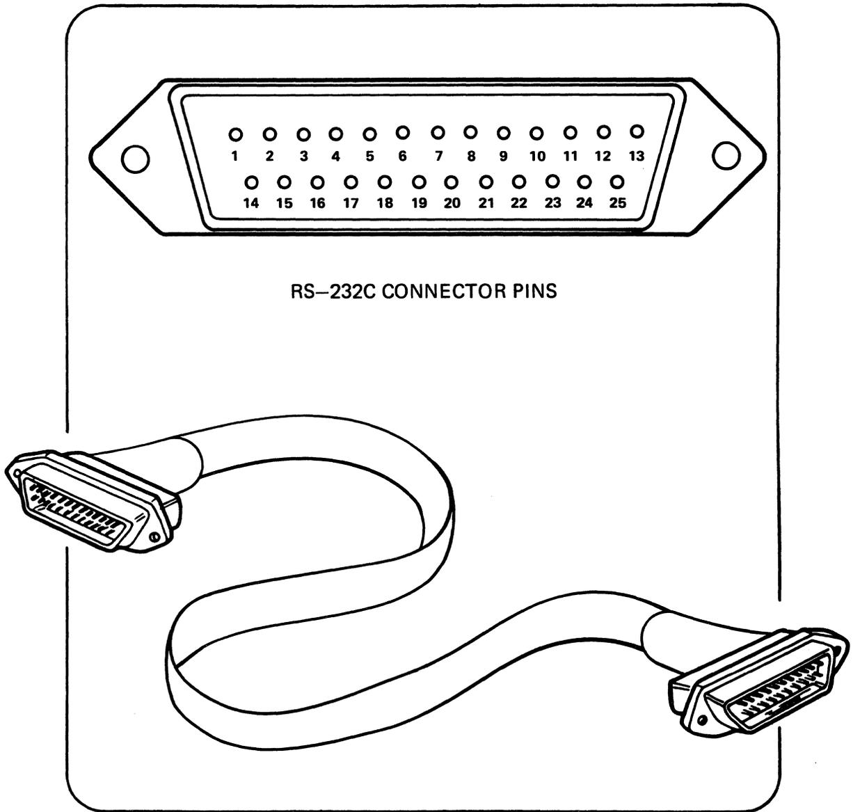
**Figure C-1: Male Connector, RS-232C Cable**
