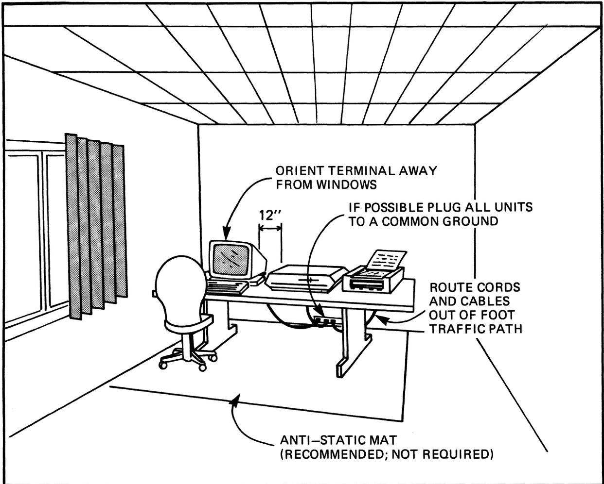
**Figure 5-1: Diagram of Computer Site**
