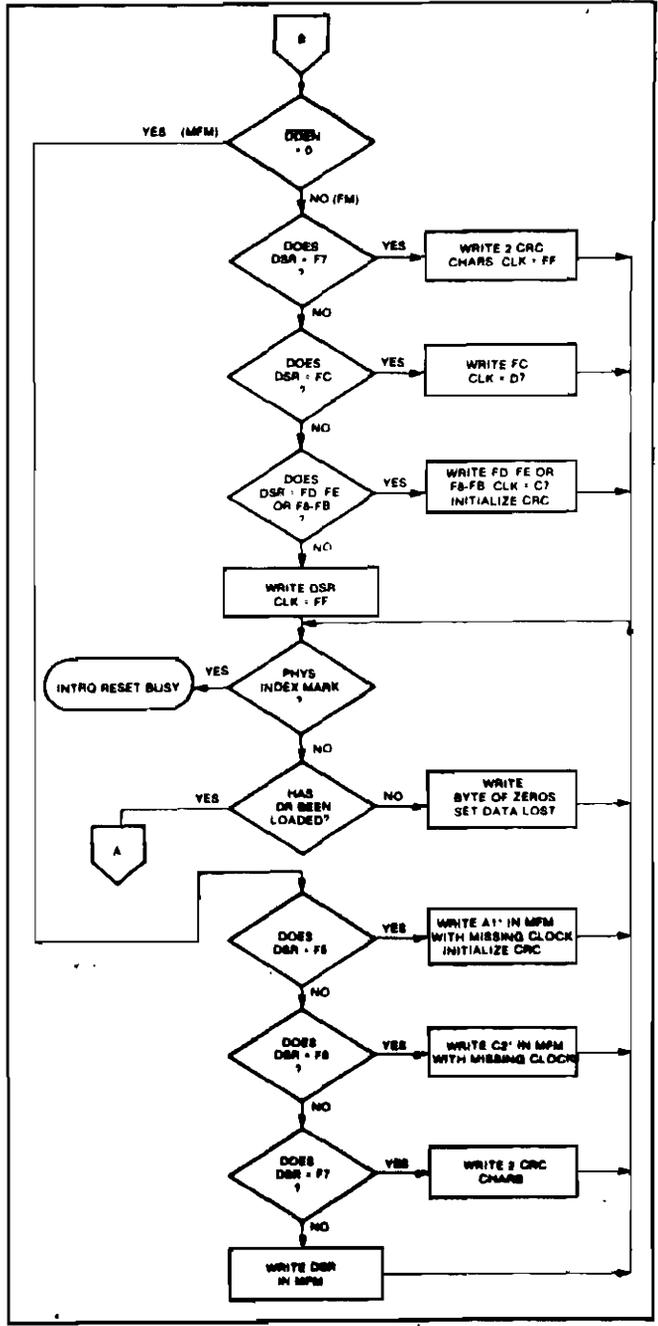
Figure 4-8. Type III Command Write Track
