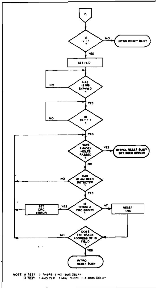
Figure 4-6. Type I Command Flow (Sh 2 of 2)
