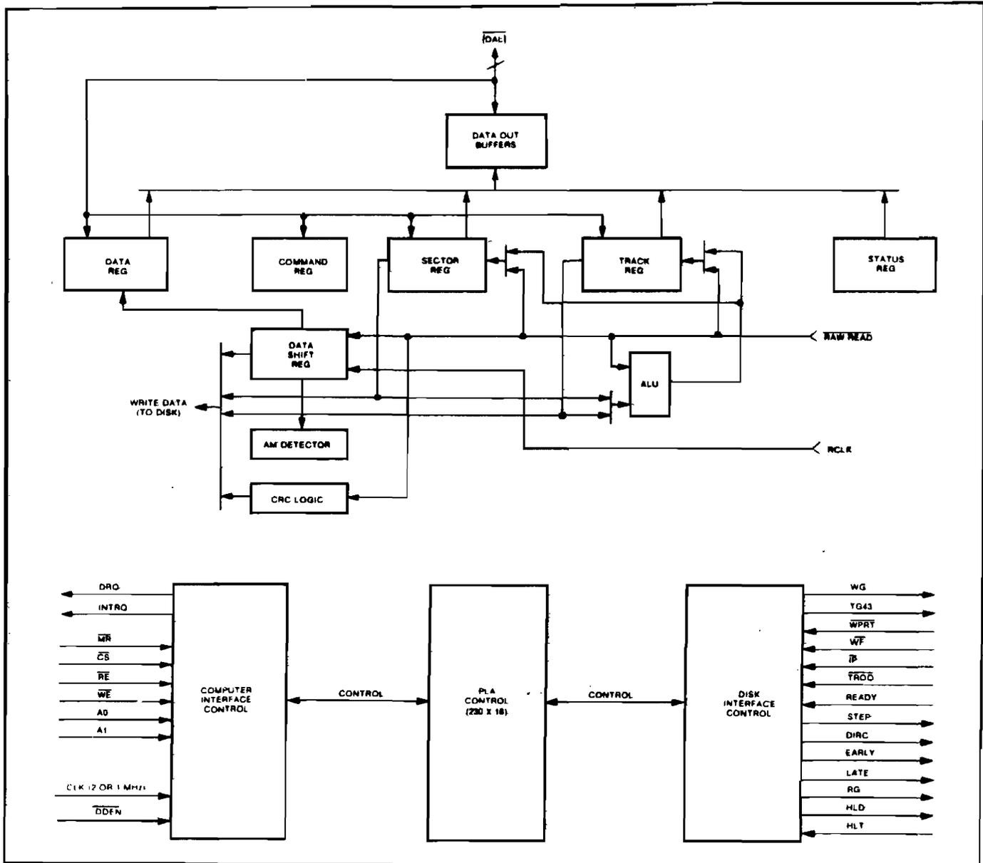
Figure 4-5. Floppy Disk Formatter/Controller Module Block Diagram
