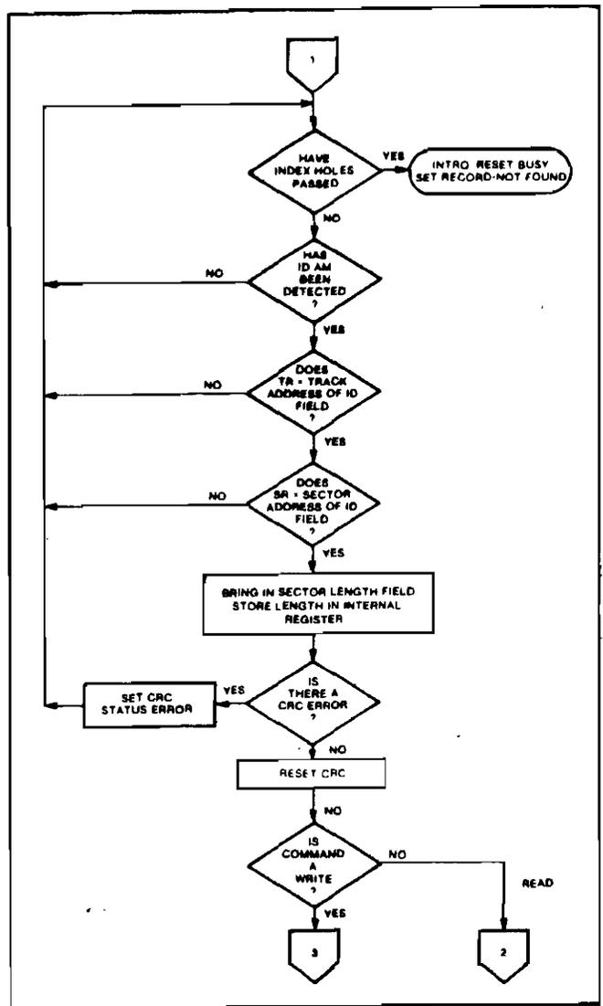
Figure 4-7. Type II Command Flow (Sh 1 of 2)
