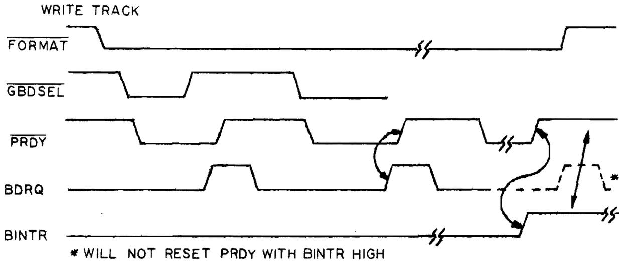
Figure 4-3. PRDY Control Logic Timing
