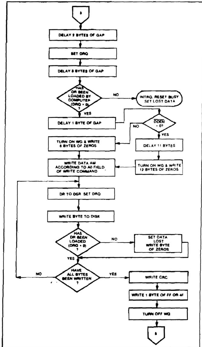
Figure 4-7. Type II Command Flow (Sh 2 of 2)
