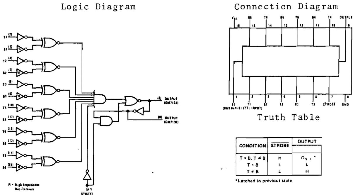
Figure 4-20. Bus Comparator Connections
