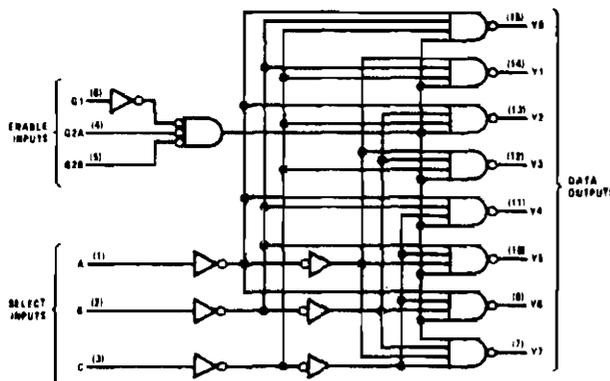
Figure 4-26. Decoder Connections
