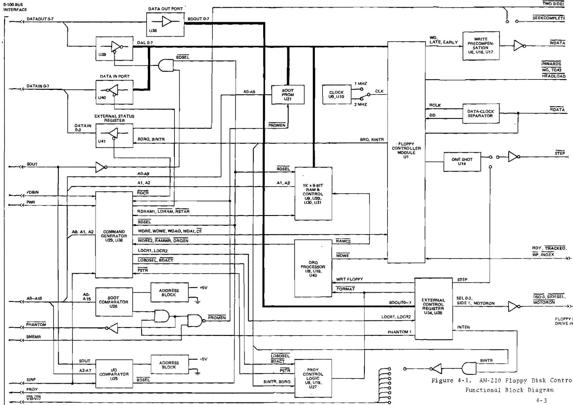
Figure 4-1. AM-210 Floppy Disk Control Functional Block Diagram
