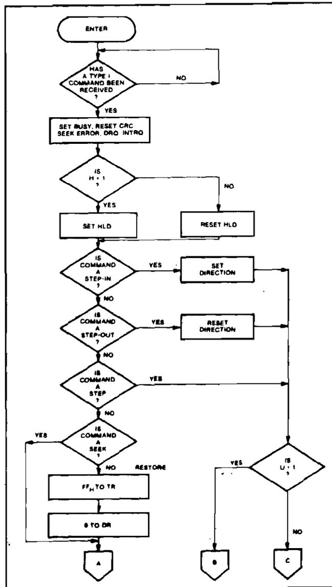
Figure 4-6. Type I Command Flow (Sh 1 of 2)
