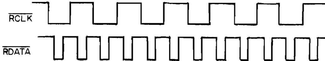
Note that RCLK will "shift" depending on the similar shift in RDATA. However, the entire trace is effectively stable when the PLO circuitry is adjusted correctly.
