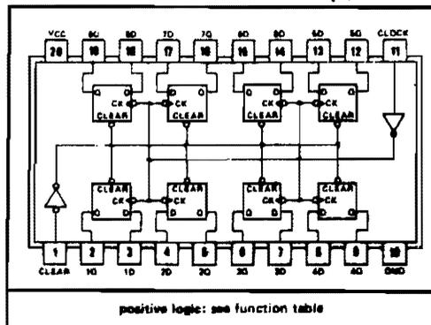
Figure 4-36. D Flip-Flop Connections
