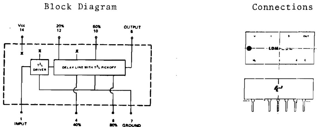
Figure 4-34. Logic Delay Module Diagram and Connections.
