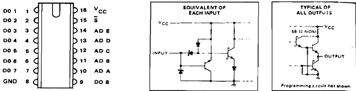
Figure 4-35. PROM Connections and I/O Circuits
