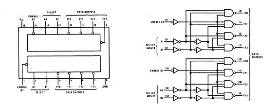
Figure 4-28. Decoder/Demultiplexer Connections
