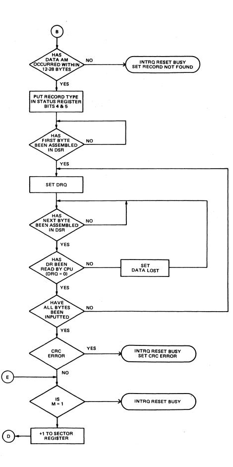
Figure 4-6. Type II Command Flow (Sh 3 of 4)
