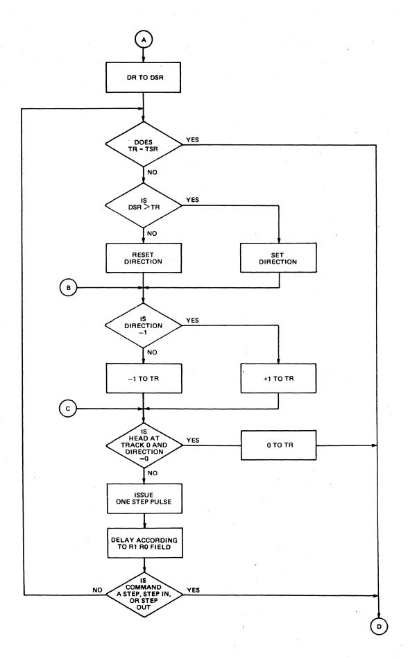
Figure 4-5. Type I Command Flow (Sh 2 of 3)
