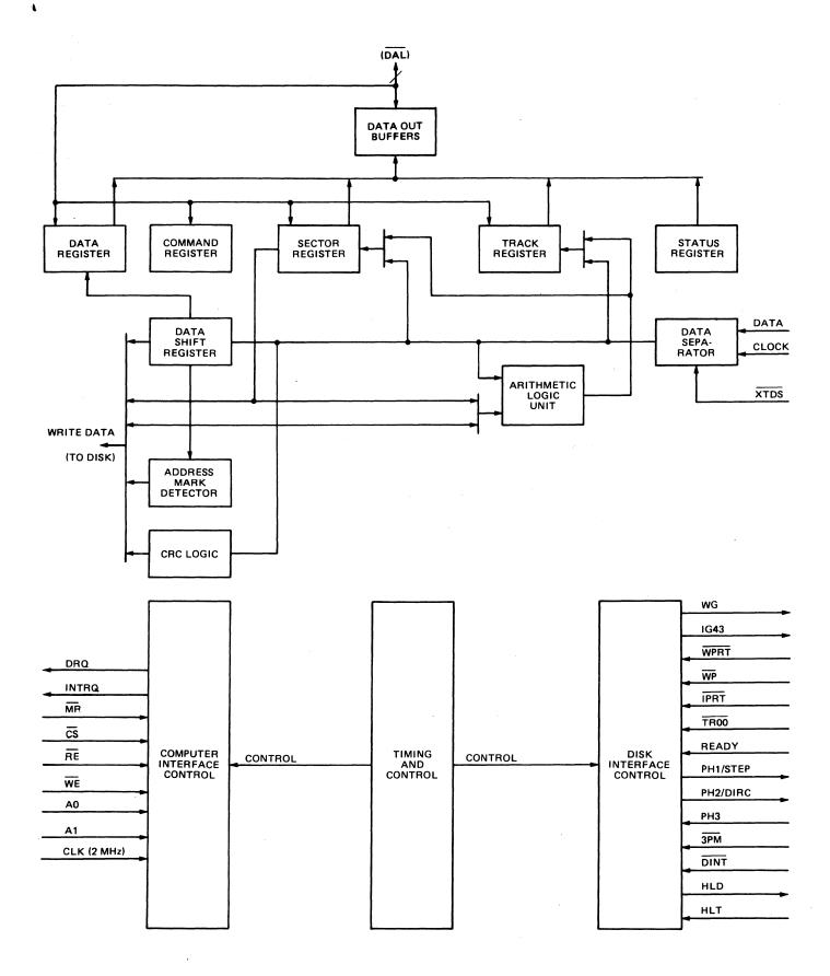
Figure 4-4. Floppy Disk Formatter/Controller Module Block Diagram
