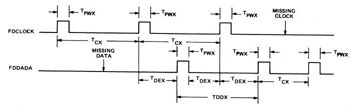
NOTE: 1. ABOVE TIMES ARE DOUBLED WHEN CLK = 1 MHZ. 2. CONTACT WDC FOR EXTERNAL CLOCK/DATA SEPARATOR CIRCUITS.
