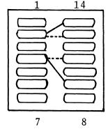
Figure 2-2. PERSCI Dual Disk Drive Wiring Modifications
