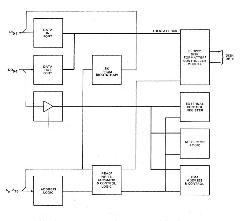
Figure 1-1. AM-200 Simplified Block Diagram
