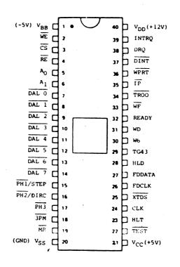
Figure 4-3. Floppy Disk Formatter/Controller Pin Connections
