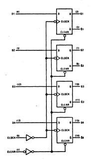
Figure 4-23. Quad D Flip-Flop Connections
