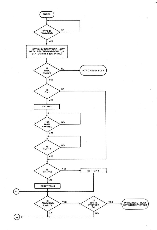
Figure 4-6. Type II Command Flow (Sh 1 of 4)
