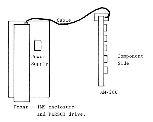
Figure 2-1. AM-200 Cabling to PERSCI Disk Drive
