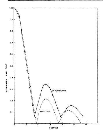
Figure 3—Directivity pattern for a surface wave radiator at 8 MHz with 0.23 inch width
