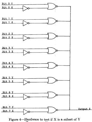
Figure 4—Hardware to test if X is a subset of Y  $Z = (\widetilde{Y}_0 \land X_0) \lor (\widetilde{Y}_1 \land X_1) \lor \ldots \lor (\widetilde{Y}_7 \land X_7)$
