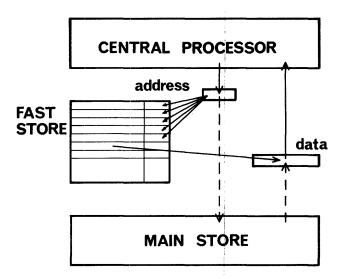
Figure 1—The use of an associative fast store to reduce the access time of the main store
