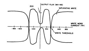
Figure 6-Output flux vs. write word current
