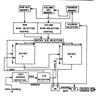
Figure 3-Digital route transposition matrix
