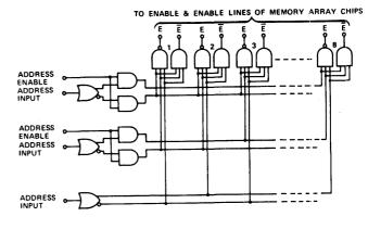
Figure 6-Chip select circuit logic
