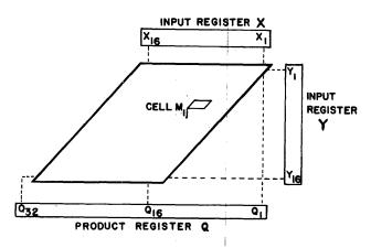
Figure 5--16  $\times$  16 bit functional multiplier
