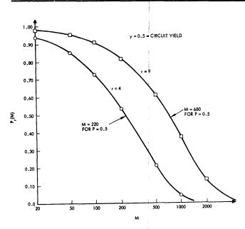
Figure 19—The probabilty P<sub>r</sub>(M) of successfully fulfilling a master pattern of M circuits by relocating from one of up to r nearby circuits. Each circuit is a tested unit which may have many gates of logic complexity
