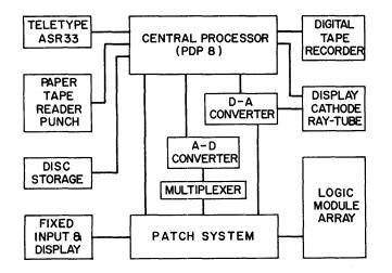
Figure 1-DADEC system - Block diagram
