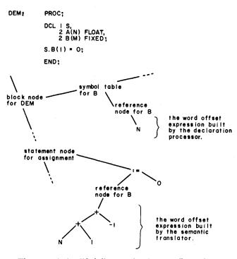
Figure 5—A simplified diagram showing the effects of subscripting
