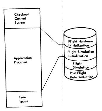
Figure 6--Phase load core memory map
