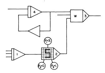
Figure 8—Use of storage element to store and transfer integrator output between simulations during iterative operation
