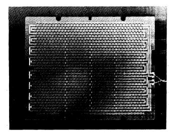
Figure 7-The mated film core array
