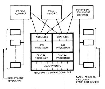
Figure 1-Typical multiprocessor application
