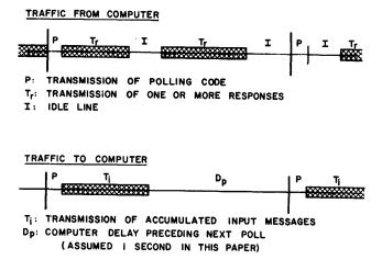
Figure 2B—Typical cycle of operation (Full-duplex message Transmission)
