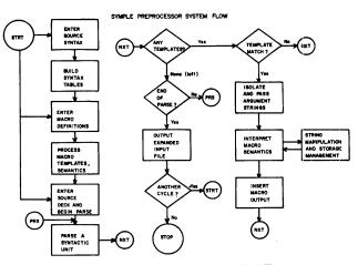
Figure 1—A general flow of the SYMPLE macro preprocessor system
