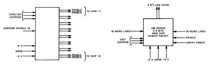
Figure 5—Chip select circuit
