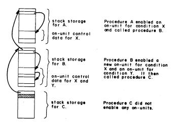
Figure 7—Stack storage and the signal mechanism A signal for condition X causes the signal mechanism to search tack through the stack until it finds the first enabled on-unit for condition X.
