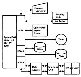
Figure 2—Flight software development laboratory— Block diagram
