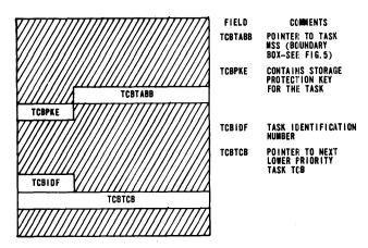
Figure 3—Task control block (TCB)
