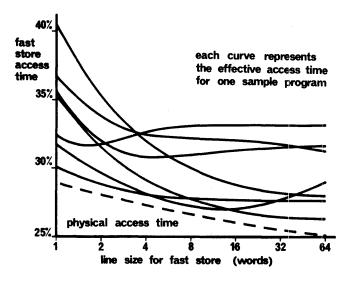
Figure 3—The physical access time of a fast store (broken line) and the effective access times (contnuouslines) for several sample programs. Access time is a percentage or main store access time line size is in words, and store size is 1024 words
