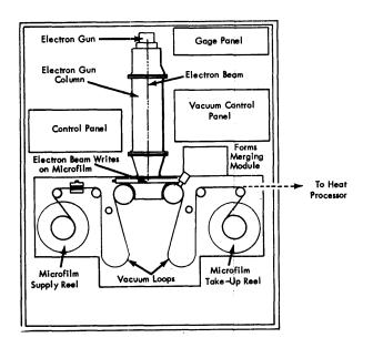
Figure 6-Electron beam recording on microfilm
