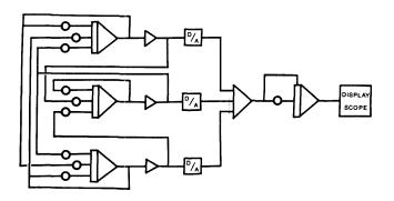
Figure 5-Linear PDE problem analog diagram
