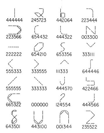
Figure 6—Segments used to print teletype symbols
