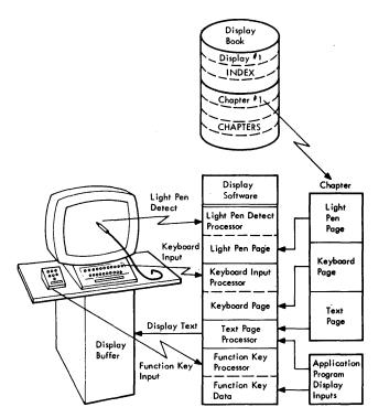
Figure 10—Display control interface
