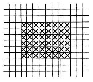
Figure 3—The 48 dot matrix defined by the intersection of one row and one column
