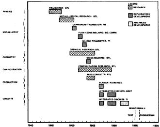
Figure 4—From transistor to Minuteman II, a twentyyear sequence of innovations in solid-state devices
