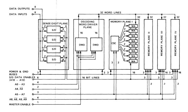
Figure 13-8192 bit memory stack-electrical organization
