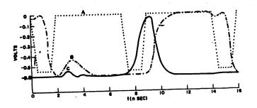
Figure 15-Waveforms of simulated flip-flop
