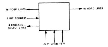
Figure 10-Decoding word driver package
