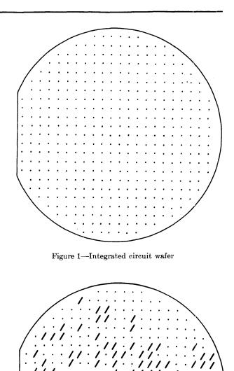
Figure 2—Wafer after test—Slashes show good circuit positions
