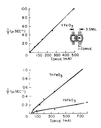
Figure 8—Functional velocity curves of YFe0<sub>3</sub>, TbFe0<sub>3</sub> and TmFe0<sub>3</sub> platelets.
