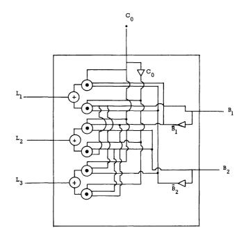
Figure 5b—Cell-K of the input control circuit
