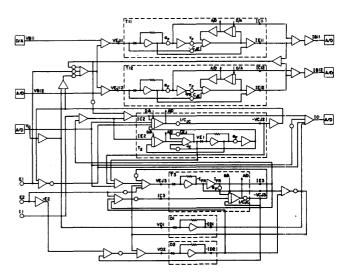
Figure 13—Analog computer simulation of a NOR gate
