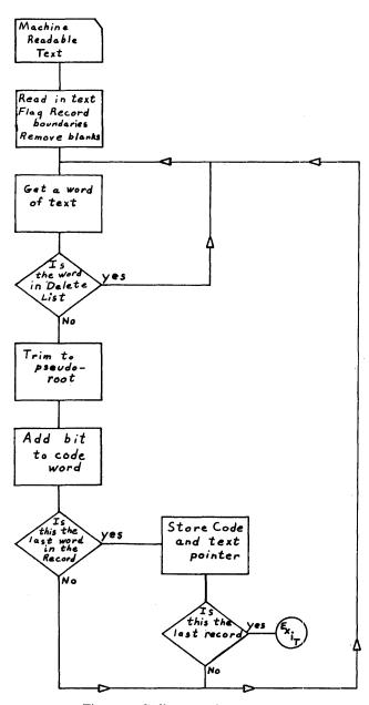
Figure 1-Coding procedure
