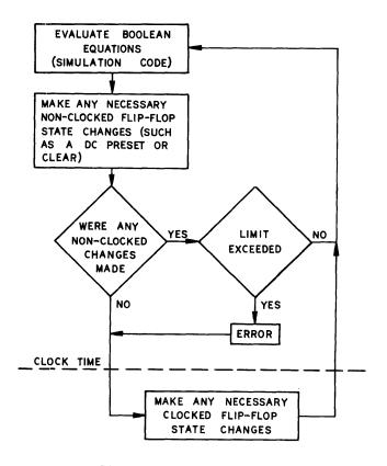
Figure 4-Simulator controller
