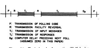
Figure 2A—Typical cycle of operation (Half-duplex message transmission)
