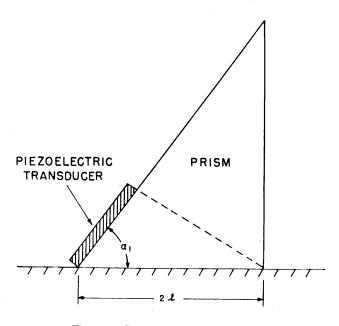
Figure 1-Surface wave radiator/sensor
