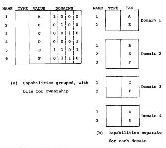
Figure 5-Capabilities and unprotected names
