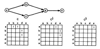
Figure 13-Examples of C<sup>n</sup> matrices
