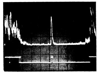
Figure 5—Echo receiver response Vertical: Upper 0.5 v/div., Lower 5.0 v/div. Horizontal: 25 µsec/div.
