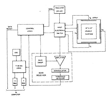
Figure 4-Position encoder block schematic
