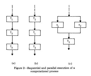
task  $T_3$  is independent of whether tasks  $T_1$  and  $T_2$  are executed sequentially as shown in Figure 2(a) or 2(b), then parallelism is said to exist between tasks  $T_1$  and  $T_2$ . They can, therefore, be executed in parallel as shown in Figure 2(c).
