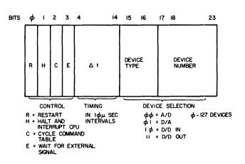
Figure 3-Hybrid processor commands
