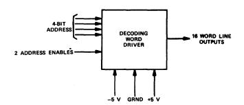
Figure 8-Decoding word driver chip
