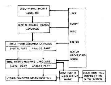
Figure 1-A hybrid computer programming system
