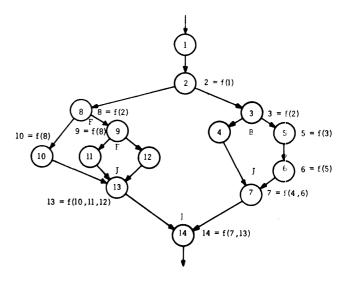
Figure 7—Final program graph of the parallel processable program
