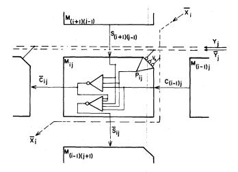
Figure 6-Functional multiplier cell
