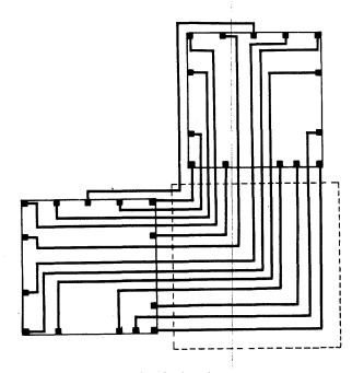
Figure 6—A set of pad relocations necessary to replace functionally the quad two-input gate circuit in area A of Figure 5
