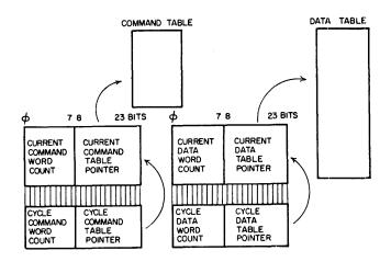
Figure 4—Command and data table structure
