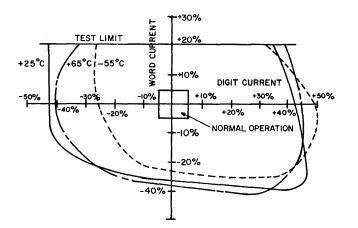
Figure 18-Memory system operating margins
