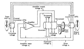
Figure 4—Schematic diagram of motor-generator instrument servomechanism
