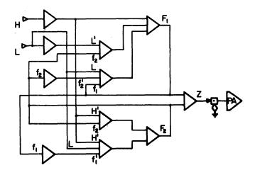
Figure 3-Pulse-height detector - Logic diagram
