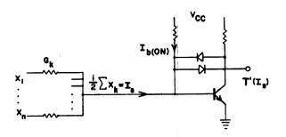
Figure 2—Threshold gate with Scnottky diode feedback
