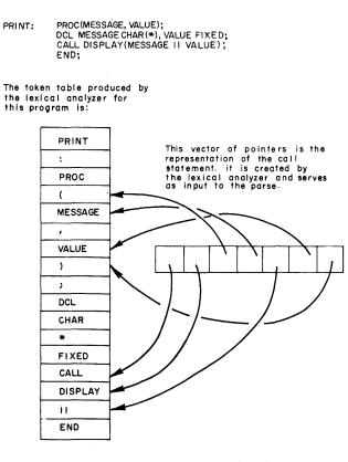
Figure 2—The output of the lexical analyzer.
