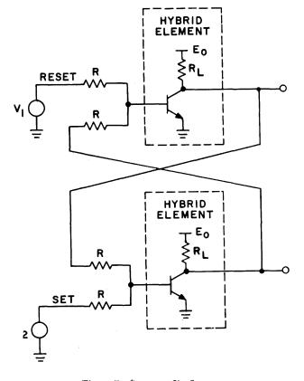
Figure 7-Set-reset flip-flop
