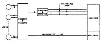
Figure 3—Asynchronous time division multiplexing system for time-sharing computer communications
