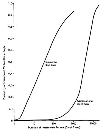
Figure 4-Sensitivity of multiply/divide logic
