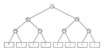
Figure 10—An alternate interconnecting scheme for the 8-modules of the  $64 \times 64$  multiplication unit
