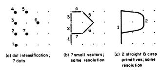
Figure 11—Comparison of straight/cusp and point intensified characters of same resolution
