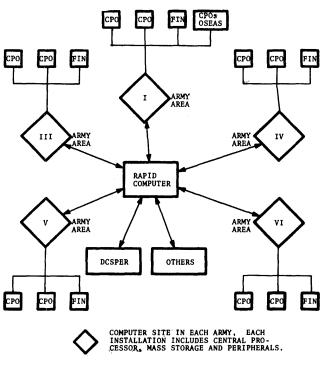
Figure 3-Six computer configuration
