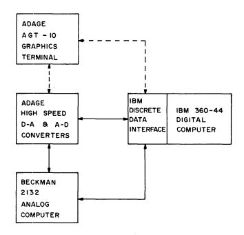
Figure 10—USC system simulation laboratory computer complement
