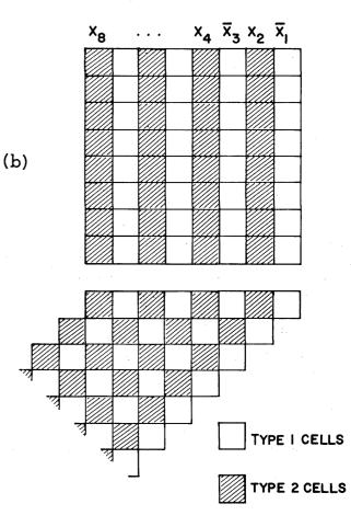
Figure 9b—Alternating columns  $X/\overline{X}$  composed of type 1/type 2 cells
