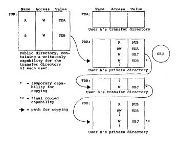
Figure 7—Sharing capabilities without access keys
