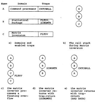
Figure 6—Traps and trapreturns
