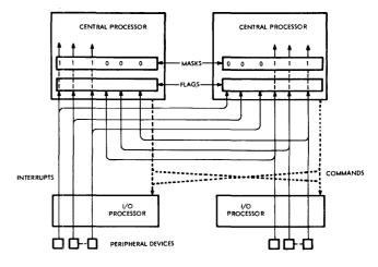
Figure 4—Input-output control block diagram
