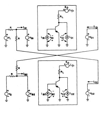
Figure 8-Set-reset flip-flop
