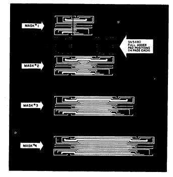
Figure 11---Four relocation patterns for SN5480's
