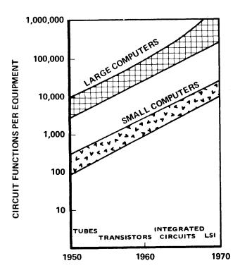
Figure 2-Functional complexity of electronic computers
