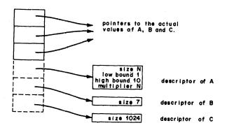
Figure 8—An argument list showing the relationship between arguments and their descriptors. The broken lines indicate that descriptors are optional. must be capable of bit addressing in order to implement unaligned strings. Since descriptors contain no addressing information, they are quite often constant and can be prepared at compile time.
