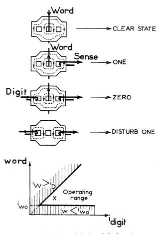
Figure 2—Operation of the three hole element
