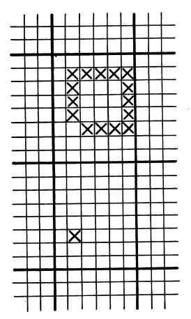
Figure 6—The pattern produced by the following coding <B%C%D%E%F%J%N%R%V>%B%F%J%K%L%MN The "<" defines subsequent characters as upper case. The ">" defines subsequent characters as lower case. The "%" is the code for the backspace function
