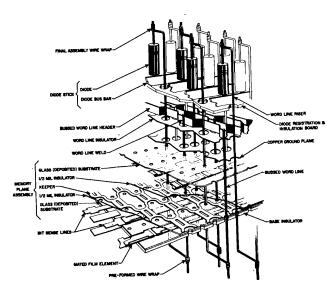
Figure 12-The substack
