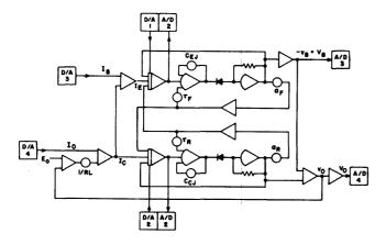
Figure 10-Analog simulation of a NOR gate
