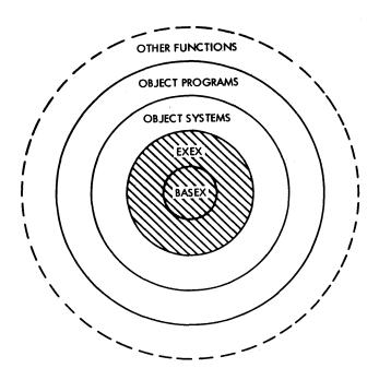
Figure 2—Multiple levels of control in ADEPT
