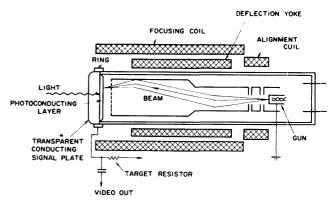
Figure 2--Schematic cross-section of the vidicon
