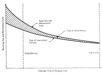
Figure 7-Cost of failures
