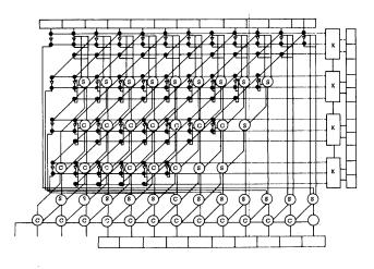
Figure 6—The binary multiplying cellular array
