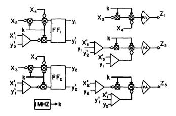
Figure 8-Shock measurement system - Logic diagram
