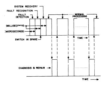
Figure 2-Fault recovery sequence (with spare)
