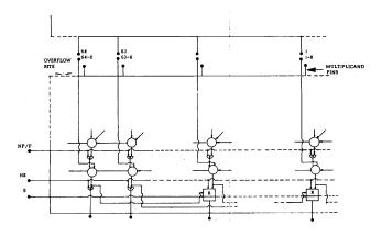
Figure 9—The combinational logic gating for reconfiguration
