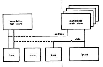
Figure 6—Typical hardware for a future large scale computer
