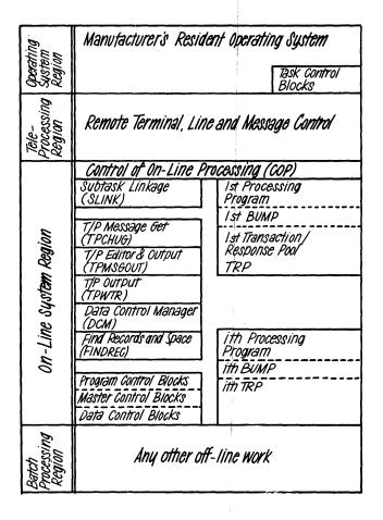
Figure 3-Main memory usage during on-line processing
