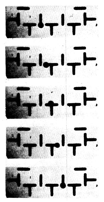
Figure 15—Sequence of photographs showing a 2 mil diameter domain propagating as the field rotates clockwise through 360°
