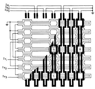
Figure 9—Thin film conductor pattern for two dimensional propagation of cylindrical domains. Conductor dimensions identical with that of Figure 6.
