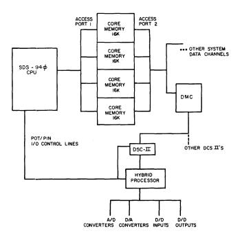
Figure 5-Connection of hybrid processor to SDS-940
