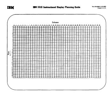
Figure 2—This shows the organization of the screen into 32 rows and 40 columns forming 1280 addressable units. The standard alphameric characters occupy two of these boxes, i.e., two rows by one column
