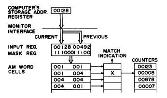
Figure 4—Recording occupancy and transitions of execution areas
