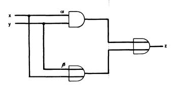
Figure 6-Example of a redundant circuit
