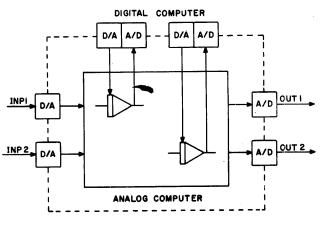
Figure 2-The hybrid element
