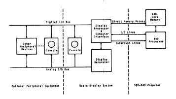
Figure 1—System configuration
