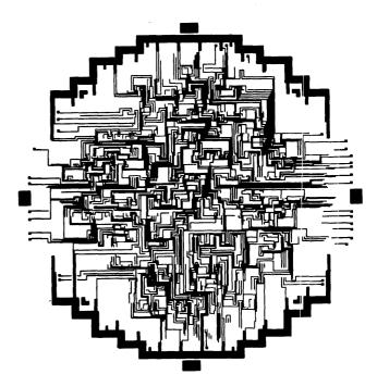
Figure 17—5-bit modular multiplier standard interconnect mask
