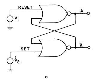
Figure 6a-Set-reset flip-flop
