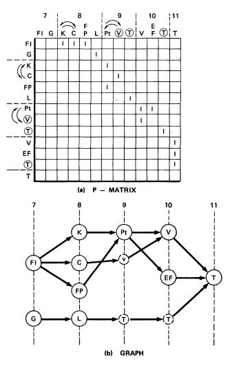
Figure 9-An example of improper "level" assignment
