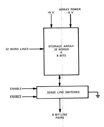
Figure 2—Block diagram MOS storage array
