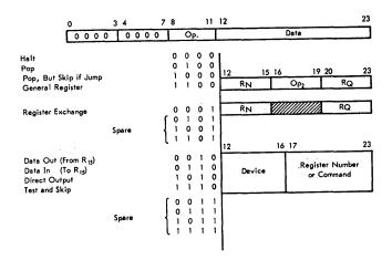
Figure 3d-Miscellaneous and I/O commands
