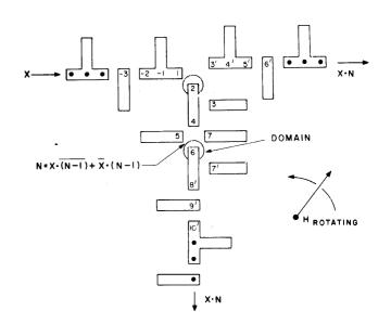
Figure 17—Cylindrical domain flip flop—The state of the flip flop is determined by the presence or absence of a trapped circulating domain at the sequencing pole positions; (idler) 4, 5, 6, 7. Each new domain entering the input channel x changes the state of the flip flop by becoming trapped in the idler if it is full
