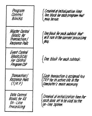
Figure 4---Control blocks for on-line processing
