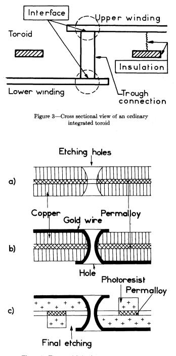
Figure 4—The new fabrication process: cross sectional view
