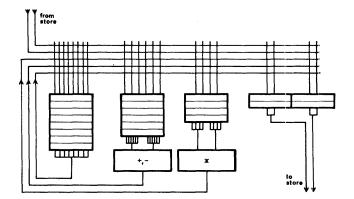
Figure 7—Detail of the floating point arithmetic unit
