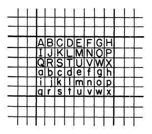
Figure 5—The characters used to define our graphic alphabet. The character plus its case determines the position of the dot within the matrix
