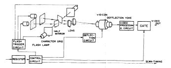
Figure 1-Schematic diagram of the character generator
