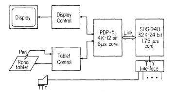
Figure 1-Hardware used in recognition research
