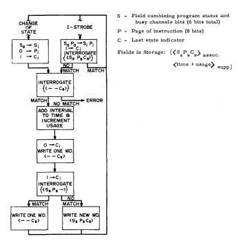
When an instruction strobe initiates a cycle, the monitored bits are routed through the A register to the I/E register for interrogation of associative memory. A match indicates no change of system state and completes the cycle.
