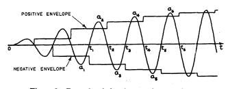
Figure 2—Data signal showing envelopes and zero crossings
