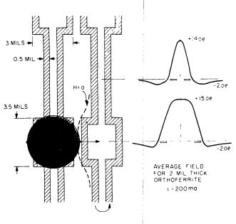
Figure 6—Conductor circuit used to propagate cylindrical domains and the resulting field profiles for 200 mA applied current
