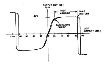
Figure 5-Output flux vs. digit current
