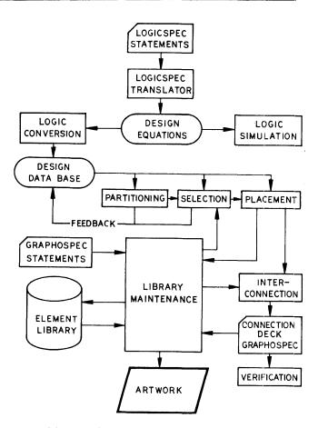
Figure 1-Computer-aided design system for CIS
