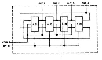
Figure 2—Four bit ring-counter
