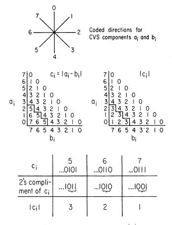
Figure 9—Algorithm for computing  $|c_i|$
