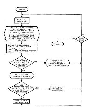
Figure 4—Static check control
