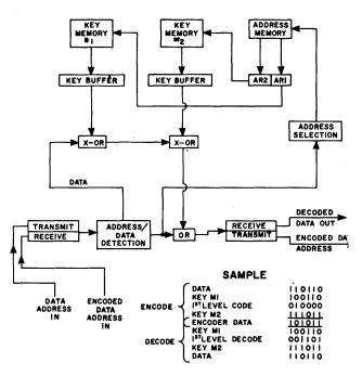
Figure 1—Digital substitution logic
