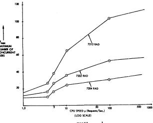
Figure 4—N<sub>max</sub> vs. CPU speed  $\mu$
