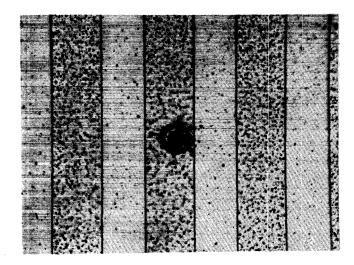
a-2. Enlargement showing self-healed pinhole
