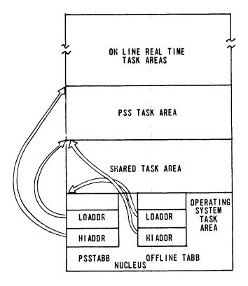
Figure 8—TABB pointers in PSS and offline task prior to modification
