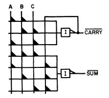
Figure 8-SLT full adder position
