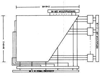
Figure 4-The modified "two bit" multiplier
