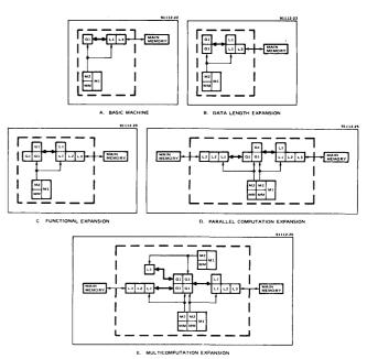
Figure 14-Four stages of expandability
