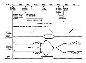
Figure 17-Timing for a typical memory cycle
