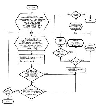
Figure 3-Potentiometer setting control
