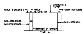
Figure 1—Fault recovery sequence (without spare)
