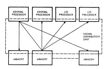
Figure 2-Fail-soft computer configuration
