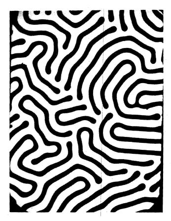
Figure 1—Strip domains, 1.5 mils in width, in a 1.7 mil thick platelet of Sm.55Tb.45FeO3 orthoferrite viewed by Faraday effect. Note the single wall domains. Bias field is zero
