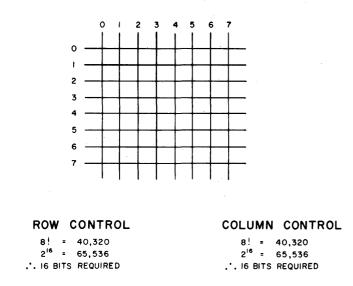
Figure 2-Digital route transposition matrix
