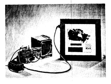
Figure 6-Touch sensitive position encoder
