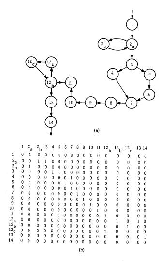
Figure 5—Program graph of a serially coded program and its connectivity matrix
