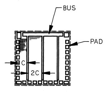
Figure 9-Typical chip layout
