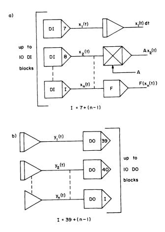
Figure 17-Disk input and disk output block configurations
