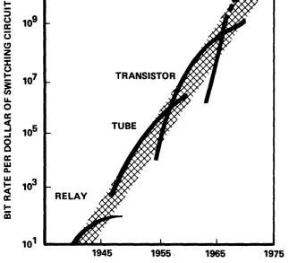
Figure 5-Switching rate per dollar for computer logic elements
