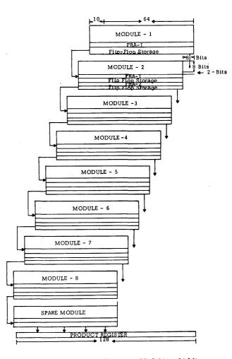
Figure 8—Example of an assembled  $64 \times 64$ -bit multiplication unit using the pipelining scheme
