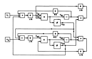
Figure 9-HYPAC block diagram for set-reset flip-flop
