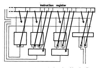
Figure 8-Control for the floating point arithmetic unit
