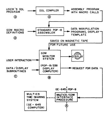
Figure 1-GDM subsystem interactions
