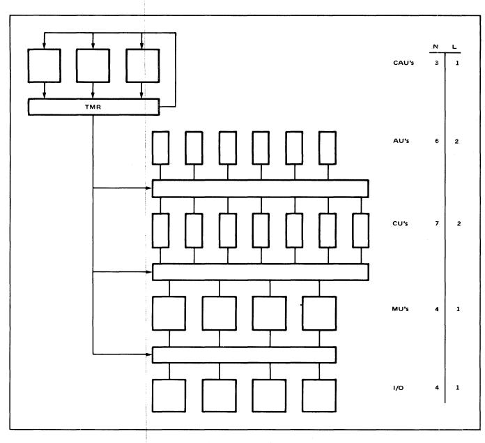
Figure 5-Multi-module modular computer
