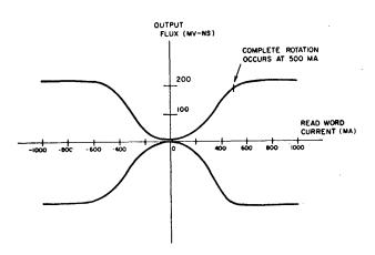
Figure 4-Output flux vs. read word current
