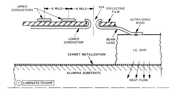
Figure 15-Interconnect cross-section
