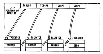
Figure 9—Portion of nucleus showing TCBLIST and TCBTCB pointer relationship prior to modification
