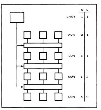
Figure 2-Three column modular computer
