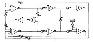
Figure 2—Simulation of an automobile suspension system
