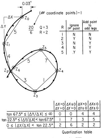
Figure 8-Algorithm for computing CVS
