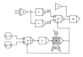
Figure 9—Storage element used to modify structure of simulation from one solution to next
