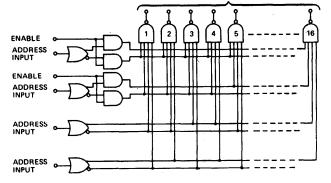
Figure 9-Decoding word driver chip logic
