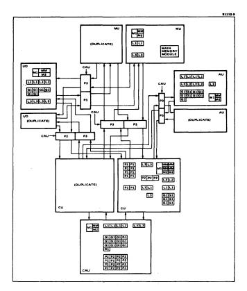
Figure 17—MCB-Modular computer breadboard block diagram
