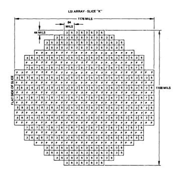
Figure 13-LSI array slice "K"
