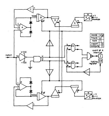
Figure 4-The envelope detection circuit
