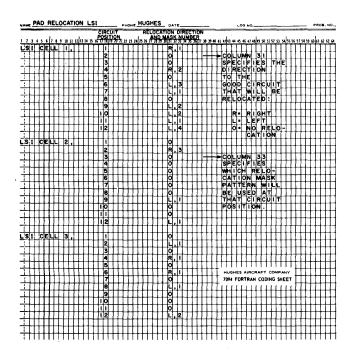
Figure 10-Coding sheet specification
