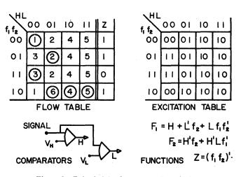
Figure 2-Pulse-height detector - Description
