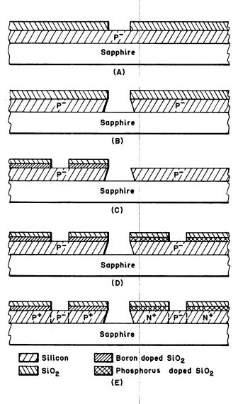
Figure 5-Low temperature CMOS Process
