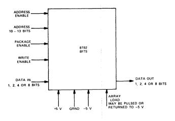
Figure 1-Block diagram 8192 bit module
