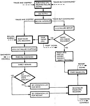
Figure 7— Central processor error: Surviving CPU
