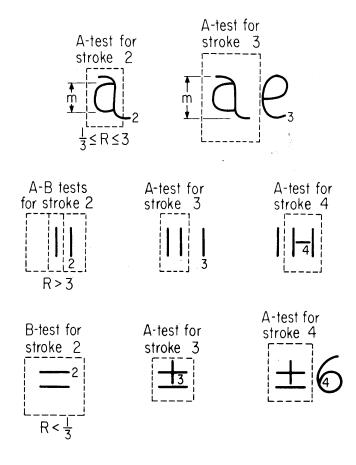
Figure 11-Symbol completion algorithm examples
