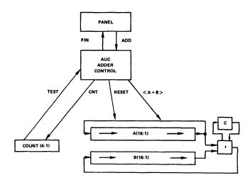
Figure 3-Serial adder
