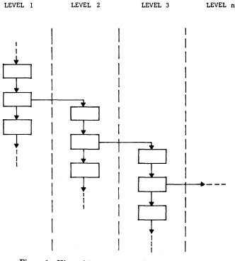
Figure 1—Hierarchical representation of a sequentially organized program
