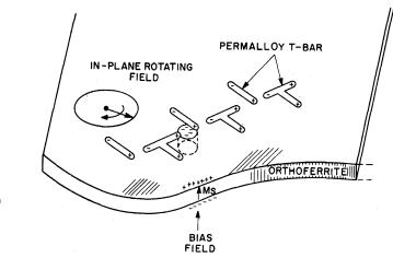
Figure 14—Isometric view of permalloy T-BAR pattern in contact with surface of orthoferrite platelet. Rotating in-plane field generates poles which cause the domain to move
