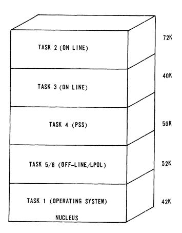
Figure 11-Initial task core allocations
