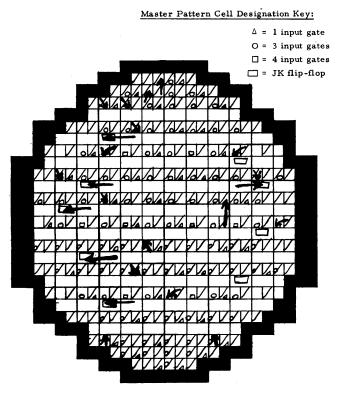
Figure 14—Pad Relocation worksheet with master pattern locations shown
