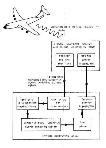
Figure 1—The data reduction system
