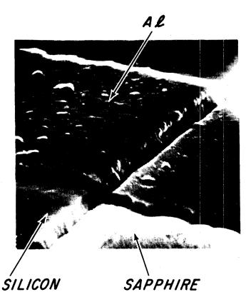
Figure 7—Aluminum metallization over oxidized silicon edge
