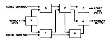
Figure 3b—Partially ordered functional modules of a processor
