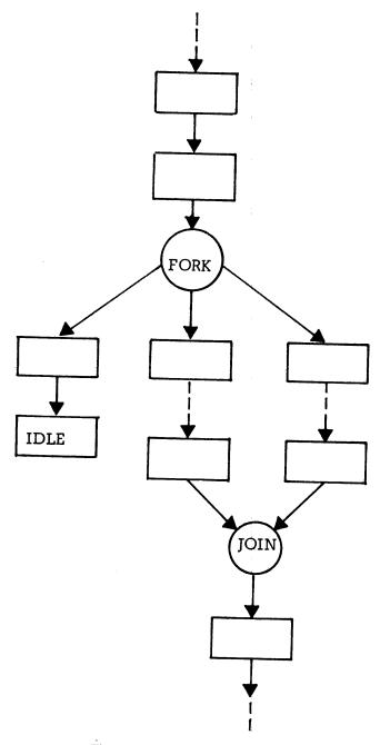
Figure 4-FORK and JOIN technique
