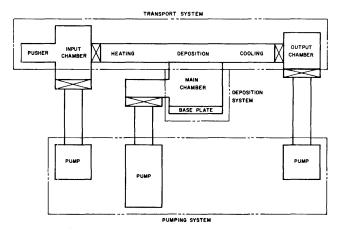
Figure 10-Continuous vacuum evaporator
