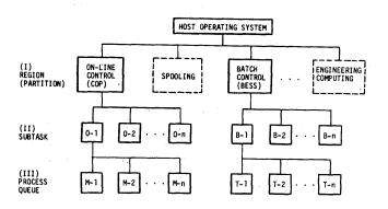
Figure 1—Hierarchical control on three levels of multiprogramming
