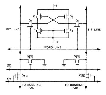
Figure 3-Storage cell circuit schematic
