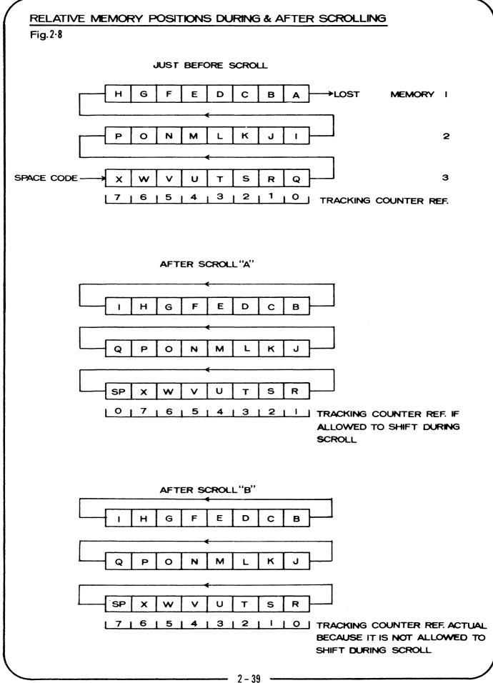
line where they should be. The same is true of memories #1 and #2. In order to correct this situation, the Tracking Counter must be allowed to go out of sync for the 80 shifts. This is done by not allowing it to count during the time the memories scroll. This reassigns the lines such that the spaces are in line 7. The bottom of Figure 2.8 shows the actual relationship between the data and the Tracking Counter. Note the Tracking Counter hasn't changed from the top reference.
