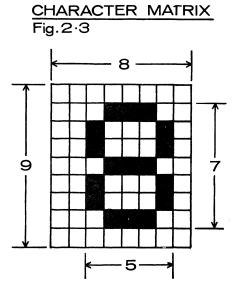
To generate a character on the screen the Read Only Memory, ROM, must supply seven five-bit words to the video shift register, one for each of the seven scan lines used to display the character. During each scan line at the given character position the video shift register shifts the five bits to the video mixer at the 12.528 MHZ rate. These bits make the video black for ones and white for zeroes, assuming a normal black on white presentation.
