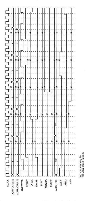
Figure 9-17. Target Arbitration Reselection
