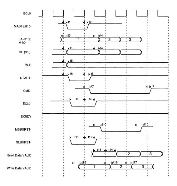
Figure 9-7. EISA Burst Transfer - 32-bit Burst
