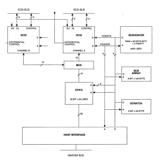
Figure 1-1. Block Diagram
