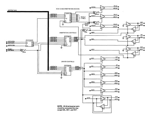
**Figure 4-1. Differential Controls**
