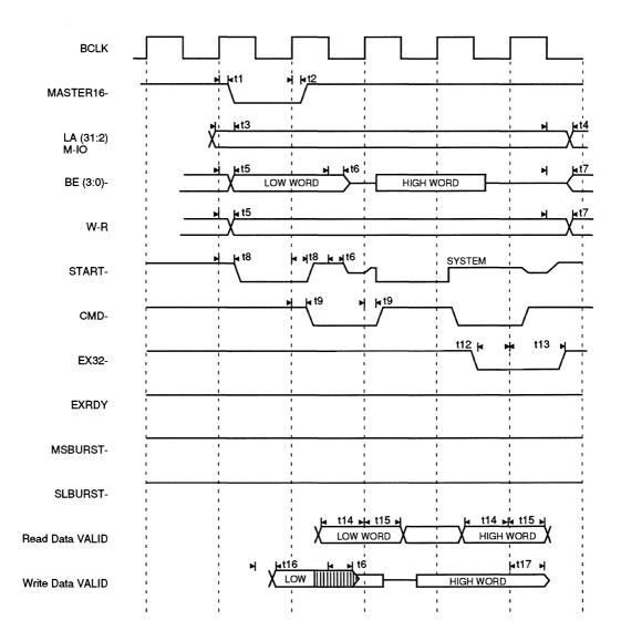
Figure 9-10. EISA Two Cycle Transfer-16-bit Translate
