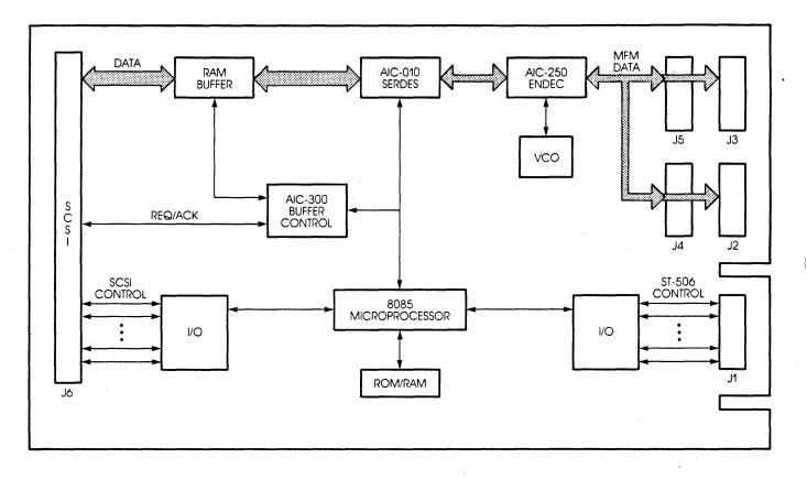
Figure 2-1. ACB-5500 Block Diagram
