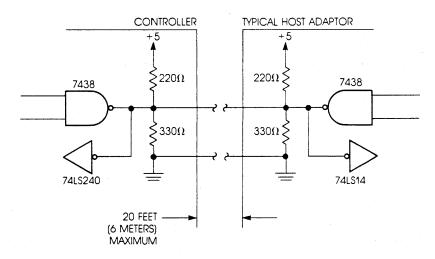
Figure 4-1. Host Adapter Bus Termination
