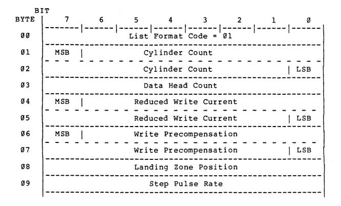
Figure 6-25. Drive Parameter List for Soft-Sectored, Fixed Drives
