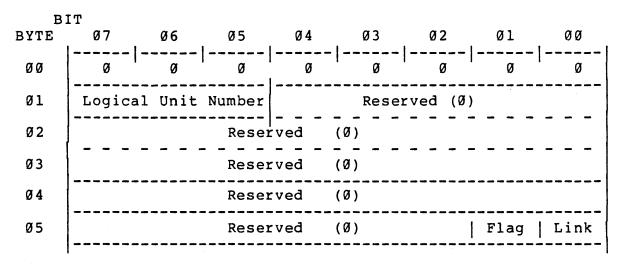
Figure 6-1. TEST UNIT READY Command
