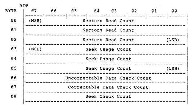
Figure 6-18. READ/RESET USAGE COUNTER Parameters
