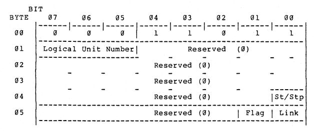
Figure 6-31. START/STOP UNIT Command
