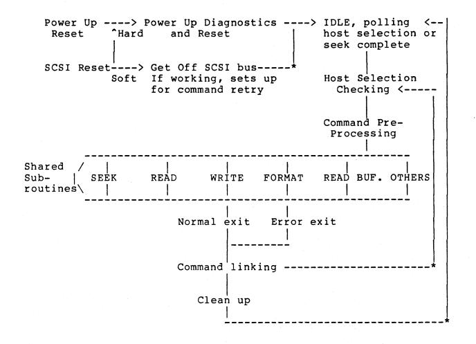
Figure 2-2. ACB-5500 Microcode Structure
