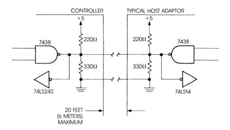
FIGURE 4-1. HOST ADAPTER BUS TERMINATION
