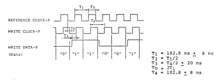
FIGURE A-1. WRITE DATA AND CLOCK TIMING
