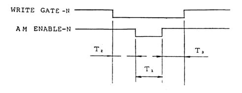
$T_1 = 24$  Bit times  $T_2 = T_3 = 100$ ns min
