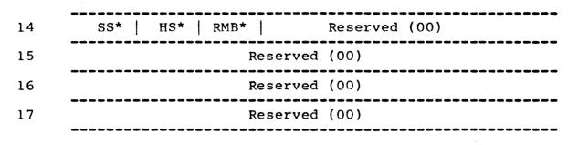
\* - Parameters not changeable by MODE SELECT; field must be set to zero
