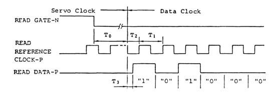
$T_{0} = 4 \text{ bytes}$   $T_{1} = 102.8 \text{ ns} \pm 10 \text{ ns}$   $T_{1}^{2} = T_{1} \pm 10 \text{ ns}$  $T_{3}^{2} = 0^{1} \pm 15 \text{ ns}$
