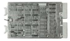
The CACHE/434 and CACHE/440 products increase the speed of DEC PDP-11/34 and PDP-11/40 computers without using additional back-plane space ( the unit installs in place of the M9202 Unibus jumper in PDP-11/34 systems or the M981 Unibus jumper in PDP-11/40 systems). In addition to speed, CACHE offers 4K words of temporary memory.
