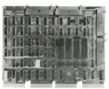
Each Able QUADRASYNC board is designed to replace four of the DEC DL11-B, DL11-C or DL11-E boards, offering significant space and power saving. Each Able QUADRASYNC is capable of sending and receiving data simultaneously, and they save dc bus loading. Jumpers are eliminated by the switch selectable data format, addressing and vector feature. QUADRASYNC/B is EIA only, QUADRASYNC/C is current loop only, and QUADRASYNC/E is EIA only but with modem control.
