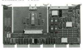
Able's EASYWAY Ethernet Port offers DEC PDP-11 and VAX-11 users high performance Unibus to Ethernet network data transfer. High performance is achieved by off-loading the host CPU, made possible by locating on the board the bottom four layers of the International Standards Organization Open System Interconnect (ISO, OSI). EASYWAY also features drivers within RSX11M/S and VAX/VMS, providing the capability for DMA operations to and from the board.
