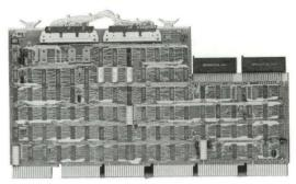
The INTERLINK/UNI is a hex width board, INTERLINK/LSI is a quad width board, and BUSLINKS are combinations of two INTERLINK boards.
