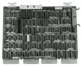
The VMZ/LP is a microprocessor based DMA line printer controller for DEC's VAX-11 series computers which contains a single parallel channel to emulate the line printer function of DEC's DMF/32 controller.
