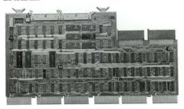
ENABLE makes it possible to extend the address space of DEC PDP-11 systems from 256K bytes to 4 megabytes. It allows all currently existing programs to remain memory resident and so substantially increases system throughput.
