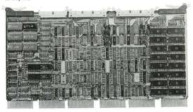
This DZ11-E look-alike and act-alike Able product supports 16 communication lines with modem, yet it uses only half the power and space of the DZ11. Hex width, it has dip switches to set vector and address. The upper 8 lines of the Able DZ/16 can be turned off, allowing easy trouble shooting, and it also features programmable line parameters, DEC diagnostic and operating system software compatibility, and on-board self diagnostic with LED display.
