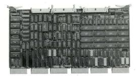
Able DH/DM is the preferred replacement for the DH11 and DM11 in virtually all of Digital Equipment Corporation's PDP-11 family of computers (except -11/04 and LSI). Like other Able products, this microprogrammed 16 line hex board with modem control offers space saving, and it requires only half the power and one third the bus loading of the DH11. It doubles the processing speed because it provides word, rather than byte (half word) data transfer.
