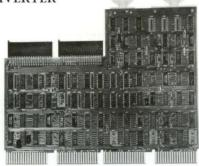
The Able QNIVERTER is the first bidirectional Unibus/Q-Bus bus signal converter. With this quad board in a DEC LSI-11 computer, older PDP-11 peripheral equipment can be used on the LSI. With the QNIVERTER in a PDP-11, newer LSI peripherals can be used. Application possibilities for this product are nearly limitless.
