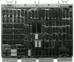
Able's Q/DH, another first, offers the user the option of operating 8 or 16 communication lines on a DEC LSI-11 computer. Programmable operating parameters provide a variety of features such as modem control (standard on all lines), EIA or EIA/20 mA current loop distribution panels, and flexibility to upgrade to 22 bit DMA addressing.
