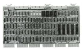
Sophisticated end users appreciate the flexibility offered by the DV/16, which provides an interface between a DEC PDP-11 computer and up to 16 communications lines. The lines can be synchronous or asynchronous, and are switch selectable in four line increments. Complete word, rather than byte, transfer improves data throughput capability. The DV/16 replaces the DEC DV11.
