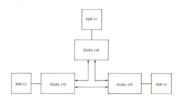
DUAL I/O As Three-Processor Programmed Link
