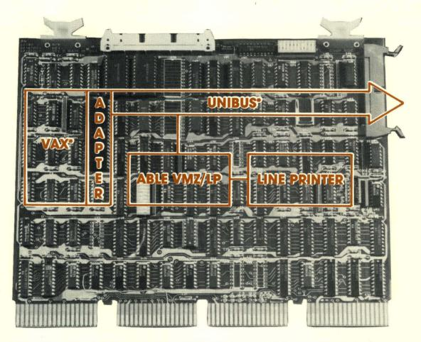
**The VMZ/LP LINEPRINTER CONTROLLER** is a microprocessor based lineprinter controller which contains a single parallel channel programmed to emulate the lineprinter function of a Digital DMF32 controller. The channel contains the hand shaking signals necessary for lineprinter operations.
