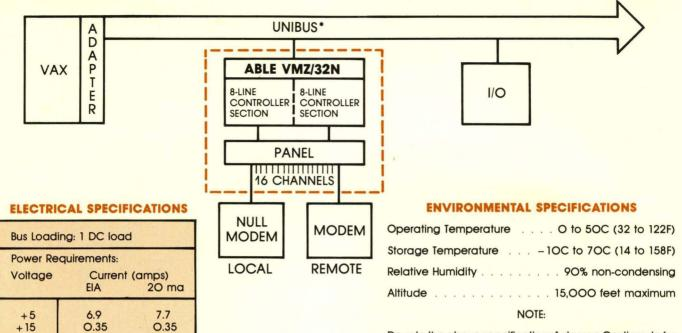
De-rate the above specifications 1 degree Centigrade for each 1000 feet of altitude above 8000 feet.
