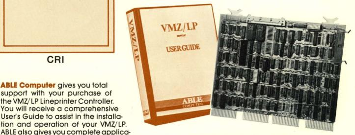
tion engineering support should you have any special applications in mind. Your VMZ/LP is shipped to you with an optional 220/330 ohm resistor pack, so you can contour your VMZ/LP to accommodate many of the popular brands of printers in the marketplace. We also assist you with rapid board replacement and repair at our factory. You will find that ABLE's quality is unsurpassed.
