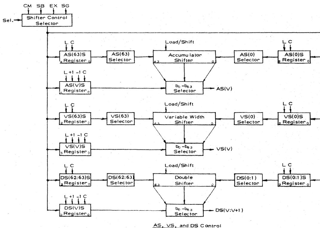
The SG which is associated with this selector is called the Common Shifter SG. Various shifter control data can be stored in this SG for various shifter interconnections and then used in environment prologues. The microoperations associated with the CS SG are shown in Table 2.15.
