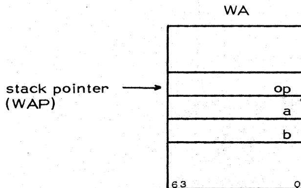
We wish to take two operands, *a* and *b*, and an arithmetical or logical operator, *op*, from the stack and place *a op b* on the new top of stack. The following microinstruction sequence does this.
