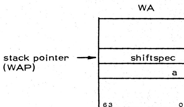
We wish to treat the AS as a left shifter whose characteristics are given by *shiftspec*. We wish to shift *a* *n*-times and return the result to the new top of stack after removing *shiftspec* and *a*. Let us assume *shiftspec* to have the following format:
