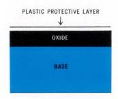
The Sandwich is constructed as shown in the diagram above. The famous "Scotch" Brand high potency oxide coating is sandwiched between a tough polyester base and a 50 micro-inch protective layer of plastic. Since the oxide is never in contact with the head, tape movement is smooth and low in friction—easy on both tape and equipment. Oxide can't rub off and distort valuable data.
