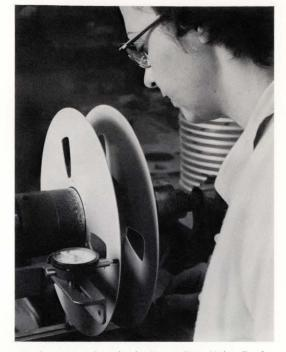
Production worker checks Heavy Duty Video Reel for lateral runout. This check is performed on each reel.
