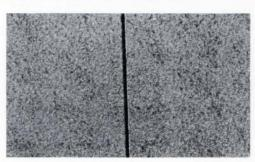
Keep in mind that a finite separation (though extremely small) exists between the tapes being spliced. Note above photomicrograph. The low viscous solvents normally used (naptha, alcohol, Freon TF\*) can seep through the separation to deteriorate the adhesive.
