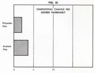
Temperature Coefficient of Linear Expansion x 10<sup>-5</sup> per degree Fahrenheit
