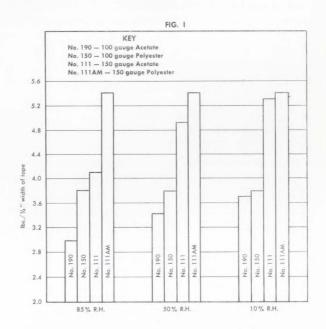
Here one can readily see that the higher humidity has a softening, or plasticizing, effect on the acetate backing, but has negligible effect on the polyester tape backing. This plasticizing effect also shows up in the relative tear strength of the acetate which accounts for the apparent brittleness of acetate at low humidities.
