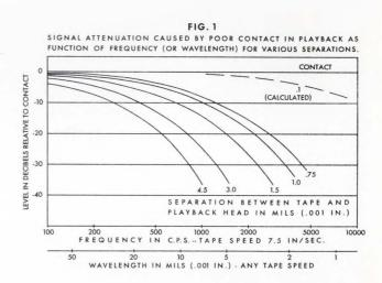
These curves show the attenuation caused by various separations of tape and playback head. On the frequency scale the data are plotted as for a tape speed of 7.5 in./sec., but it should
