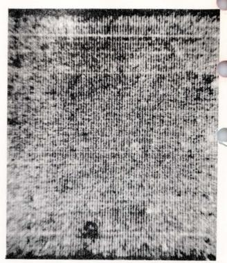
This photo-micrograph illustrates the fine definition obtainable with an oil suspension. The wavelength is .002 in. so that the lines are .001 in. apart. Lamination defects may
