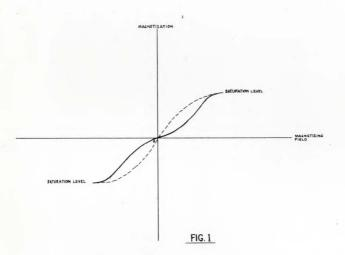
field (such as produced by a recording signal) is not directly proportional to the original signal. This characteristic, if not corrected would result in very bad distortion of
