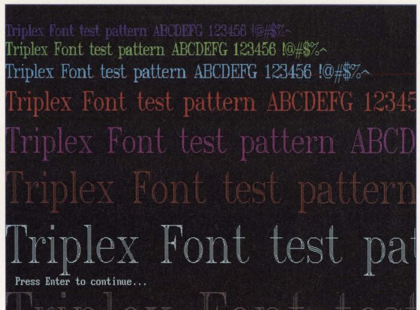
Figure 8. A BGI stroked font in increasing sizes. Stroked fonts often improve in appearance as they are enlarged. Note the clipping of drawn characters at the bottom edge of the screen.
