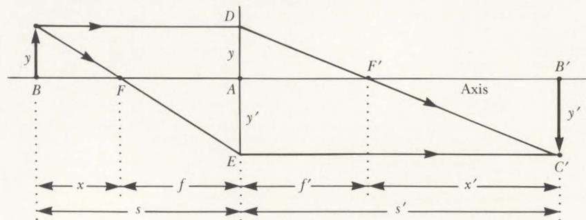
to the image of height  $y'$ . Let  $s$  represent the object distance from the center of the lens and let  $s'$  represent the image distance from the center of the lens.  $x$  represents the object distance from the focal point  $F$ , and  $x'$  represents the image distance from focal point  $F'$ .
