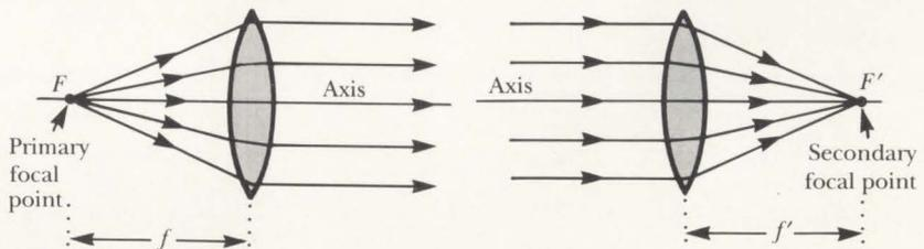
Figure 1. Two views of a thin lens with rays from and to  $F$  and  $F'$ , respectively.
