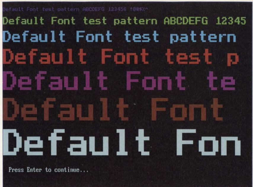
Figure 7. A BGI bit-mapped font in increasing sizes. Note how aliasing (the stairstep effect on diagonal character segments) becomes more objectionable as the characters are enlarged.
