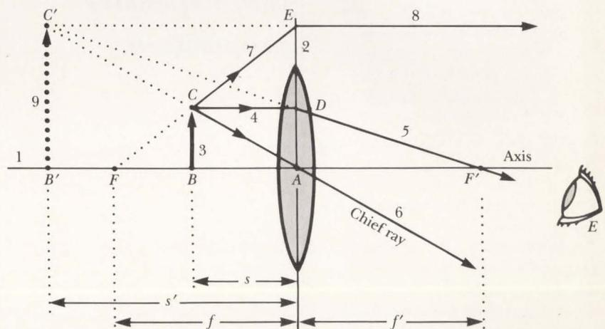
Figure 3. Placement of an object between the focal point and the lens, creating a virtual image.
