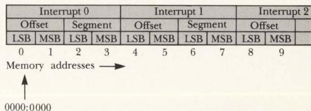
Figure 1. The structure of the 8088 interrupt vector table. There are 256 vectors in the table, each consisting of 4 bytes that represent the service routine segment and offset in the order shown.
