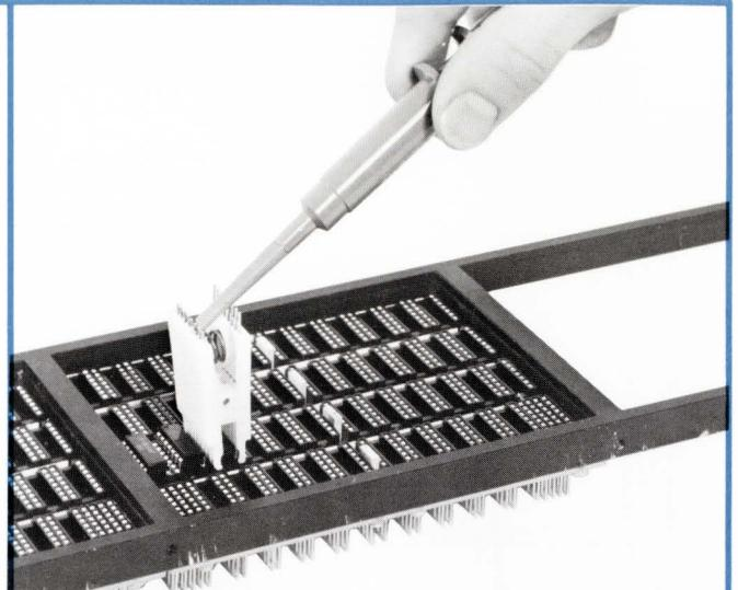
**H-2705 Test Clip and Insertion/Extraction Tool for IC's**
