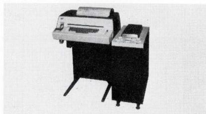
**Station arrangement** includes Teletype 38 wide platen ASR terminal and Model 4210 magnetic tape data terminal.
