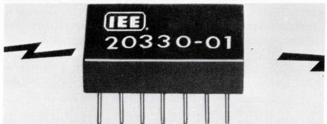
This hybrid "Hex Buffer" drives 6 150mA or 3 300mA incandescent lamps. Inputs TTL/DTL compatible and 5V logic supply. With pull-up resistor, can be used in clock and line driver applications with high fan-out. One-999 20330s, \$5.45; 4-6 weeks ARO. Tom O'Gorman, IEE, 7720-40 Lomona, Van Nuys, Ca. 91405 (213) 787-0311
