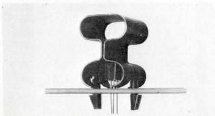
Three sizes of snap-in heat sinks cool and mechanically support plastic transistors on 1/16 to 3/32 in. thick cards. Types 293-3 and -2 may be used with two transistors side-by-side when common collectors are permitted. Wakefield Engineering, Inc., Audubon Rd., Wakefield, Mass. 01880.
