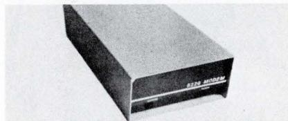
The 5220 is a low-cost, compact, originate or answer-only modem. It includes power supply and indicating lights for power and carrier detect when supplied. The unit is compatible with the Bell 101, 103, and 113 Series. It will operate full-duplex at speeds up to 300 b/s, is strappable for half-duplex and will interface with Bell couplers. RFL Industries, Inc., Boonton, N.J. 07005.
