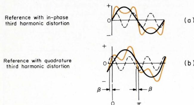
**Third-harmonic distortion of the reference.** In (a), with in-phase third harmonic, there is no shift in the zero-crossover points. With a quadrature third-harmonic (b), there is an effective phase shift of  $\beta$  whose magnitude (in radians) is given by  $\beta \approx$  third harmonic  $\div$  fundamental. A similar condition exists for higher order odd harmonics.
