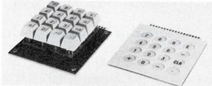
Because of its unique mechanism, you can get these keyboards in standard configurations or with extremely low profiles. The switch itself uses a gold plated elastic diaphragm to contact a gold plated pad on a printed circuit card. Datanetics Corp., 18065 Euclid St., Fountain Valley, Calif. 92708.
