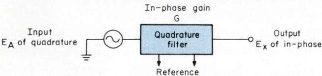
The in-phase component of the output resulting from a quadrature input is an error voltage. A quadrature input,  $E_A$ , causes an in-phase output,  $E_x$ . The equivalent in-phase input error is  $E_x/G$ , where  $G$  is the in-phase gain. The  $QRR_i$  (quadrature to in-phase rejection ratio) is  $\frac{E_A}{E_x/G}$ . In this case,  $QRR_i$  is defined as
