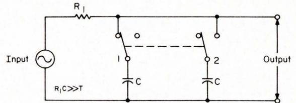
A basic quadrature filter is made up of RC networks and time-controlled switches.
