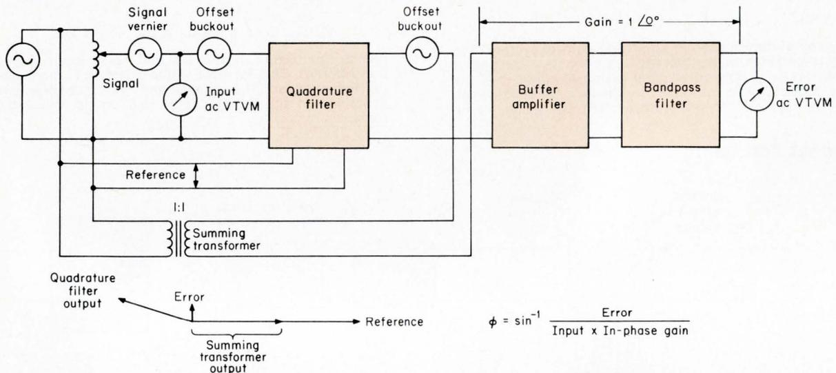
**Measuring the phase shift.** The signal control should be a low-phase-shift variable transformer. It can be a low-resistance potentiometer if no phase shift is introduced by the load on its arm. The signal vernier is the same type of in-phase generator as the in-phase offset buckout generator. The summing transformer should have low phase-shift and low series-leakage inductance and resistance. The signal controls are adjusted for a null on the error ac VTVM. The sum-
