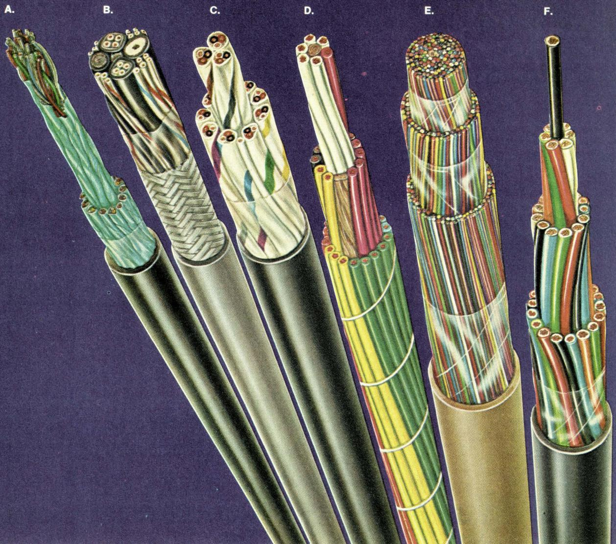
**A. RECORDING STUDIO:** Audio sound cable: 25 shielded pairs, stranded copper conductors, low loss insulation, twisted with uninsulated drain wire, isolated aluminum tape shields, cabled, PVC jacket.
