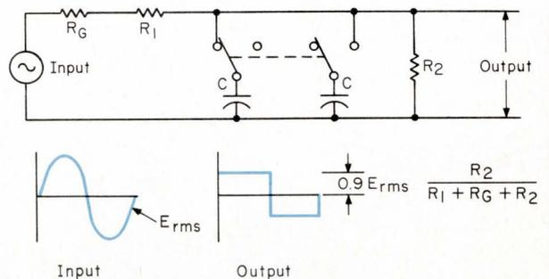
A quadrature filter modified by additional input and output resistors is shown above. This modification reduces the output voltage by the factor given in the output waveform.
