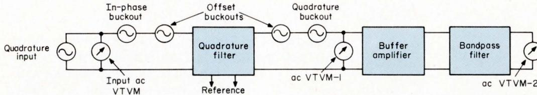
**Setup for making quadrature-rejection tests.** The offset buckouts remain set as before. The in-phase buckout is used to determine the in-phase output resulting from a quadrature input. It is placed in the input circuit so that its phase is not critical. The in-phase and quadrature buckout controls are adjusted for a null on ac VTVM—2. The noise output is then read on ac VTVM—1. The in-phase output is equal to the
