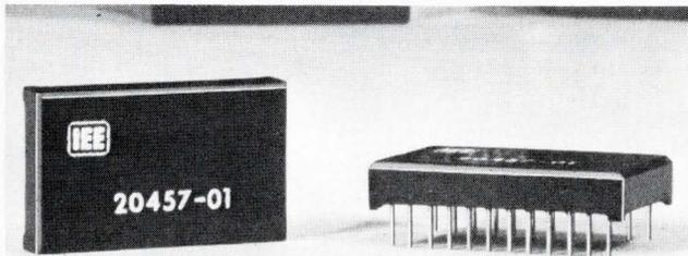
The 20457 Series of hybrid circuits decodes standard 8421 BCD data into 12 outputs. Or, if only 10 outputs are needed, two may be used as lamp buffers. Intended primarily, as display drivers, the circuits have a drive capability of 300 mA at 30 V. The circuits are DTL/TTL compatible and you can get them with or without memory. Industrial Electronic Engineers, Inc., 7720-40 Leona Ave., Van Nuys, Calif. 91405.
