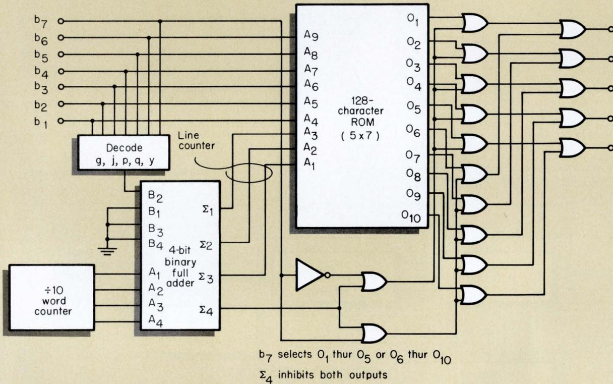
Some character fonts require the use of descender characters such as g, j, p, q and y. A larger matrix can provide two extra bottom lines for these characters, or you can use a circuit such as this one. The descender characters are detected and an adder subtracts a
