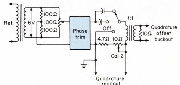
is also kept to a minimum, the secondary voltage is induced by inductive rather than capacitive coupling between primary and secondary. This provides an accurate primary readout of the isolated secondary. The resistances of the range resistors depend upon the voltage ranges and the output-transformer winding resistances.
