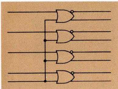
**MC10101 Strobed Quad OR/NOR Gate** — Very useful for distributing 4 bits of parallel information on or off card. With both OR/NOR outputs available, 4 twisted pair lines may be driven at data rates of 100 megabits/second. Use the single strobe input to gate the data on or off in 2 ns.
