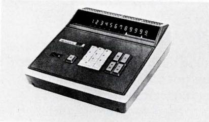
Models 1201 and 1201C offer mixed sequential calculations, constant multiplication, constant division, square and power calculations. Each is equipped with floating decimals and shut-off clearing. Models 1203 and 1603 also have grand totals and extra storage, a fixed and floating decimal point, and round-off. Sperry Rand Corp., Remington Rand Div., Box 999, Blue Bell, Pa. 19422.
