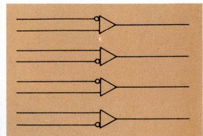
**MC10115 Quad Line Receiver** — Useful for receiving 4 bits of differential data transmitted over twisted pair or ribbon cable from the MC10101. Also recommended for MOS to MECL interfacing and is ideal as a sense amplifier equivalent for MOS 1103 type memory translation to MECL.
