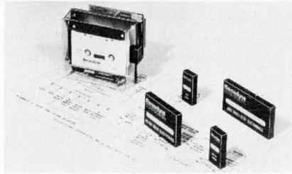
Philips cassette and achieves a packing density of 120 b/in for a total of 432,000 bits (or 43,000 characters) on one cassette. Character error rate is less than 1 in  $10^7$ .
