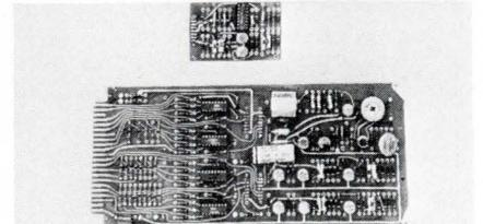
each telephone push-button digit, into a corresponding level output on 12 or 16 lines. You can select BCD or some other output coding, and the unit can provide unique digit format decoding to perform a variety of control functions. Quindar Electronics, Inc., 60 Fadem Road, Springfield, N.J. 07081.
