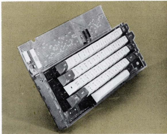
**This solid-state keyboard** from Micro Switch combines MOS memory with n-key rollover technology. It provides an electronic shift lock, three operating modes, a lighted shift lock key, full 128 character set and ASCII coding.
