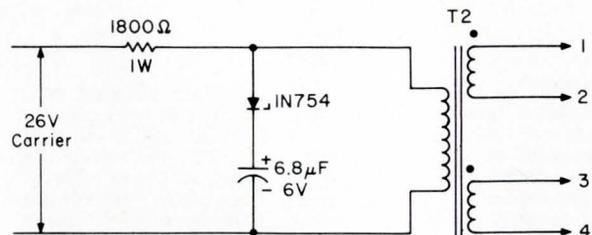
zener-capacitor clipper, and transformer T2 provide a clipped sine wave for the chopper excitation. The capacitor does not permit any dc to saturate the transformer or to be fed back into the supply. Transformer T<sub>1</sub> is a 2:1 stepdown (end to end) while T<sub>2</sub> is a 1:1:1. Both must have 10-H minimum primary inductance. All values in the circuit are based on a 400-Hz carrier.
