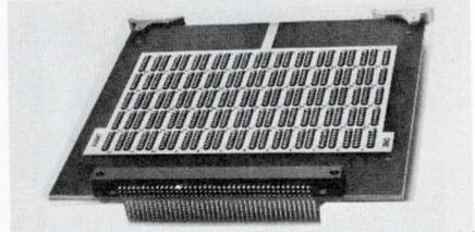
New standard panel is for 60 or 72 DIPS, 14 or 16 lead. Series 8136-W panels come with male connectors (120 contacts, 3 rows of 40 with 0.100 in. spacing between pins and rows). Mating female connectors are available. Panel is 1/8 in. glass epoxy with electro-tin plated VCC and Gnd. planes. About 7.350 x 6.950 in. Augat Inc., 33 Perry Ave., Attleboro, Mass. 02703.
