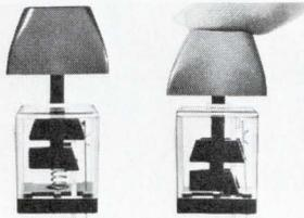
Contacts in this key are made of WE Alloy #1 (69% Gold, 25% Silver and 6% Platinum). Result is low contact resistance (typ. 25 mΩ). Also, contacts are normally held apart, eliminating bounce or microphonics. Cherry Electrical Products Corp., 3600 Sunset Ave., Waukegan, Ill. 60085.
