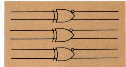
**MC10107 Triple 2-input Exclusive OR/Exclusive NOR Gate** — A three gate array providing the positive logic Exclusive OR and Exclusive NOR functions for high speed applications. Temperature compensated internal bias on 10,000 series devices insures that the threshold point remains in the center of the transition region over temperature.
