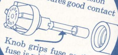
Knob grips fuse so that fuse is withdrawn when knob is removed
