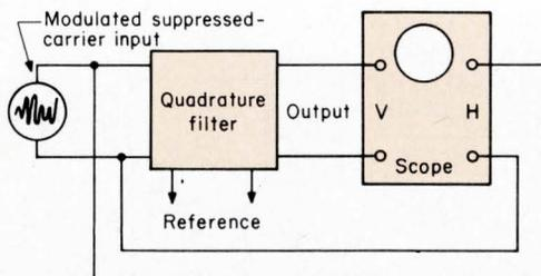
**Bandwidth is measured using this setup.** A Lissajous pattern of the modulation appears on the oscilloscope. The carrier also appears on the oscilloscope but can be disregarded. Since the quadrature filter appears as an RC network to the modulation, the 3-dB bandwidth is at the modulating frequency where the phase angle of the Lissajous pattern is  $45^\circ$ .
