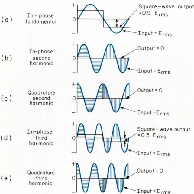
Signal harmonics in the input affect the output of a quadrature filter. The in-phase fundamental is shown in (a) as a reference. Since the quadrature filter is a waveform averaging device, it is not susceptible to even-order harmonics as shown in (b) and (c). In-phase odd harmonics produce a fundamental in-phase output seen in (d) and (e). Note that in the above figures the cross-hatched areas cancel.
