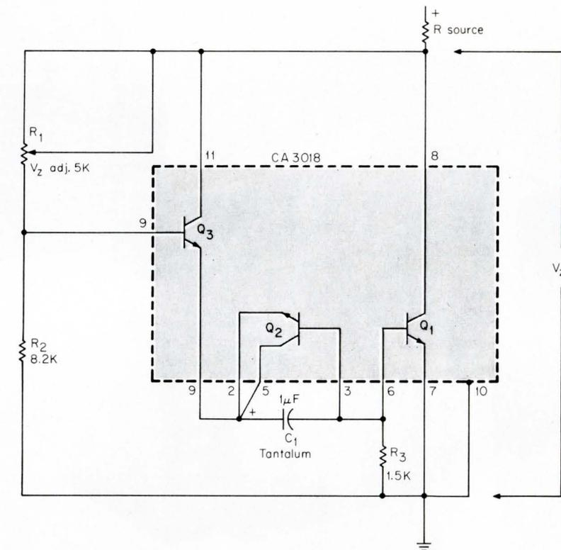
can be established by  $R_2$ . Thus  $R_1$  can program the terminal voltage across the IC, allowing regulation at any voltage from 8.4 V up to the maximum rating of the IC.
