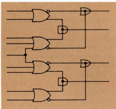
**MC10117 Dual 2-Wide OR-AND/OR-AND-INVERT Gate** — A powerful logic function featuring the first available OR-AND/OR-AND-INVERT emitter coupled logic gate. The internal collector AND/emitter OR dotted logic gate will perform the OR-AND/OR-AND-INVERT logic function in 2.4 ns. Useful for data multiplexing and data distribution.
