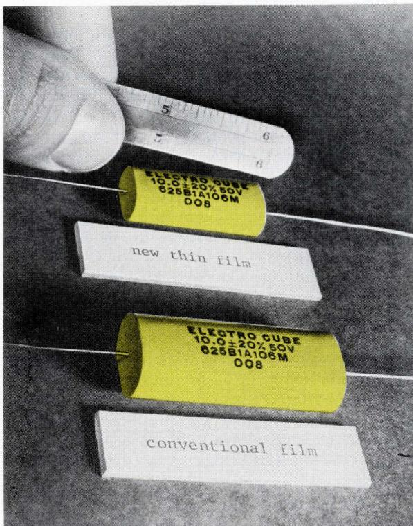
**A metallized film capacitor** can be from 20 to 50% smaller than a similar unit rolled with conventional film and metal foil. In addition, the metallized unit heals itself after a short burns a portion of the electrode. However, metallized film capacitors have higher dissipation factor and lower insulation resistance, and cost more than conventional film units. (Photo courtesy of Electro Cube, compares metallized polycarbonate unit, above, with one rolled with film and metal foil.)
