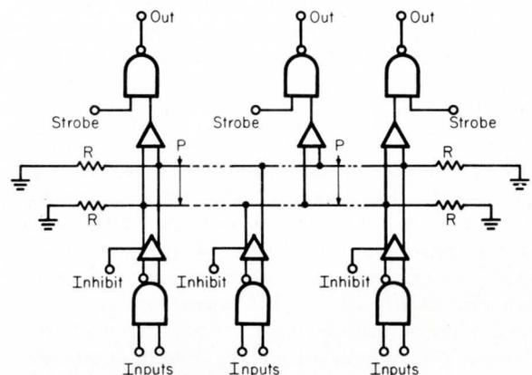
**This party line system** is made possible by the strobe provision on the receivers and the inhibit feature of the drivers. Any driver may communicate with any or all receivers in such a system.
