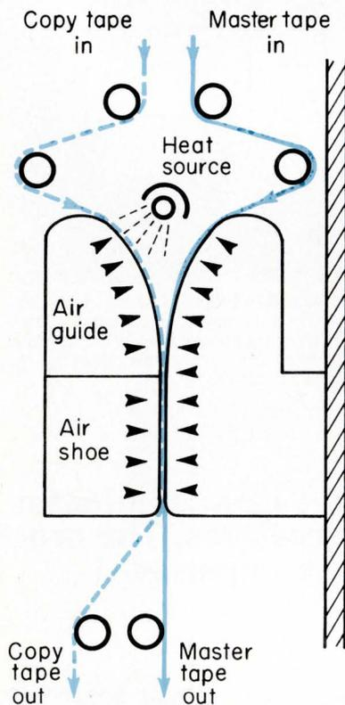
Video tape recordings can be reproduced rapidly using Du Pont's heat process.
