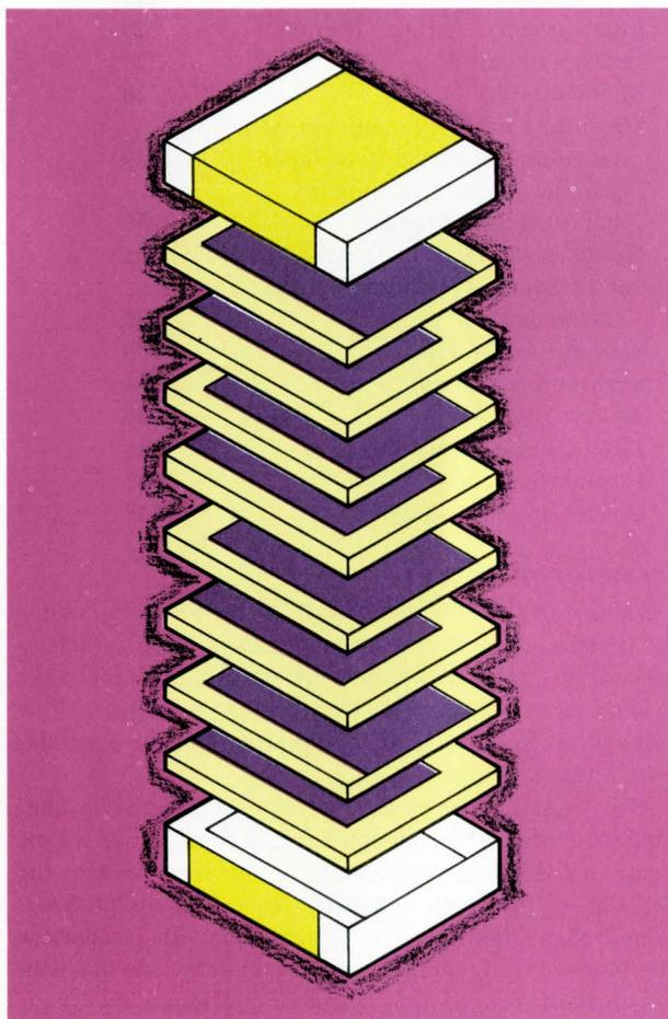
Construction of monolithic chip capacitor (Sketch courtesy of Monolithic Dielectrics, Inc.)
