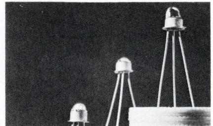
Type QS-507 is for general purpose computer and industrial applications that require light sensitivities 10 to 20 times those of normal photo transistors. It provides light current of 5.0 mA with irradiance of only 2.0 mW/cm<sup>2</sup>. Is sensitive to both visible and near I-R illumination. 45c (1,000 quan.). Quantum Sensing, Inc., 1650 Locust Ave., Bohemia, N.Y. 11716.
