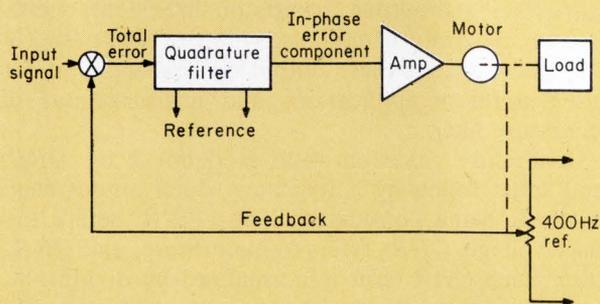
A typical ac position servo system shows the implementation of a quadrature filter. The error derived
