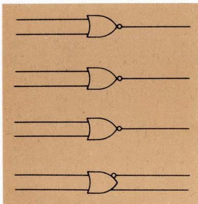
**MC10102 Quad 2-Input NOR Gate** — Offers four 2-input NOR gating functions with an additional OR output available. Input pulldown resistors on all devices eliminate need to tie unused inputs to an external supply.
