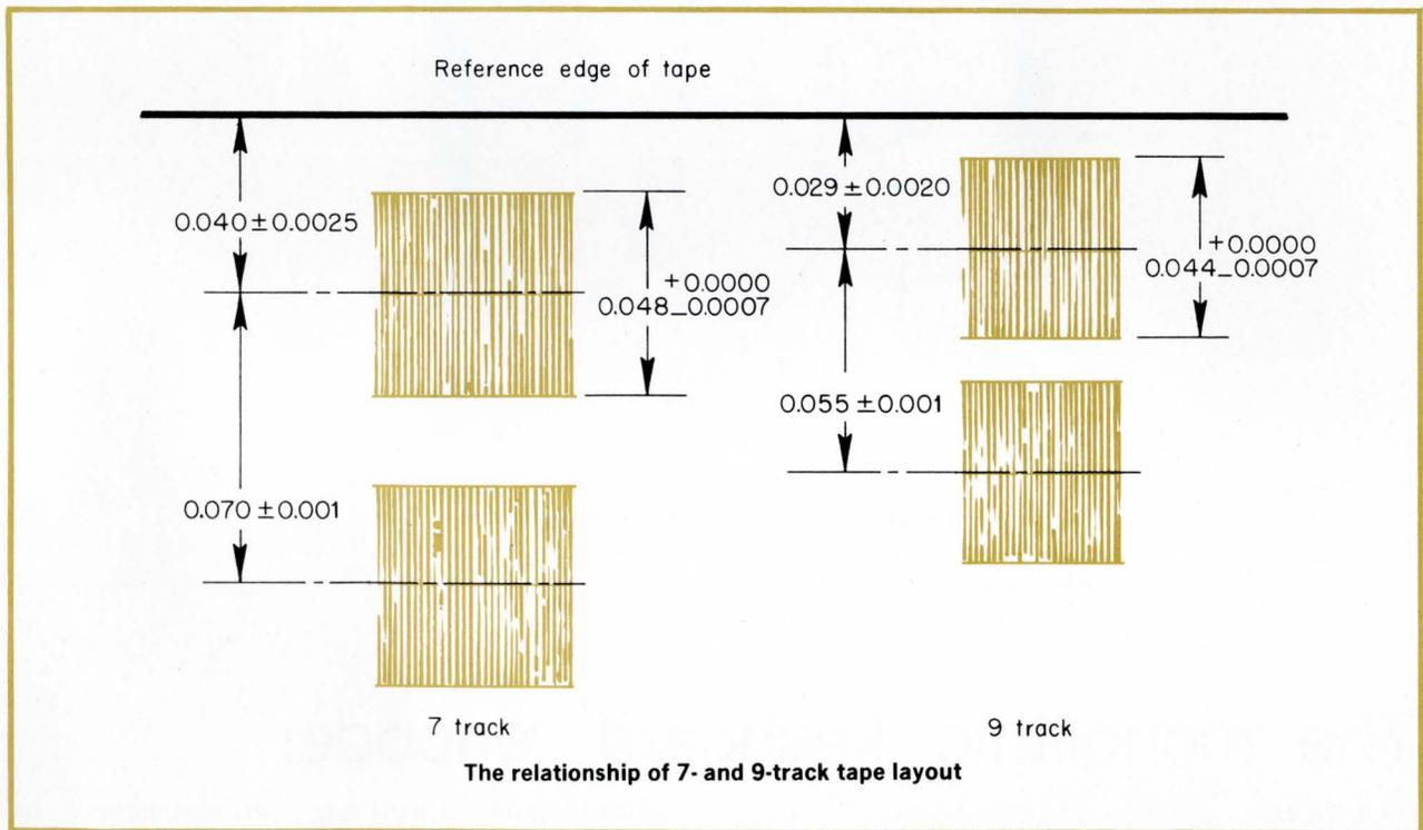
ment on Unrecorded Magnetic Tape for Information Interchange and GSA W-T-0051B, are guidelines that will be applied to new developments both in tape and equipment.
