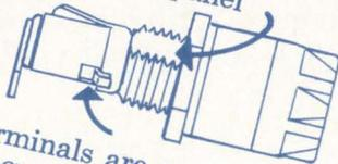
Terminals are mechanically secured in holder as well as soldered
