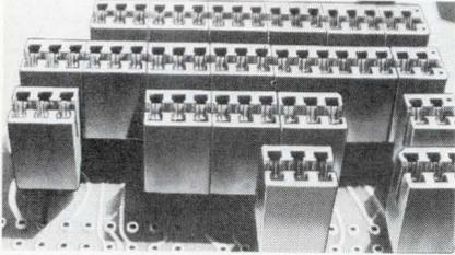
Series 6318 modular card edge connector provides a means to update connection systems without having to redesign existing PC cards with their 0.156 in. center contact traces. It comes in modules of four and six contacts. Elco Corp., Maryland Rd. at Computer Ave., Willow Grove, Pa. 19090.
