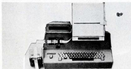
The Electro/Set 450 Editor is designed for speed and economy in making corrections and then producing a clean tape for high speed computerized equipment. The unit includes a floating display which offers 128 different symbols. Fairchild Graphic Equipment Division, 221 Fairchild Ave., Plainview, N.Y. 11803.
