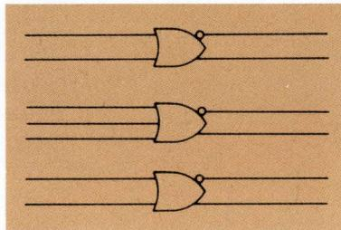
**MC10105 Triple 2-3-2 OR/NOR Gate** — A system oriented device aimed at reducing package count by providing three OR/NOR gates within one package. This versatile logic element provides manipulation of Boolean functions in typically 2 ns.
