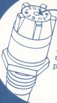
Knob has break-out hole to allow use of test probe
