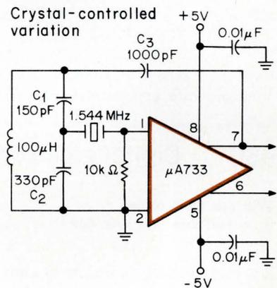
frequency in two ways, both of which give rise to the voltage-control variant of the basic circuit. In one method, you shunt an FET across  $R_1$ , and vary the FET's drain resistance by its gate voltage. Take care that you still satisfy the division ratio restrictions for the combination of  $R_1$ ,  $R_2$ , and the FET.
