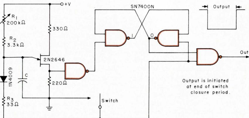
first gate which, in turn, SETS the flip-flop with a negative signal. The output is again HIGH.
