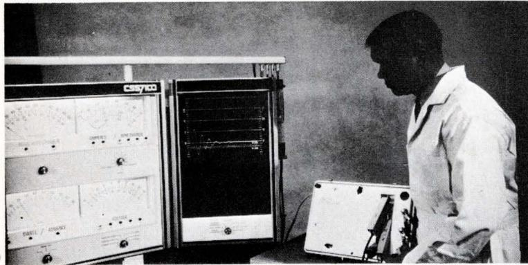
**Clayton's dynamometer** includes electronic instrumentation amplifiers for the panel meters. The electronic circuitry is packaged in rugged modules to withstand the service shop environment and to simplify service.
