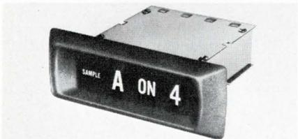
Series 0400 display features 0.50 in. message, viewable at 10 ft.; 60 fL brightness using 6 V lamps; front panel access; 0.752 in. center-to-center spacing, and a total weight of only 3 oz. Input is straight decimal (1 lamp/input terminal); or BCD with IEE driver/decoder. Industrial Electronic Engineers, Inc., 7720-40 Lemona Ave., Van Nuys, Calif. 91405. (213) 787-0311.
