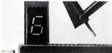
Because of its unique construction, the Data-Lit 3 can be plugged into a PC board edge card connector for a vertical display. Since it requires only 1.7 V/segment you can power the display from the same supply as the logic card. \$9.85 ea. (1000 quan.). Litronix, 10440 N. Tantau Ave., Cupertino, Calif. 95014. (415) 329-0810.
