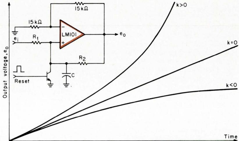
ous powers by adjusting the ratio of  $R_1$  to  $R_2$ .
