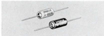
Unmatched for reliability at 125C by any other metallized paper capacitor. Higher insulation resistance than that of any other metallized paper design. Unique dielectric combines metallized paper and polyester film impregnated with special high temperature mineral wax. Hermetically sealed.
