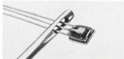
"HT-series" "Micro Sensor" consists of either a photo transistor or a photo-darlington sensor bonded to a ceramic substrate with three leads attached (emitter, base, and collector). HT-700 series offers low cost and fast switching speeds; HT-800 series has high gain and high sensitivity. The HT-700 is \$1.51 and the HT-800 is \$1.86 ea. in 100 lot quan. HEI, Inc., Jonathan Industrial Ctr., Chaska, Minn. 55318. (612) 448-3510.
