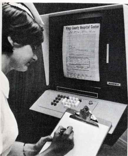
**Ampex's Videofile™ Information System** is just what the doctor ordered for the handling of massive, dynamic document files. This installation is at a hospital complex. Doctors and nurses throughout its 23 clinics, with the help of Videofile, have rapid access to the medical record of any patient, either as a TV picture or as hard copy.
