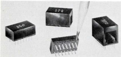
These 14-pin headers, with caps, have gold plated pins laid out in the std. 0.100 x 0.300 in. DIL grid. U-shaped openings in the tops of the pins accept component leads to wire size 24. Soldering is the normal means of component attachment. \$0.75 to \$1.20 ea. (< 100 pcs.). Design & Production Associates, 1600 N. Arrowhead Ave., San Bernardino, Calif. 92405. (714) 886-8612.
