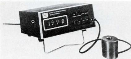
The Model 10A uses feedback techniques for short and long term stability and linearity. The instrument measures from  $10^{-3}$  to  $10^5$  ft. candles and ft. L or  $10^{-9}$  W to  $10^{-1}$  W within a spectral range from 2200 to 11,500 Å. You can also get a 10B telephotometer/microphotometer lensing system and fiber optics probes as accessories. United Detector Technology, 1732 21st St., Santa Monica, Calif. 90404.
