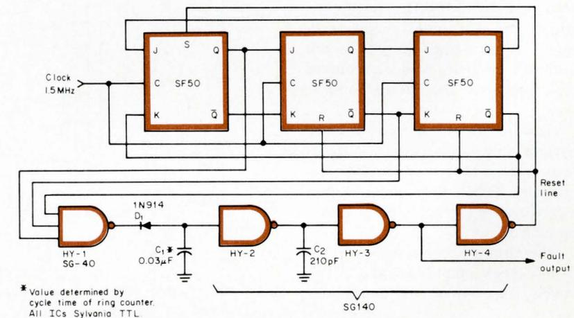
reaches the logic threshold level, HY-2 sends a logic 0 through HY-3 and HY-4 to reset the counter. This, in turn, forces HY-1's output to drop to a 0 and discharge  $C_1$  through  $D_1$ . The input to HY-2 thus drops below threshold, removing the reset pulse.
