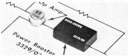
You can use the Model 3329/03 in cascade with all general purpose op amps. It functions as a high current output stage and is used inside the feedback loop as though it were an integral part of the op amp. Unit price is \$20.00. Burr-Brown Research Corp., International Airport Industrial Park, Tucson, Ariz. 85706. (602) 294-1431.
