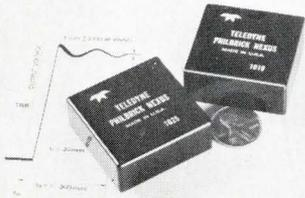
Model 1025 FET input op amp settles to 0.01% of final value in 300 ns. Designed for inverting applications, it also offers a wideband positive input with a  $\pm 2$  V common mode range. Gain bw product is 50 MHz and open-loop gain is 100,000. Output is  $\pm 50$  mA at  $\pm 10$  V, with a slew rate of 500/ $\mu$ s over a temp. range of  $-25$  to  $+85^\circ\text{C}$ . \$75.00 (1-9). Teledyne Philbrick Nexus, Allied Dr. at Rte 128, Dedham, Mass. 02026. (617) 329-1600.
