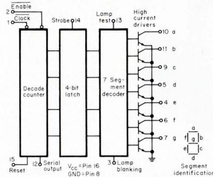
**MC4050 Counter-Latch-Decoder.** Resetting the input suppresses the leading zeroes in a display. The lamp blanking input allows control of display brightness through control of the duty cycle, and a lamp test input permits verification of all diode integrity.
