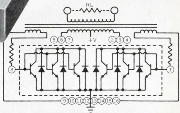
Take RCA transistor chips with current capabilities up to 80 A, rectifiers with peak currents to 80 A, and resistors to 10 watts. Interconnect them — in any number of ways. What do you get? A power capability up to 800 W, current capability up to 300 A!
