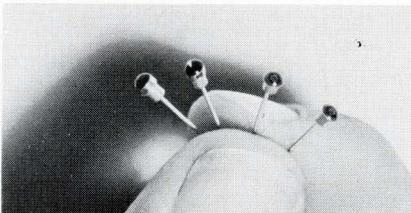
Solid-Lite red light-emitting lamps use GaP electroluminescence for brighter light at lower current. Compatible with IC output, they produce 2 mcd luminous intensity at only 15 mA drive current. OSL-1 provides wide-angle viewing with good visibility over  $180^\circ$ ; OSL-2 features higher luminous intensity with a narrower viewing angle. OPCOA Inc., 330 Talmadge Rd., Edison, N.J. 08817.
