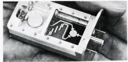
All that's needed to form a complete microwave Doppler radar is the module, an antenna, a display, and a power source. Possibilities for consumer uses include automobiles, private airplanes, and pleasure boats. The radar will be used in industrial applications such as intrusion alarms, automatic traffic controls, railroad speed controllers, and automatic aircraft landing systems.
