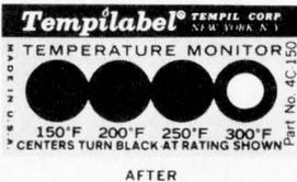
Self-adhesive Tempilabels<sup>o</sup> assure dependable monitoring of attained temperatures. Heat-sensitive indicators, sealed under the little round windows, turn black and provide a permanent record of the temperature history. Tempilabel<sup>o</sup> can be removed easily to document a report.
