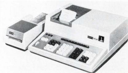
Printed tape output is a feature of this computer. It has a programming capability of 256 steps, a dynamic range of  $10^{-99}$  to  $10^{99}$ , and it can be programmed for 85% of commonly encountered technical, engineering and scientific computations. Eugene Dietzgen Co., 2425 N. Sheffield Ave., Chicago, Ill. 60614. (312) 549-3300.
