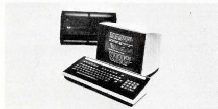
Up to 32 video displays may be connected to, and controlled by, a System IV/70 which, in turn, communicates with a central computer facility.
