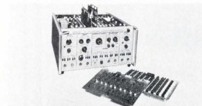
Model SAI-54 provides fine line resolution spectral analysis from dc to 1 MHz in 10 selectable bands. This unit processes complex signals for study, evaluation, identification and analysis in vibration testing, medical diagnosis, acoustics, radar and oceanography. \$13,000. Signal Analysis Industries Corp., 595 Old Willets Path, Hauppauge, N. Y. 11787.
