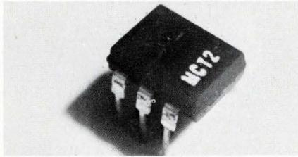
The MCT2 consists of a diffused planar IR light-emitting diode optically coupled to a silicon planar photo-transistor. Voltage isolation exceeds 1500 V and isolation res. is typ. 100 G $\Omega$ . It also has a current transfer ratio of 35% and rise and fall times of 2  $\mu$ s. \$5.85 ea. (1-9) and \$3.55 ea. (1000). Monsanto Co., 10131 Bubb Rd., Cupertino, Calif. 95014. (408) 257-2140.
