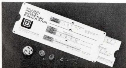
This silicon photodetector calculator helps you get the best performance out of your photodetectors. Most of the scales are general purpose and can be used for almost all types of photodetectors, including photomultipliers and phototransistors. \$1.00 with instruction book. United Detector Technology, 1732 21st St., Santa Monica, Calif. 90404. (213) 393-3785.
