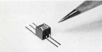
Model 4211-1007 microminiature audio transformer is a low-profile unit, only 0.125". It has a freq. range of 4 kHz to 40 kHz. Power rating is 10 mW at 20 kHz. It meets Mil-T-27, grade 5, and features electrostatic shielding. Bourns Pacific Magnetics Corp., 28151 Highway 74, Romoland, Calif. 92380. (714) 657-5195.
