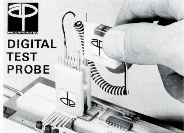
WATCH THIS LOGIC SLEUTH DETECT TRUE LOGIC "1" AND LOGIC "0" LEVELS ON YOUR OWN CIRCUITS
