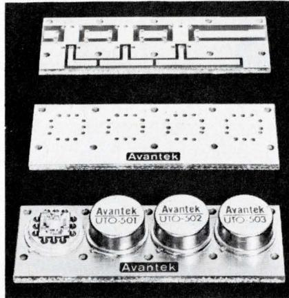
**Just solder them in.** New gain modules take the work out of broadband circuit design. Stable, repeatable, and cascadeable, each TO-8 can has 14 dB of gain and a 5-500 MHz,  $\pm 1$  dB response. (Extra flatness is available to order.) Shown here is an optional 4-socket PC board; 1-, 2-, and 3-socket boards are also available. You can order assembled cascades and shielded cases as well.
