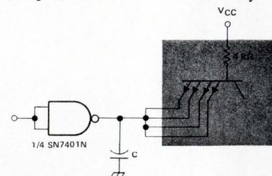
**Schmitt trigger in pulse-stretcher circuit**
