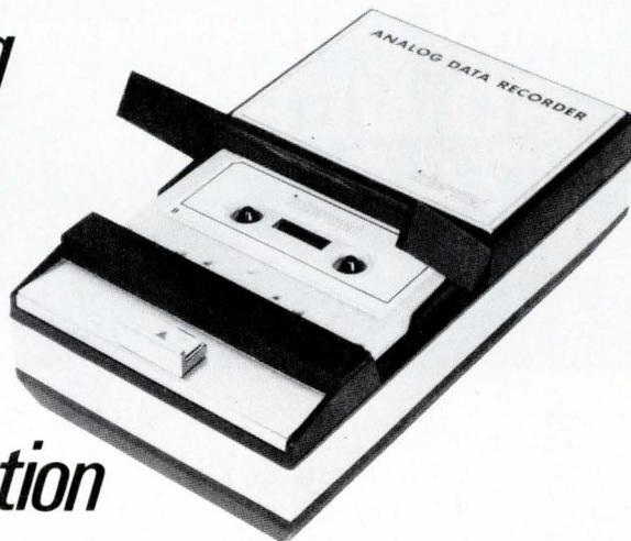
Design features include four hours of simultaneous four-channel record time; PWM electronics with 33 dB dynamic range; standard C-120 cassette tapes; a self-contained battery power supply; and a three pound package.
