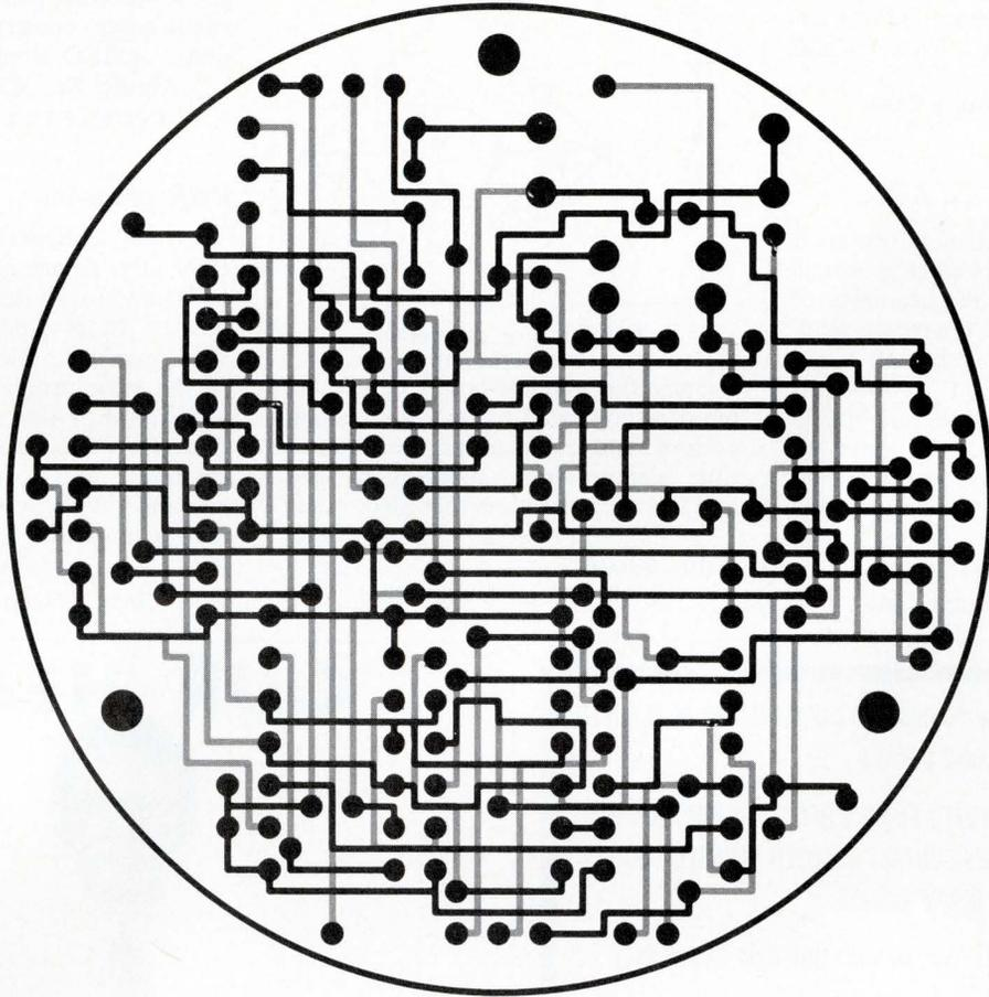
*Computerized two-layer printed circuit board interconnection artwork produced by Electronic Graphics, Inc. Shown twice actual size.*
