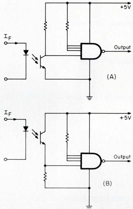
**A Schmitt trigger circuit** using an optical couple to interface with TTL offering fast rise and fall times with an isolated signal input. Figure A provides a non-inverting function, while Fig. B provides an inverting function.—Texas Instruments.
