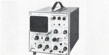
The SM111 has a dc to 18 MHz bandwidth, sensitivity of 2 mV/cm to 50 V/cm, timebase of 200 ns/cm to 1 s/cm, and a 10 cm x 8 cm CRT. The scope is powered by either ac or an optional self-contained battery pack. Available from stock, it costs \$1,195. B & F Instruments, Inc., Cornwells Heights, Pa. 19020.
