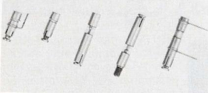
The 7200 series trimmer capacitors are for ic, hybrid circuit, microstrip circuit and microwave applications. They have a 10:1 tuning ratio and offer capacitances ranging from 0.1 to 2.0 pF. Made of gold plated brass, they use high K glass and alumina ceramics. Johanson Mfg. Corp., 400 Rockaway Valley Rd., Boonton, N.J. 07005.
