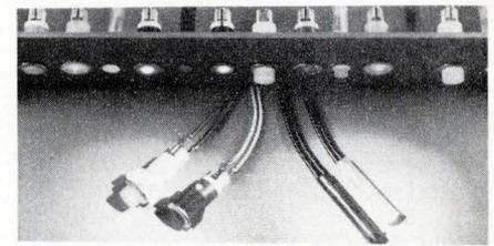
Pre-assembled nylon encased neon and incandescent Ampillum<sup>TM</sup> lights are self-mounting in panels 0.032 to 0.062 in. thick. Standard lens styles are "top hat" and "flush." Both types come with natural red, orange, or yellow lenses with 125 or 250 V ratings. Incandescents are also available in blue, green, and purple and 6.3, 12, and 24 V ratings. AMP Inc., Harrisburg, Pa. 17105. (717) 564-0101.
