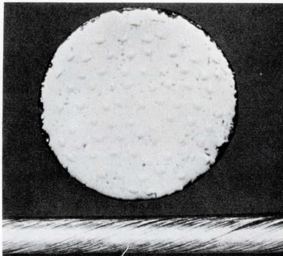
**Superconducting wire** by Whittaker, 0.002-in. diameter, looks something like a pancake on a griddle when magnified 638 times (top). What appear to be "bubbles in the batter" are actually the ends of individual niobium-tin filaments in the wire's copper matrix. At bottom is a microscopic view of Norton's multifilament superconductor containing more than 400 highly stable niobium-titanium alloy filaments, each only 0.007 in. in diameter, embedded in a copper matrix.
