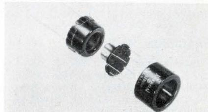
Operating without thermostatic controls, this ss component stabilizer self-stabilizes itself and contained TO-5 component at  $65^{\circ}\text{C}$  in  $< 1$  min. Drawing  $< 1$  W in its steady state at room temp., it operates over ambients from  $-55^{\circ}$  to  $15^{\circ}\text{C}$  below its control temp. Operating voltage is 24 V ac or dc. Texas Instruments Incorporated, Control Products Div., Attleboro, Mass. 02703. (617) 222-2800.
