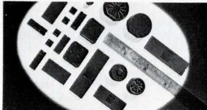
AlSiMag<sup>®</sup> 782 alumina ceramic parts offer a new safeguard for light-sensitive electronic devices. This opaque black material is used for encapsulation and as a substrate. It has a helium leak rate of  $< 1 \times 10^{-8}$  cc/s at one atmosphere pressure and can be reheated in an oxygen atmosphere without color change. American Lava Corp., Chattanooga, Tenn. 37405.
