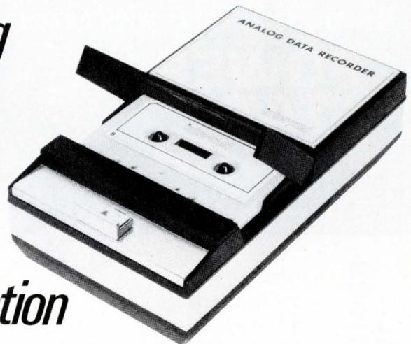
Design features include four hours of simultaneous four-channel record time; PWM electronics with 33 dB dynamic range; standard C-120 cassette tapes; a self-contained battery power supply; and a three pound package.
