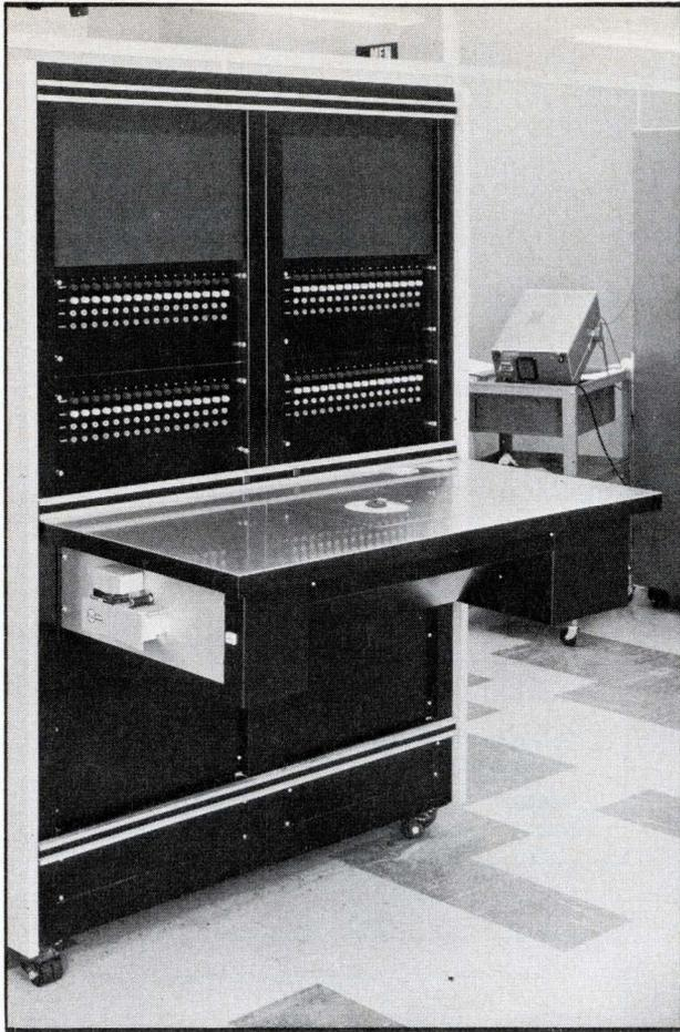
This is Redcor's PAFT II (Programmable Automatic Function Tester). The system uses a RC-70, 16-bit computer as the center of the test system.
