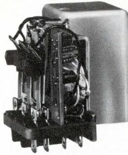
This hybrid impulse relay is unique. Its basic structure is our KUL, a single coil latching relay employing a shunting-type magnetic circuit. To that we have added a solid state flip-flop circuit to obtain a truly modern, alternate-action, impulse relay.
