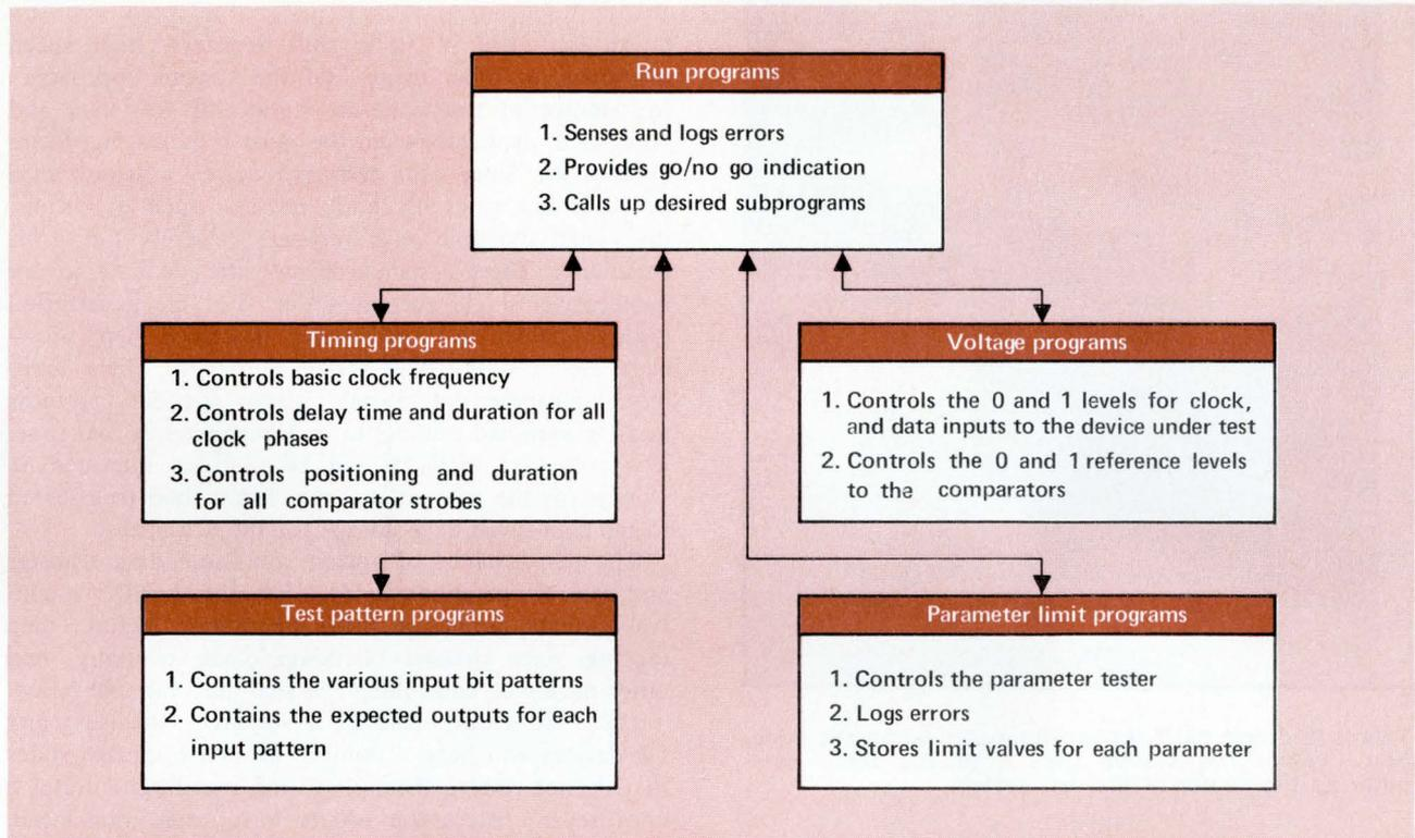
The software system for a programmable functional tester should include at least all the functions shown.
