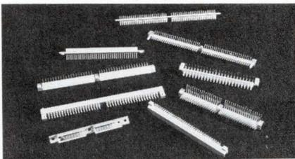
These circuit-card header systems are connectors consisting of extruded or fabricated aluminum bases containing male blade contacts on 0.100 in. (type M1001), 0.125 in. (type M1201), or 0.150 in. (type M1501) centers. The contacts, when used with mating tuning fork contacts, offer low insertion force, typ.  $< 6$  oz./mated pair. Teradyne Components, 900 Lawrence St., Lowell, Mass. 01852. (617) 454-9195.
