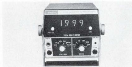
Model 262A measures dc voltage and current, ac voltage and current and ohms. The multimeter has a basic dc accuracy of 0.1% of reading. All dc ranges feature automatic polarity indication and automatic zero correction circuitry gives you maximum stability. \$375. United Systems Corp., 918 Woodley Rd., Dayton, Ohio 45403. (513) 254-6251.
