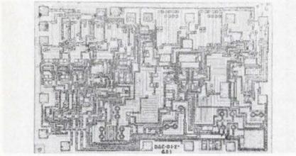
The monoDAC-01 converter is a 6-bit current steering converter. It consists of an internal voltage reference, six precision current sources, six current steering logic switches, a diffused resistor network, and an internally compensated output op-amp. \$40 ea. in quantities of 100. Precision Monolithics Inc., 1500 Space Park Dr., Santa Clara, Calif. 95050.
