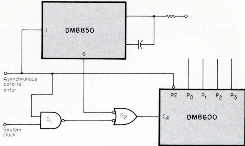
stable entry of data. The third function is the initiation of the one-shot which provides the clock pulse for the parallel entry.
