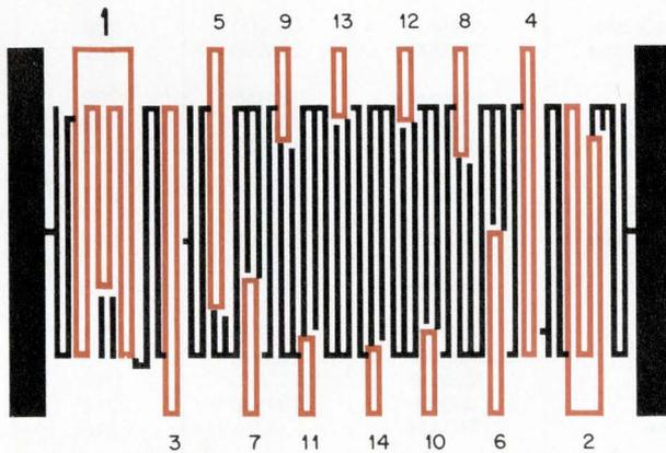
**Fig. 1. A 1,300-square thin-film resistor pattern with parallel adjustment loops. A portion of each loop is common to the main conducting path. Opening the loop removes a shunt according to the following values:**
