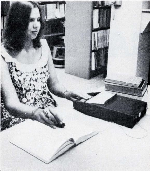
**Candy Linville** is using an optoelectronic device to convert printed matter into Braille for reading by the blind. The experimental device was developed by her father, Professor John Linville of Stanford.
