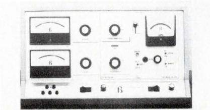
This plug-in module is used with the manufacturer's Model 70 test set to measure transistor high freq. parameters. You can test both pnp and npn transistors from 20 MHz to 100 MHz. The new module is \$690 and the Model 70 test set is \$945. Birtcher Corp., Instrument Div., 1200 Monterey Pass Rd., Monterey Park, Calif. 91754. (213) 264-6610.
