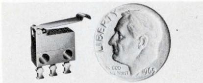
New Mini-Mite™ has a case that is <math>< 0.250</math> in. high by 0.300 in. wide by 0.100 in thick. Ratings are 2 A, 125-250 Vac; 2 A (res.) and 1 A (ind.), 30 Vdc. The switch, which meets Mil-S-8805 specs, is available with four types of terminals—single and double turret, quick connect spade and solderless wrap. McGill Mfg. Co., Inc., Valparaiso, Ind. 46383.
