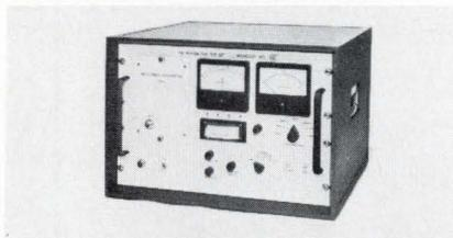
Model 1216 measures deviations from  $\pm 100$  Hz to  $\pm 2$  MHz. It has an accuracy of  $\pm 2\%$  of full scale and is internally self-calibrating to within  $\pm 0.1\%$ . You can use the test set with telemetry, television and microwave communications. Instrumentation Div. of Microdot Inc., 220 Pasadena Ave., So. Pasadena, Calif. 91030. (213) 682-3351.
