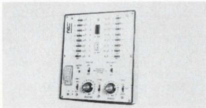
The Model ICT-200 uses individual switches to apply dc voltage levels, a pulse, or a square wave function to any of up to 16 pins. A selectable meter allows rapid verification of the IC's operation and output voltage levels. Unit price, \$199. Innovation Development Co., Box 7, Azusa, Calif. 91702.
