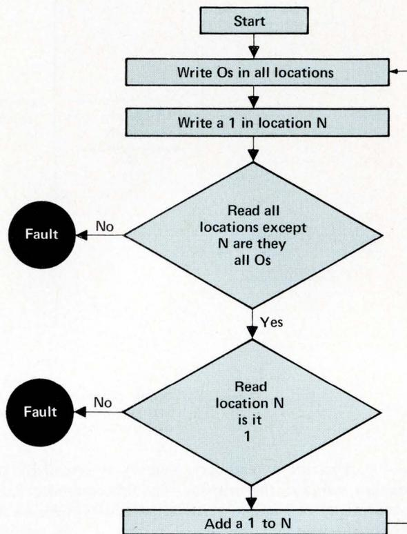
A typical test for a read/write memory consists of walking a 1 through all locations in the memory. The same approach can be used to walk a 0 through the memory.
