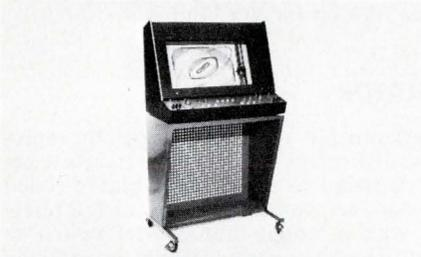
The Gould 100 produces clear, uniform traces even for discontinuous plots and at crossover points of lines. A disposable plastic ink cartridge has sufficient capacity for 40 miles of trace. Total response time to a full scale step input is 300 ms. maximum. Brush Instruments Div., Gould Inc., 3631 Perkins Ave., Cleveland, Ohio 44114. (216) 361-3315.
