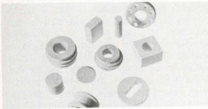
This desiccant is strong enough to be a mechanical part, workable enough to be machined into nearly any shape, and weighs only 1.1 g/cc. Natrasorb® 900 will absorb about 18% of its own dry weight in moisture vapor under std. conditions (25°C. 10 mm Hg. water vapor pressure) and can dry atmospheres to a -100°F dew point. Multiform Desiccant Products, Inc., 1418 Niagara St., Buffalo, N.Y. 14213. (716) 881-0100.
