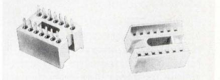
Type 561 socket fits 14-pin DIL ics on 0.100 in. centers for adjacent terminals. Consistently reliable mating of the ic package is achieved by using a tapered pin entrance design. Solder tail centers of the socket are identical to those of the ic, permitting std. board layouts to be used. About \$0.20 ea. Connector Corp., 6025 N. Keystone Ave., Chicago, Ill. 60646. (312) 539-3108.
