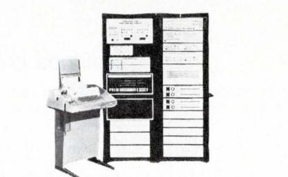
The W102 controls x-y positioning optics and a trimming laser to adjust up to 20 resistors on a single chip while simultaneously checking dc circuit operation. It can process 3000 typical substrates (eight resistor voltage regulator)/h. A basic system is priced at \$77,900. Teradyne Applied Systems, 4034 N. Nashville Ave., Chicago, Ill 60634.
