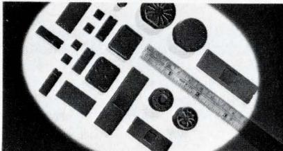
AlSiMag® 782 alumina ceramic parts offer a new safeguard for light-sensitive electronic devices. This opaque black material is used for encapsulation and as a substrate. It has a helium leak rate of  $< 1 \times 10^{-8}$  cc/s at one atmosphere pressure and can be reheated in an oxygen atmosphere without color change. American Lava Corp., Chattanooga, Tenn. 37405.
