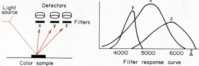
The need often arises to make quantitative measurements for color matching or color control in a wide variety of industrial and laboratory applications. This is done by using photocells and filters for color synthesis, color process control, color matching and color identification. Some applications include fruit ripeness testing, textile matching, paint mixing and process control.—United Detector Technology.
