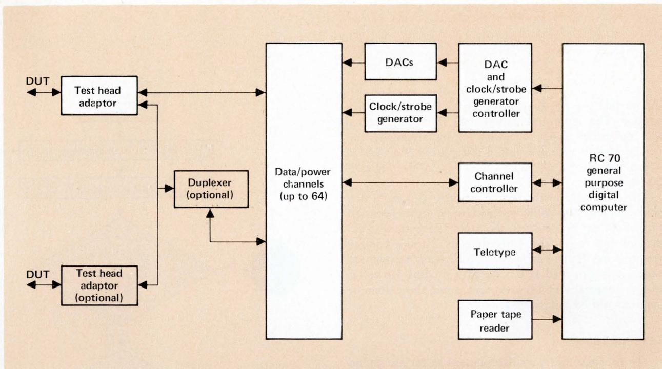
**Block diagram of the PAFT II system.** The system performs parameter testing, such as stress and leakage and functional tests.
