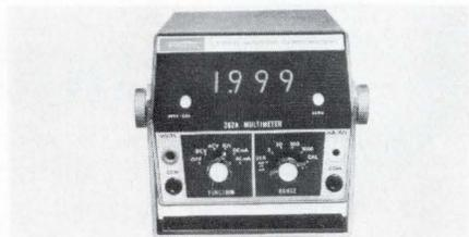
Model 262A measures dc voltage and current, ac voltage and current and ohms. The multimeter has a basic dc accuracy of 0.1% of reading. All dc ranges feature automatic polarity indication and automatic zero correction circuitry gives you maximum stability. \$375. United Systems Corp., 918 Woodley Rd., Dayton, Ohio 45403. (513) 254-6251.
