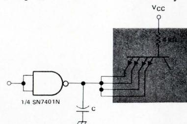
**Schmitt trigger in pulse-stretcher circuit**
