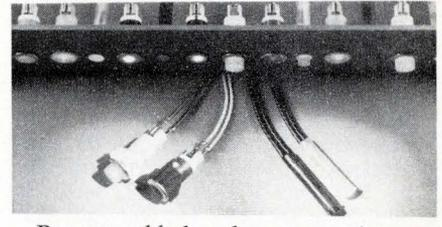
Pre-assembled nylon encased neon and incandescent Ampillum<sup>TM</sup> lights are self-mounting in panels 0.032 to 0.062 in. thick. Standard lens styles are "top hat" and "flush." Both types come with natural red, orange, or yellow lenses with 125 or 250 V ratings. Incandescents are also available in blue, green, and purple and 6.3, 12, and 24 V ratings. AMP Inc., Harrisburg, Pa. 17105. (717) 564-0101.
