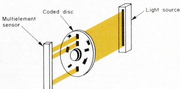
Shaft encoders use multiple unit optoelectronic light sensors. A shaft position encoder, also referred to as a "converter" or "coder", is a device which transduces mechanical analog shaft rotation into digital representation. It will give a separate distinct digital indication for each position of the shaft, and the rotation can be divided into as high a number of segments as necessary.—Centralab.
