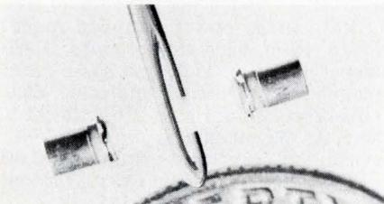
SE 2450 GaAs emitter and SD 2440 silicon detector are offered as a matched-pair combination of a source and sensor. They are well suited for high-density PCB mounting. Uses include punch card and tape readers, character recognition, shaft encoders, position indicators and warning devices. Spectronics Inc., 541 Sterling Dr., Richardson, Tex. 75080. (214) 231-9381.
