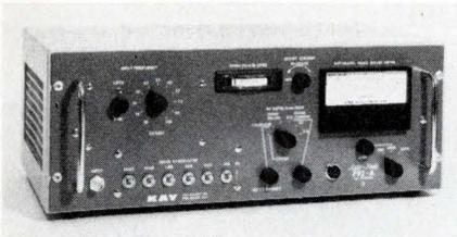
Model 792A1 has a 75  $\Omega$ , 10 to 250 MHz tuned amplifier input and a 75  $\Omega$ , 10 to 1000 MHz full range noise head. The meter provides noise figure readings from 0 to 20 dB for the 6 dB reference and 3 to 30 dB for gas tube and solid state sources. \$840. Kay Elemetrics Corp., 12 Maple Ave., Pine Brook, N. J. 07058.
