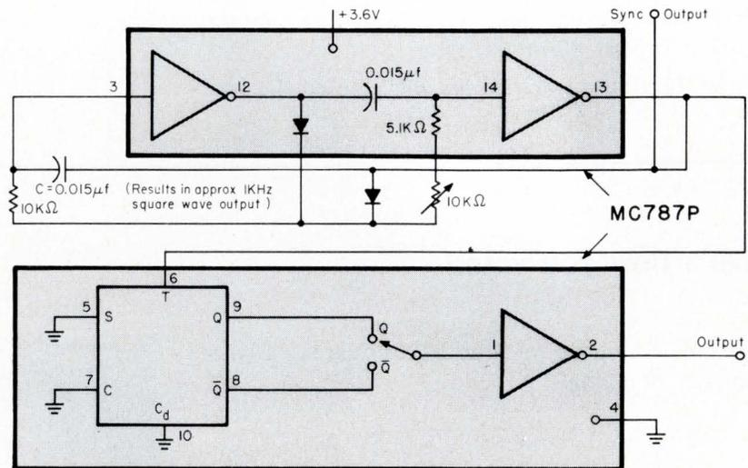
put frequency of about 1 kHz for the RC values shown. A variable frequency control, sync output and
