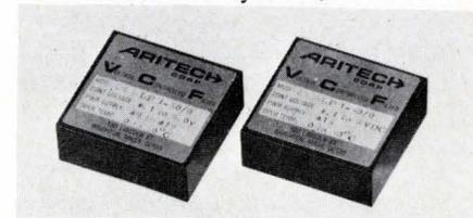
These filters are for dual or multichannel systems for simultaneous processing of signals or for multiple channel recording. They come in the range from 0.1 Hz to 100 kHz. Matched fixed filters are being produced to within  $\pm 1^{\circ}$  in phase and  $\pm 1/4$  dB in amp. Voltage Controlled Filters (VCF's) track to within  $2^{\circ}$  and  $\pm 1/2$  dB over a 50:1 freq. range. < \$100 (in quan.), Aritech Corp., 130 Lincoln St., Brighton, Mass. 02135. (617) 254-2990.
