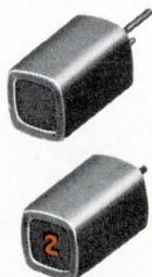
Pusher "legs" on back of button are connected to internal fluorescent illuminator which actuates the "glow." When you push the button "in" the internal fluorescent illuminator is put in contact with the front screen and legend glows brightly . . . even in very high or very low ambient light situations. Release, it's out. Won't lose its brilliance. 2 types: white-face button has visible legend whether button is "in" or "out," black-face button has visible legend only when button is "in."
