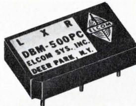
Model DBM-500PC has an rf and LO input frequency of 2 to 500 MHz and an i-f which operates from dc to 500 MHz. You can use the unit as a mixer, balanced modulator, rf switch and phase detector. Prices range from \$12 to \$24, with delivery from stock to 30 days. Elcom Systems Inc., 151 W. Industry Court, Deer Park, N.Y. 11729. (516) 667-5800.
