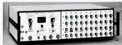
RUN, the instrument automatically recycles at the finish of the last step of a waveform. In GATE, the instrument free-runs as long as an external command signal (+2 V, DTL/TTL compatible) is applied or a panel push-button is depressed. In 1 STEP, you can advance the waveform one step at a time. And in 1 CYCLE, the instrument completes one waveform cycle (all steps) for each push-button signal.
