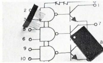
The MN304 is a quad, two input non-inverting power gate with four transistor output stages. The unit has an output voltage rating of 50 V and output current of 200 mA/output stage. Operating range is 0 to 70°C. Available from stock, the unit price is \$13.50. Micro Networks Corp., 5 Barbara Lane, Worcester, Mass. 01604. (617) 756-4635.
