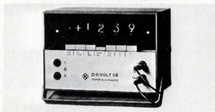
The UGWD measures dc and ac voltages from 100  $\mu$ V to 1000 V and resistances from 1  $\Omega$  to 15M $\Omega$ . It is an integrating voltmeter that uses the dual slope technique and it has a true integrating time of 300 ns and a sampling rate of 3 measurements/s. \$750. Rohde & Schwarz, 111 Lexington Ave., Passaic, N.J. 07055.
