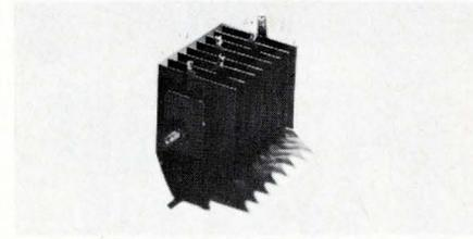
You can use these units to build custom rectifiers. The plates are rated at either 30 PIV, 25 V rms (style PT), or 36 PIV, 30 V rms (style PU), and range from 0.5 A capability to 173 A in 24 sizes from 1 in.<sup>2</sup> to 8 x 16 in. Plates are stacked for the required voltage and circuit configuration. Siemens Corp., Components Div., 186 Wood Ave. So., Iselin, N.J. 08830. (201) 494-1000.
