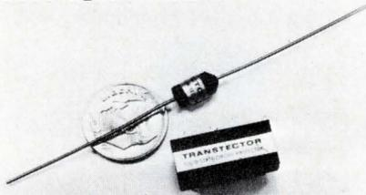
This line of hybrid SCR crowbar circuits protects transistors, ics and multilayer circuit boards from overvoltage transients. Transrector Circuit Protectors™ have operating current levels of up to 10 A. They can be ordered with std. overvoltage trip points ranging from 5 to 200 Vdc. Standby power loss runs <1 mW/V. Transrector Systems, 1161 Monterey Pass, Monterey Park, Calif. 91754.
