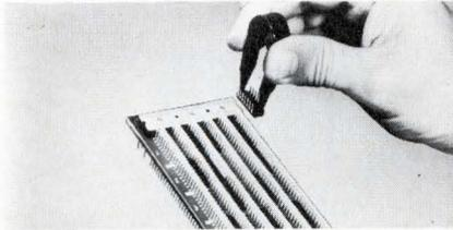
DIP-PAC is a pluggable DIL packaging system with contacting fingers that permit the DIP to be inverted and plugged into the system. DIP-PAC provides an integrated ground and voltage plane on the wiring side connected to dummy pins or specified DIP locations. Tail side of the system is arranged for automatic wiring. It comes in std. sizes of 30, 60, 90, 120, 150 and 180 DIP positions. Elfab, Box 34555, Dallas, Tex. 75234. (214) 239-7181.
