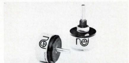
Standard models come in both servo and bushing designs with a 7/8 in. dia. and a choice of a 1/8 or 1/4 in. dia. shaft. All have infinite resolution, resistance ranges from 1 k  $\Omega$  to 10 k  $\Omega$ , and linearities from 1 to 0.25%. Power rating is 1 W at  $70^{\circ}$ C, de-rated to 0 at  $125^{\circ}$ C. \$4.99 (100 units). New England Instrument Co., Kendall Lane, Natick, Mass. 01760. (617) 873-9711.
