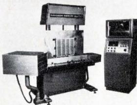
Model 15YN is a useful companion to the fully automatic Wire-Wrap® machine, answering the needs of those whose wire terminating requirements are 1,000,000 wires/yr. It is well suited for handling twisted pair wires and those wire gauges that are not normally wrapped on the automatic machine. Standard equipment includes terminal locator capable of wiring an area 24 x 36 in., lighted wire bin (32 tubes), and a ss numerical control. Gardner-Denver Co., Gardner Expressway, Quincy, Ill.
