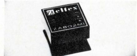
Model ZA802M1 features 15 pA (max.) input current; 100,000:1 CMR and 4 MHz (unity gain) freq. It has a max. input voltage drift of 50  $\mu$ V/ $^{\circ}$ C (-25 $^{\circ}$  to 85 $^{\circ}$ C). Price/performance ratio make it attractive for use in current-to-voltage conversion, integration, buffering, sample/hold operations, and differential amplification. \$26 (1-9). Zeltex, Inc., 1000 Chalmar Rd., Concord, Calif. 94520. (415) 686-6660.
