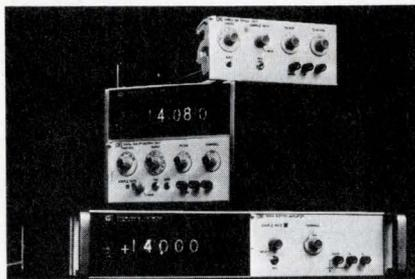
**Take your choice.** Hewlett-Packard's new multifunction, 4-digit DVM uses the D/A conversion technique of successive approximation to reach a reading rate of 1000/s for dc measurements. In addition, it uses a proprietary thermopile to read true rms values that can include the dc component. Three plug-ins, two mainframe styles, and three options within the mainframe itself give Model 3480 a wide range of configurations.
