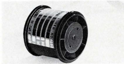
Nanos® is a compact (1 in. in dia. by 1 in. long), hf fan that provides up to 7.5 cfm free delivery. It withstands 100 g shock in any direction, operates from  $-55^{\circ}$  to  $+100^{\circ}$ C, and may be mounted in any attitude. Air-flow is reversible by turning the fan end-for-end. Power requirement is 26 Vac, 400 Hz, 1  $\phi$ . Rotron Inc., Hasbrouck Lane, Woodstock, N.Y. 12498. (914) 679-2401.
