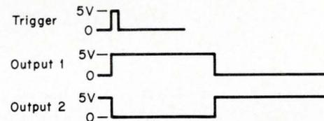
voltage on the capacitor exceeds the threshold voltage of the gate, the gate output goes low and resets the flip-flop. The capacitor now discharges rapidly through the diode
