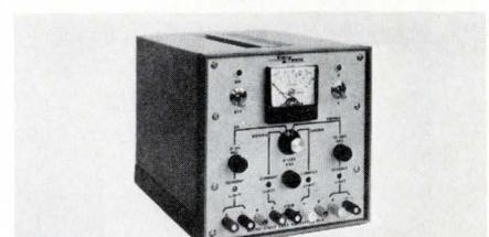
Model 401 has four power supplies in one cabinet. The logic section furnishes 3-5 Vdc at 3 A with overvoltage protection. The linear section has dual tracking dc outputs of 0.5 A, adjustable from 6-18 V. The mos/relay section provides 0.5 A, from 15-28 V. \$295. Astro-Space Laboratories, Inc., 110 Wynn Dr., N.W., Huntsville, Ala. 35806.
