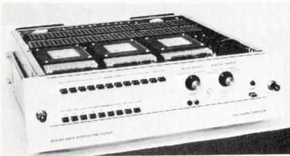
Model MDD1-06 accepts digital information from a computer along with channel address data, converts it into equivalent analog form and then distributes it to selected output holding amplifiers. System accuracy is 0.05% FS  $\pm 1/2$  LSB and linearity is 0.03% FS  $\pm 1/2$  LSB. Raytheon Computer, 2700 S. Fairview St., Santa Ana, Calif. 92704. (714) 546-7160.
