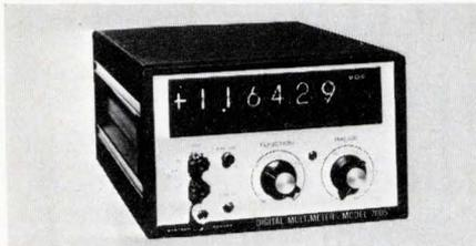
Model 7005 features a 5½-digit readout with  $\pm 0.005\%$  accuracy. The standard unit provides a resolution of 0.001% (10  $\mu$ V) or you can increase it to 1  $\mu$ V with a plug-in card (\$225 option). DC measurements can be made up to 5 samples/s. \$1295. Sys-tron Donner Corp., 888 Galindo St., Concord, Calif. 94520.
