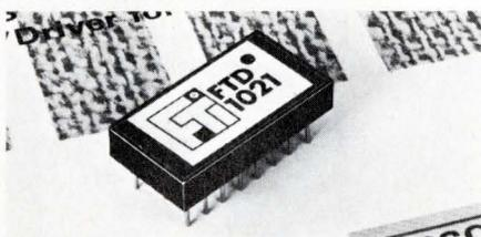
The FTD-1021 decodes BCD inputs to drive 7-segment cold cathode displays. Each output has a 100 V standoff rating at 2  $\mu$ A standoff current. In the on state, each output can sink 20 mA continuously, with 50 mA surge currents, \$10.50 in 100 quantities. Fabri-Tek Micro-Systems, Inc., 1150 N.W. 70th St., Ft. Lauderdale, Fla. 33309. (305) 933-9351.
