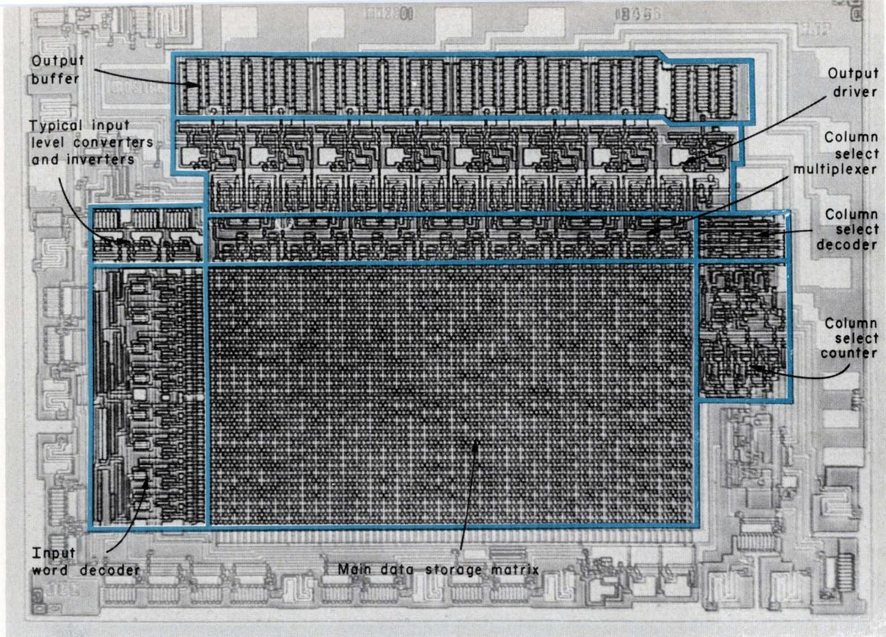
This completely decoded ROM shows the space allocations for the different types of circuitry required.
