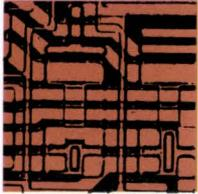
Fairchild's new 9340 is the perfect arithmetic logic unit for almost every application. It's a high-speed device that can perform two arithmetic operations (ADD or SUBTRACT) and any of six logic operations on two 4-bit binary words in parallel. To handle 16 bits, just hook up four 9340s.
