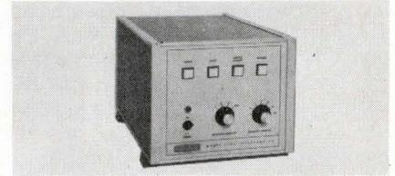
The 3108 not only automatically turns on the teletype to record a sample, but also removes power from the TTY 6 seconds after each conversion cycle. This increases the life of the ASR 33 teletype which is designed for intermittent use only.
