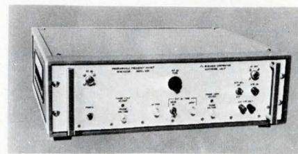
Model 6011 is available in L, S, C, X or Ku-band and preserves a-m and fm modulation characteristics of the input signal. Key technical characteristics include up to 1000 MHz rf bandwidth, 20 MHz fm bandwidth, and  $\pm 500$  kHz freq. offset range. ITL Research Corp., 8955 Quartz Ave., Northridge, Calif. 91324.
