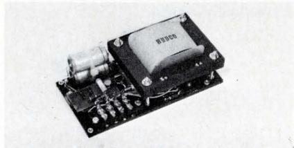
Miniaturization is achieved in the Model HM5-4 without switching techniques; thus there is no switching noise and/or spikes in the dc output. The 5 V unit is rated at 4 A at  $71^{\circ}$ C. It works from 105 to 125 V, 50 to 500 Hz. Regulation is  $\pm 0.25\%$  for line and load changes. Ripple is 4 mV rms max. Response time is 50  $\mu$ s max. \$48 (100 to 499). Hudco, 2740 S. La Cienega Blvd., Los Angeles, Calif. 90034.
