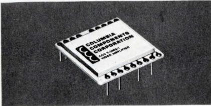
Each D-3000 series module has a high slew rate output amplifier, ladder network, internal voltage reference and high speed switching circuits. The series includes units with accuracies of 8 or 10 bits binary or 12 bits BCD. The output, 100 mA at +5 V, is short-circuit proof. Columbia Components Corp., 60 Madison Ave., Hempstead, N.Y. 11550. (516) 483-8200.
