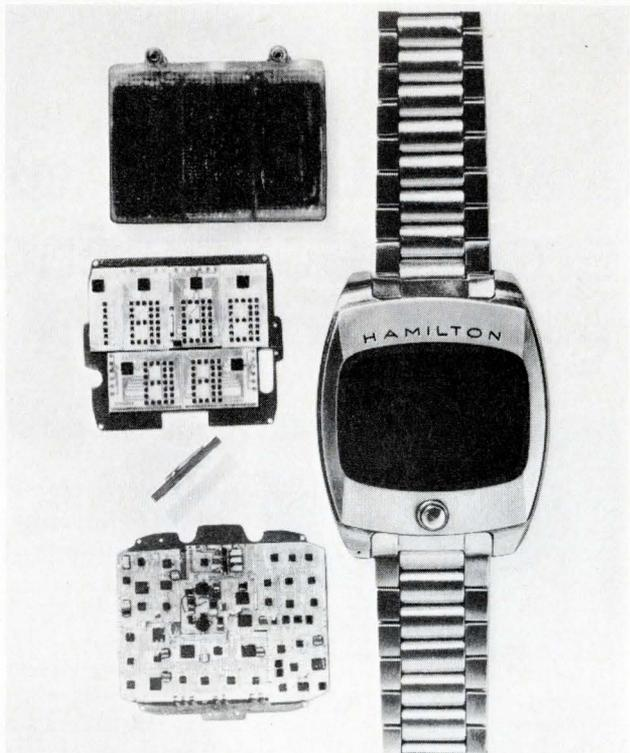
Pulsar's major components are (top to bottom), a  $4\frac{1}{2}$ -V rechargeable battery, a computer module (display side), a quartz crystal, and the logic side of the computer module. They all fit into a case the size of a normal wristwatch (rt.). The time will appear on the face of the timepiece only when the demand button is pressed.
