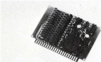
Seven new converters each provide a complete system element. All are available with bipolar or unipolar output. All that is needed to operate any unit in the DAC-A series is a  $\pm 15$  V supply. All units are completely self-contained. Temperature coeff. is  $\pm 5$  ppm/ $^{\circ}$ C. They are TTL compatible. Phoenix Data Inc., 3017 W. Fairmount Ave., Phoenix, Ariz. 85017. (602) 277-4767.
