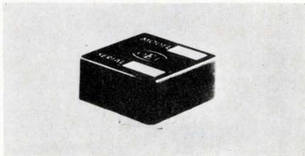
Model 9428 lets you build hf analog systems operating from limited power (battery) sources. Heat build up in large complex analog systems is no longer a problem with the low power 9428. It features:  $\pm 500$  V/s slewing rate, 80 dB min. open loop gain, 100 MHz closed loop BW, 70 ns settling time to 0.1% residual error and  $\pm 10\%$  V at  $\pm 30$  mA output current capability. \$76 (1-2). Optical Electronics, Inc., Box 11140, Tucson, Ariz. 85706. (602) 624-8358.
