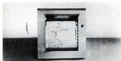
Available in six case configurations, this unit has 0.5 s full scale response, potentiometric input impedance, source impedances to 10,000  $\Omega$ , sensitivity to 1 mV, and accuracy of 1%. It comes in any of the manufacturer's three direct writing styles. Esterline Angus, div. of Esterline Corp., Box 24000, Indianapolis, Ind. 46224. (317) 632-6501.
