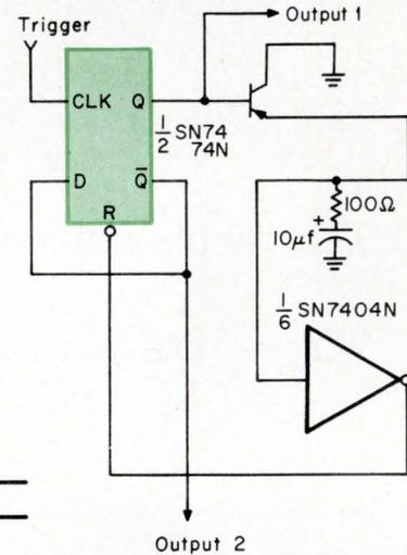
(or transistor) and the output transistor of the flip-flop. With the capacitor discharged, the output of the gate goes high again and the circuit is ready for the next pulse.
