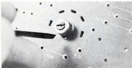
First of a projected line of switches in transistor cans, the TO-5 rotary switch is for circuit selection on pcs. The screwdriver-actuated switch is SP7T 8-pos., one position off. It has a positive detent action holding the switch in each position, contacts plated with 30  $\mu$ in. of gold over 30 nickel, and easy assembly. Chicago Switch, Inc. 2035 W. Wabansia Ave., Chicago, Ill. 60647. (312) 489-5500.
