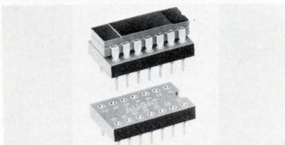
Low profile body of these 14 and 16 contact DIL sockets is made of glass filled nylon. Machined contacts are beryllium copper, gold over nickel plated. Sleeves are brass, gold over nickel plated. Body dimensions are 0.450 in. max. x 0.750 in. max. x 0.180 in. max. \$0.78 to \$1.41. Augat Inc., 33 Perry Ave., Attleboro, Mass. 02703. (617) 222-2202.
