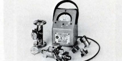
This ThruLine<sup>®</sup> coaxial wattmeter is an insertion type instrument for measuring forward and reflected cw power in 7/8 in. EIA and in rf cable transmission lines. It measures rf power flow with an accuracy of  $\pm 5\%$  in discrete frequency bands from 0.45 MHz to 2.3 GHz. Bird Electronic Corp., 30303 Aurora Rd., Cleveland, Ohio 44139. (216) 248-1200.
