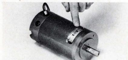
New line of dc permanent magnet servo motors is for computers, business machines, machine tools, and similar applications. They come in 2.5, 3.3, 4.0, and 6.0 in. diameters and with many shaft configurations. Units can be supplied in 18 std. armature windings for 6 to 120 Vdc service. Speed of the motor line ranges to 6000 rpm (no load) with stall torque ratings of 75 to 1600 oz-in. AMETEK/Lamb Electric, 629 Lake St., Kent, Ohio 44240. (216) 673-3451.
