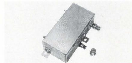
Model 2510-1 tunable preselector tunes the 116-150 MHz band and has 15 W capability. Two screwdriver controls tune it to any vhf freq. Loss is 4 dB max. and rejection at  $\pm$ 2 MHz is 30 dB min. It has miniature connectors and brackets for systems mounting. \$95.00. Microwave Filter Co., Inc., 135 W. Manlius St., East Syracuse, N.Y. 13057.
