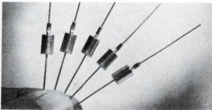
TransZorb® transient voltage suppressors come in voltages from 6.8 to 200 V (JEDEC types 1N5629 through 1N5665A). All dissipate 1500 W of pk. power for 1 ms with instantaneous clamping capability. They can actually dissipate over 10,000 W of pk. power for up to 10  $\mu$ s. From \$3.25 ea. (100-piece quan.). General Semiconductor Industries, Inc., 230 W. Fifth St., Tempe, Ariz. 85281. (602) 966-7263.
