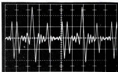
**Levels and slopes.** These two illustrations give you some idea of what Exact's new waveform synthesizer can do. The trace at the left shows a digital waveform constructed with 20 steps, with the instrument in its 20-variable-step-width mode. On the other hand, the right-hand photo shows an analog waveform such as you may need to simulate speech, sonar, transient, or vibration signals. It was built with the instrument in its variable-slope mode, using all 40 segments.
