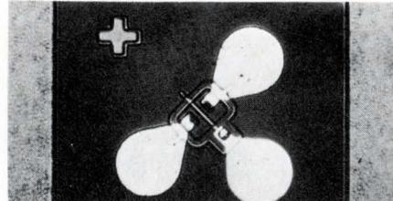
These matched, dual, n-channel FETs also have low differential drift. Types 2N5902 through 2N5905 have an  $I_G$  of 3 pA max.; the 2N5906-09, 1 pA max. The 2N5902 and 2N5906 have 5 mV offset max., with 5  $\mu$ V/ $^{\circ}$ C differential drift. In TO-78 cans, the FETs cost \$7.05 to \$22.50, 100-pc. lots. As chips, CDNT01, \$4.35/pair, 100-pc. lots. Siliconix Inc., 2201 Laurelwood Rd., Santa Clara, Calif. 95054. (408) 246-8000.
