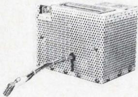
This supply's operation is relatively independent of input voltage, polarity, or frequency. No changes or adjustments are needed for it to function on positive or negative 22 to 32 Vdc; 115 or 230 Vac  $\pm 10\%$  at 50 to 420 Hz. The unit shown provides five independent 1-v outputs (+25, -12, -3.2, -6, and -12 Vdc) each regulated to  $< 1\%$  with 36 W at 95°C with a  $\tau_c$  of  $< 0.007\%$  from -54 to +95°C. Capatron Div., AMP Inc., 155 Park St., Elizabethtown, Pa. 17022. (717) 564-0101.
