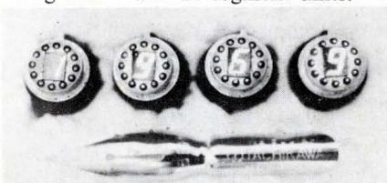
These photodiodes provide bright readouts, fast response to switching, low power consumption and long life. An 8-segment display about the size of a thumbtack can produce figures from zero to nine and a stop sign in bright red. The 16-segment diode can produce the complete alphabet. Large crystals of arsenic phosphate gallium (GaAs P) are used in a monolithic integrated structure. Hitachi, America Ltd., 437 Madison Ave., New York, N.Y. 10022. (212) 758-5420.
