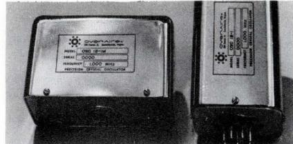
OSC 18 series proportional oven controlled oscillators range in stability from  $1 \times 10^{-9}$ /day through  $1 \times 10^{-8}$ /day. Oscillator and oven together need only 3 W power (12 Vdc or 24 Vdc) in steady state condition, at  $+25^\circ\text{C}$ . Available with  $< 2 \times 10^{-10}$  change in freq./ $^\circ\text{C}$  amb. change. Frequencies from 500 kHz to 30 MHz. Plug-in or PCB mounting. Ovenaire, Inc., Charlottesville, Va. 22902. (703) 293-5148.
