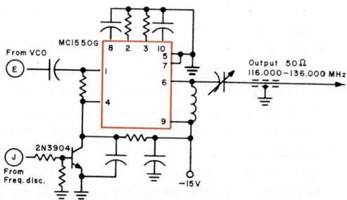
**Fig. 9: Gated amplifier.** This stage serves as a buffer between the output of the synthesizer and the system into which it feeds. It also lowers the output of the synthesizer at least 40 dB when the synthesizer is out of frequency lock. This is done by applying the logical output from the window detector to the 2N3904 transistor, as shown. When this transistor is turned on, it removes the dc bias from the amplifier, which causes the 40 dB reduction in output.
