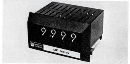
DP400 Series 10,000 count meters are high-accuracy ( $\pm 0.02\%$ ,  $\pm 1$  count) dc voltage measuring devices that provide direct digital readout of the value of the applied input voltage. Three models are available with full-scale input ranges of 1.0, 10.0 or 100.0 V. Range is 30°F to 140°F, and TC is 0.003%/°F. \$273.00 and up. Computer Products, 2709 Dixie Hwy, Box 23849, Ft. Lauderdale, Fla. 33307. (305) 565-9565.
