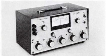
The DC 110C has a 6-digit readout and a guarded 100  $\mu$ V null detector. The voltmeter gives you a recorder output of 0 to 1 V at ½ mA. Also included is a voltage reference source (from 0 to 11 V) that has an accuracy of 0.01% of setting. \$675. Precision Standards Corp., 1701 Reynolds (Irvine Industrial Complex) Santa Ana, Calif. (714) 546-0431.
