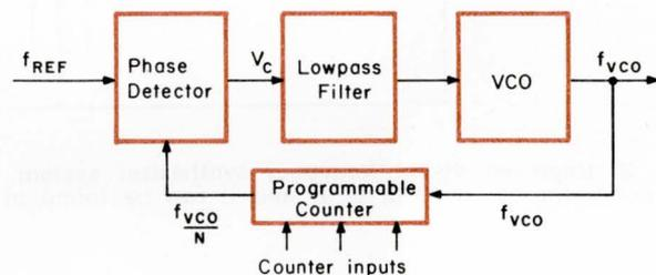
Multiple channel phase-locked loop system.
