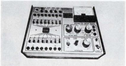
Model 101 performs dc and functional testing of most digital IC's. Panel layout follows typical data sheets for fast programming. Model 101A has a test socket for TO-5s and flat packs as well as 14- and 16-pin DIPs. \$295 (Model 101) and \$315 (101A). Spectrum Dynamics, 2300 E. Oakland Park Blvd., Ft. Lauderdale, Fla. 33306. (305) 566-4467.
