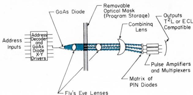
an ROM subroutine, he can generate completely tested masks in-house and ship any number to his customers, without expensive field maintenance, downtime, or re-wiring, which add substantially to the cost of a memory.
