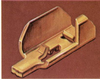
These legs straddle the conductor, and are then rolled 180° to pierce the insulation again. This displacement makes reliable positive contact. Two protruding lances on the under side of the "U" pierce the insulation from the other side. The result is four metal-to-metal-to-metal gastight area contacts in each termination with no deforming effects on the conductor.
