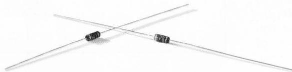
**Performance.** HP's PIN diode offers better cross-modulation and second order distortion performance than FETs or other conventional techniques. Our current-controlled resistors have an effective minority carrier lifetime of  $1.3 \mu\text{s}$  with extremely low distortion over the 1 MHz to 1 GHz range. They also have tight resistance tracking between units, and the RF resistance limits are fully specified.
