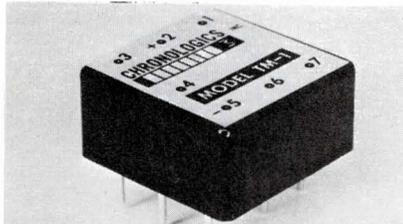
By adding ext. resistors and capacitors to the TM series modules, you can obtain timing ranges from milliseconds to hours. Timing is fixed or adjustable with delay or interval modes of operation. Outputs are pulse, continuous, or complementary. Repeat accuracy is ±1% at constant temp. Series also features on/off voltage level control. Chronologics Inc., 24 Martin St., Webster, N.Y. 14580. (716) 782-1470.
