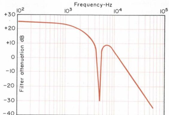
Fig. 5: Loop filter response.
