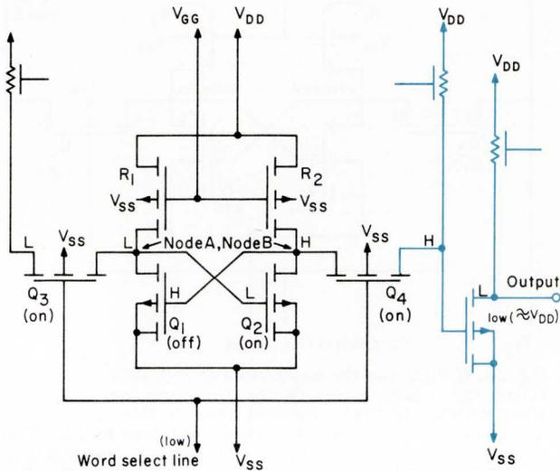
Fig. 3. Reading out of the basic storage cell. The portion of the circuit in color is the simple MOS inverter used as the sense circuit.
