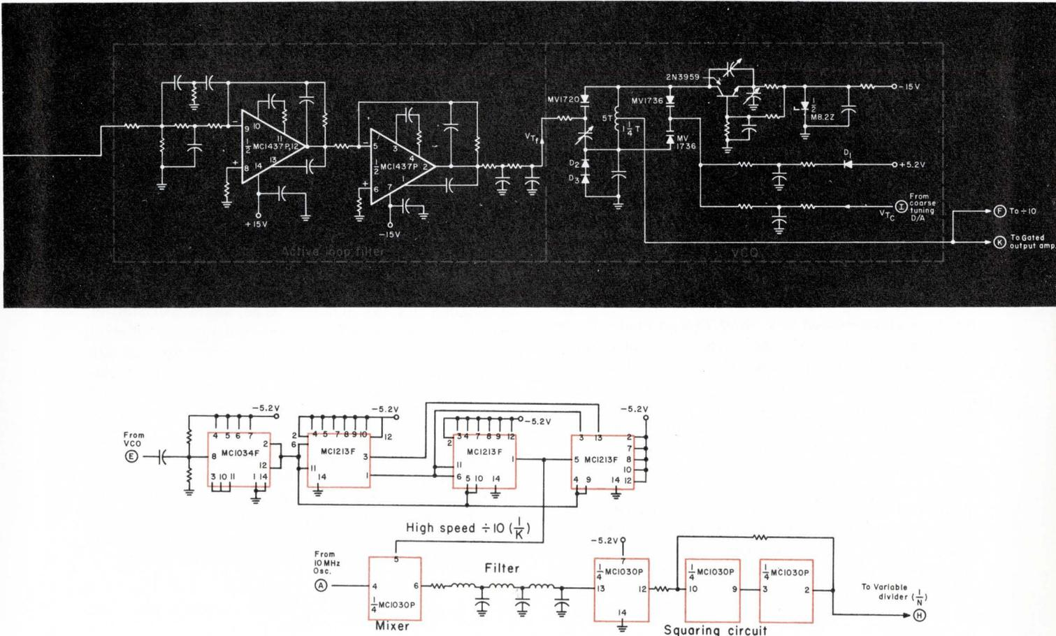
Fig. 6: High-speed divide-by-ten function. Four ceramic flat-pacs were used, with care taken in the layout.
