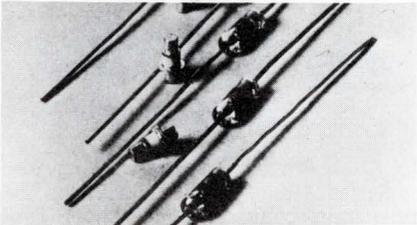
These PIN diodes provide up to 1.0 kW peak power with 5 ns switching time and dynamic Q of 300. Minimum breakdown of 100 V and lifetime of 75 ns are other characteristics. These diodes, characterized at 1 GHz, are for use in fast switches and modulators in waveguide, stripline or coaxial circuits. Microwave Associates, Burlington, Mass. 01803. (617) 272-3000.
