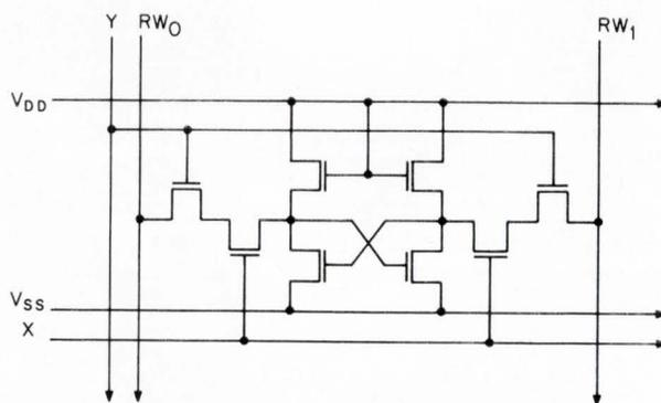
The memory cell for a high speed RAM is a simple cross-coupled flip-flop.
