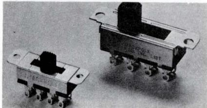
New miniature slide switch is about half the mass of a regular slide switch. Typical overall length is reduced from 1⅜ in. for a std. sized switch to 1 in. for a comparable miniature switch. The multi-purpose switch is available in all combinations from SPST to double pole—three position. Initial ratings are 1 A at 125 Vac (ind. load). Stackpole Components Co., Box 14466, Raleigh, N.C. 27610.
