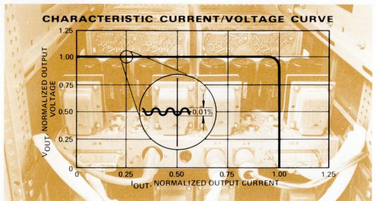
Voltage regulation of 0.01% is standard duty for the MC1566 lab quality regulator.
