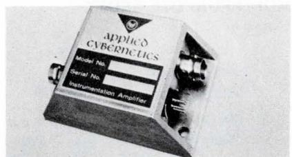
These video preamplifiers are suitable for use in CCTV and CATV as well as high resolution video detection, low light level tv, pulse studies, and general lab use. Features include 1 V pk-pk into 50  $\Omega$ , 50 MHz bandwidth, 0-40 dB gain,  $Z_0$ : 50 or 75  $\Omega$ ,  $Z_i$ : 50  $\Omega$  to 1 kM $\Omega$ , and a rugged aluminum case. AMF Alexandria Div., 1025 N. Royal St., Alexandria, Va. 22314. (703) 548-7221.
