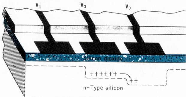
equally divided between the semiconductor and the insulator, there are no holes at the semiconductor-insulator interface. If holes are introduced into the depletion region—by avalanche multiplication, light, or other means—they will collect at the semiconductor interface, causing the interface potential to become more positive.
