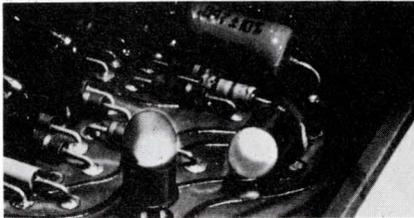
New HP 5082-4403 red light-emitting diode (LED) is designed to displace miniature incandescent and glow lamps in indicator applications. The GaAsP lamp is for self-mounting in panels or PC boards, and has a rugged lead-frame and plastic construction. It has a typ. life of 1,000,000 hrs. Operating on 1.8 V at 20 mA, it is compatible with ics. Hewlett-Packard Co., 1501 Page Mill Rd., Palo Alto, Calif. 94304. (415) 326-7000.
