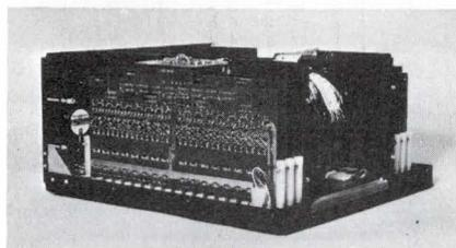
The MSI approach makes use of the inherent fast NDRO properties of plated wire to achieve a 200 ns Read cycle. The EAROM is organized in such a way to make the write function very tolerant of timing, drive current variations, and line recovery, as a tradeoff for high read speed. Even so, it has a 1  $\mu$ s write cycle. Memory Systems, Inc., 3341 W. El Segundo Blvd., Hawthorne, Calif. 90250. (213) 772-4220.
