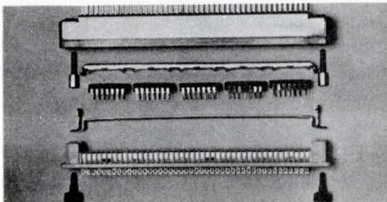
New packaging system, DipStik II, provides high capacitance and low impedance ground and power planes. With it you can mount DILs, remove or replace them and change logic circuitry, all in a few seconds—without the use of solder. Its high density packaging capability allows 1000 DILs to be mounted in a 5¼ in. rack. ACS Industries, 13726 Saticoy St., Van Nuys, Calif. 91402. (213) 988-5310.
