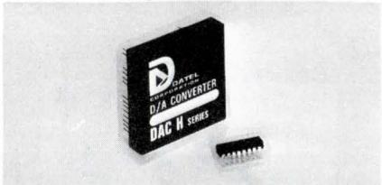
The 25 ns settling time to within 0.1% of the final value in these DAC-II converters allows for an update word rate of 40 MHz. Full scale output is  $\pm 2.5$  mA with a max. voltage compliance of  $\pm 1.2$  V. Output linearity is  $\pm 2.5$   $\mu$ A with a current resolution of 5  $\mu$ A. Overall accuracy is  $\pm 0.005\%$  with a TC of  $\pm 15$  ppm/ $^{\circ}$ C. Total volume is only 1.6 in.<sup>3</sup> Datel Systems Corp., 943 Turnpike St., Canton, Mass. 02021.
