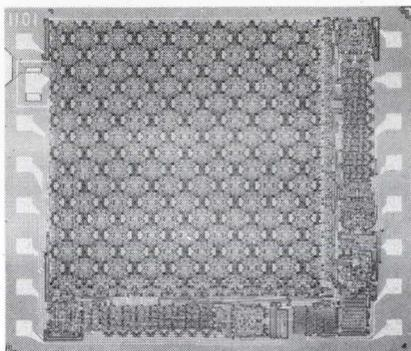
In volume production since August 1969. Intel's Model 1101 is a fully-decoded silicon-gate MOS device with 1.5  $\mu$ sec maximum cycle time. Drives DTL and TTL logic directly. Has OR-Tie capability. Dissipates only 50  $\mu$ W per bit on standby and 2 mW per bit during access. Packaged in 16-lead DIPs. Intel can begin immediate delivery to you in production volume at a price of about 6¢ per bit.
