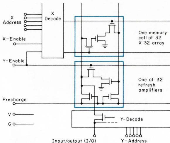
Fig. 4. A dynamic MOS RAM. The chip contains 1024 bits.
