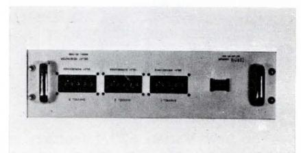
Model 413, gives you three independently delayed output pulses (from 1.0 to 9,999.9  $\mu$ s). You can vary input pulse sensitivity from +10 to +1200 V, and the generator produces a pulse of +100 V into 50 $\Omega$  with a rise time of 100 ns (10-90% points) and with a duration of 100  $\mu$ s. Cordin Co., 2230 So. 3270 W, Salt Lake City, Utah 84119.
