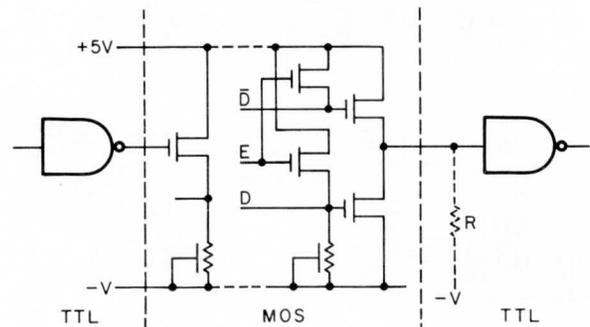
Fig. 3. Interfaces between low-threshold MOS circuitry and TTL or DTL logic.
