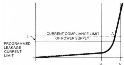
**Breakdown voltage testing**
