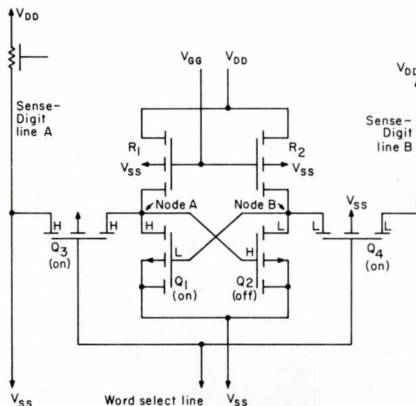
**Fig. 2a.** Writing into the basic storage cell. When the word-select line is low,  $Q_3$  and  $Q_4$  are turned on and  $Q_1$  and  $Q_2$  are connected to the sense-digit lines. In this case, line A is high (close to  $V_{SS}$ ) and line B is low (close to  $V_{DD}$ ). The result is  $Q_1$  is biased on and  $Q_2$  biased off. The H and L designations indicate whether a point is close to  $V_{SS}$  (H) or  $V_{DD}$  (L).
