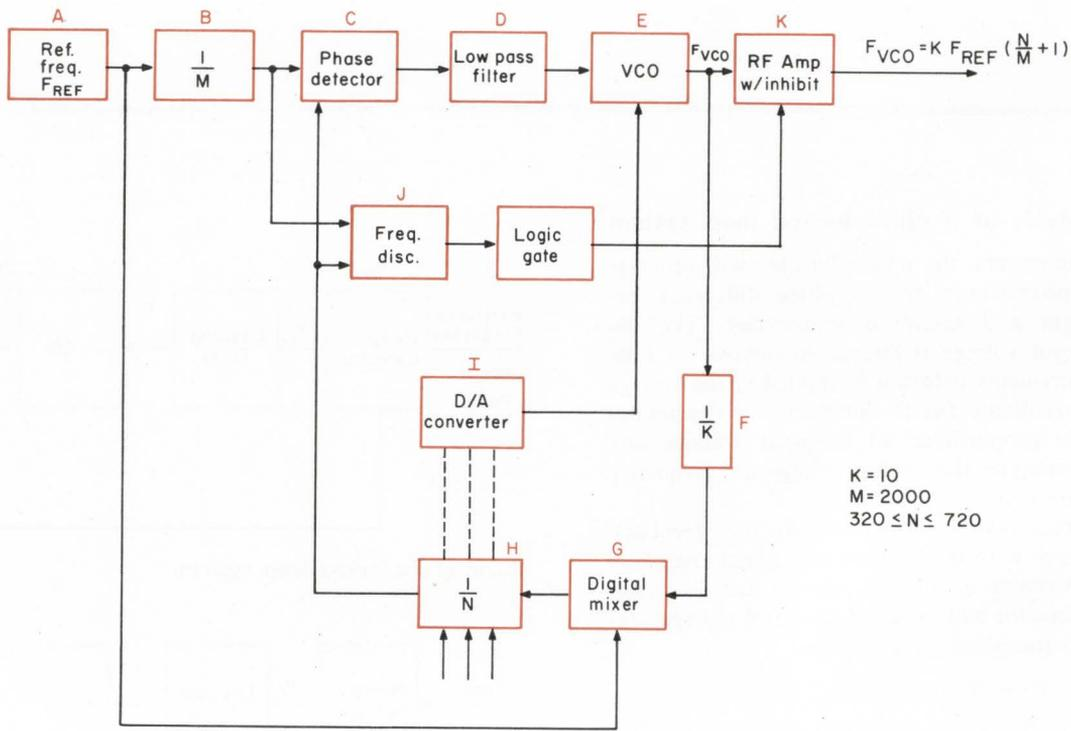
Fig. 2: Improved digital frequency synthesizer system. Circuitry for boxes A, B, C, D and E can be found in
