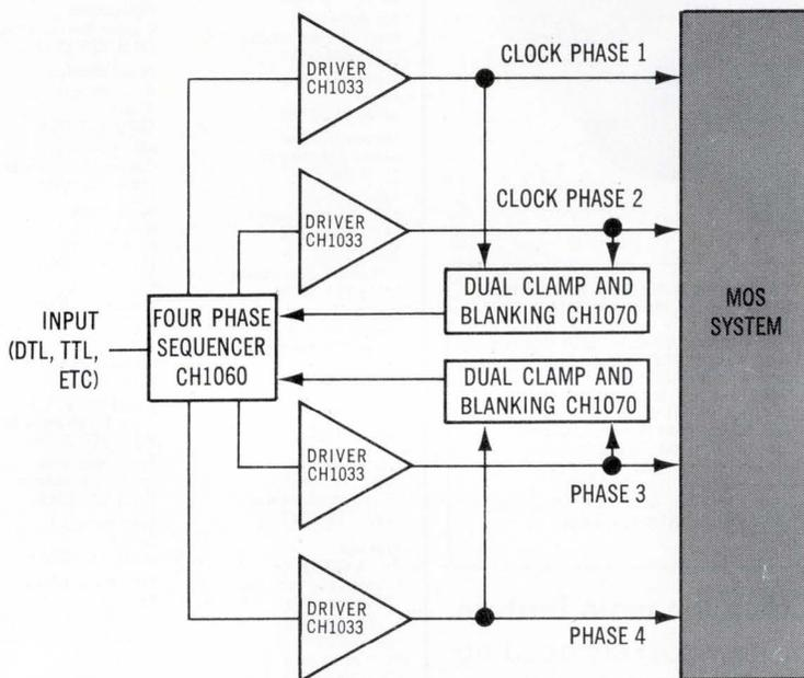
The four phase system shown uses a CH1060 FOUR PHASE SEQUENCER, four CH1033 HIGH SPEED CLOCK DRIVERS and two CH1070 DUAL CLAMP AND BLANKING CIRCUITS.
