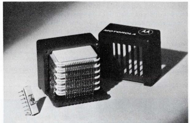
Fig. 6. This random-access memory module stores 8192 bits with an access time of 150 ns. The module combines the high packing density of MOS arrays for the storage function with bipolar read and write circuitry.
