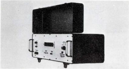
Model DLT-1 accepts start/stop signals and measures the time interval between them logarithmically. The basic unit reads in 0.1 dB steps up to a max. reading of 60 dB, with the reference (0 dB interval) selected as 10  $\mu$ s, 100  $\mu$ s, 1 ms, 10 ms, 100 ms, or 1s. Microwave/Systems, 1 Adler Dr., East Syracuse, N.Y. 13057.
