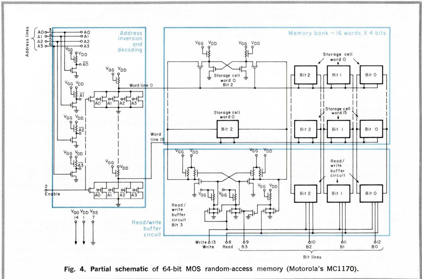
Fig. 4. Partial schematic of 64-bit MOS random-access memory (Motorola's MC1170).
