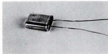
New, series resonance AT precision cut crystal is available in small HC-18/U-or HC-25/U holders. The fundamental mode crystal holds tolerances as low as  $\pm 0.003\%$  over a range of  $-55$  through  $105^{\circ}\text{C}$ .  $R_s$  max. varies from 500  $\Omega$  at 2.0 MHz to 75  $\Omega$  at 4.0 MHz. Drive level is 1 mW with a  $C_0$  of 4.0 pF. McCoy Electronics Co., a subsidiary of Oak Electro/Netics Corp., Mt. Holly Springs, Pa. 17065.
