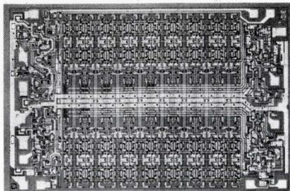
Intel's Model 3101 has been in volume production since September 1969. It's a fully-decoded Schottky-process bipolar RAM with fast 60 ns maximum access. Compatible with DTL and TTL logic. Has OR-Tie capability. Dissipates 6 mW per bit. Packaged in 16-lead DIPs. Immediate delivery in production volume at a price of about 25¢ per bit.
