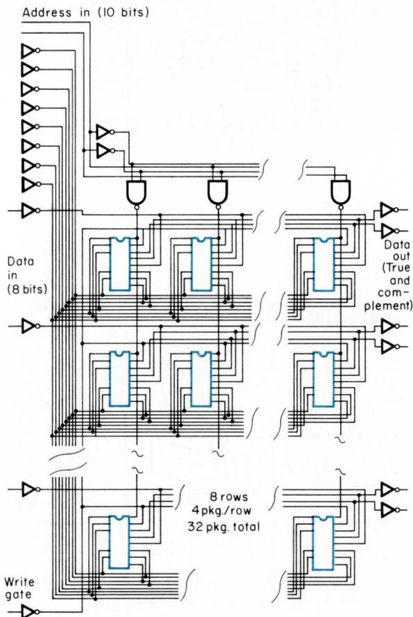
Fig. 5. A 4096 word, 12-bit/word memory using the 1024-bit dynamic MOS RAMs.
