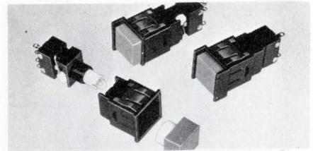
Snap-in housing of the 01-600 series switches is available in bezel, single barrier or double barrier design. Indicator, momentary and alternate action units are available, also 1 or 2-pole switch packages using the 10 A Butterfly<sup>®</sup> double break switch mechanism. Lamp does not move during switch operation. Licon Div., Illinois Tool Works Inc., 6615 W. Irving Park Rd., Chicago, Ill. 60645. (312) AV 2-4040.
