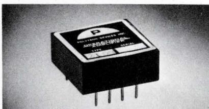
These op amps, Series 210, feature an input impedance of  $10^{12}\Omega$ , and voltage drifts from 2  $\mu$ V/ $^{\circ}$ C. They are especially useful in instrumentation where the recording device (galvanometer) requires dc stability and a high current drive or in applications as a power buffer. Polytron Devices, Inc., 844 E. 25th St., Paterson, N.J. 07513. (201) 523-5000.
