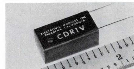
Constant current regulator provides current reg. of 1% over wide ranges of input voltage and temp. A two terminal regulator, it can be used in series with the current line and needs no ref. to ground. TC is 0.03%/ $^{\circ}\text{C}$ . Current stab. with voltage 1%. Maximum power diss. ranges from 1 to 3 W at  $25^{\circ}\text{C}$  case. Electronic Modules Inc., 2560 East Foothill Blvd., Pasadena, Calif. 91107
