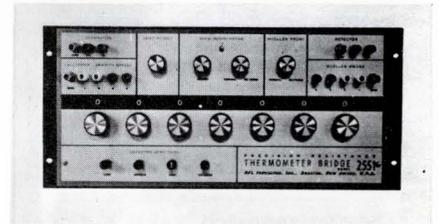
This instrument, Model 2551, can measure temperature or temperature difference (with resistance thermometer probes) to within  $\pm 0.005\%$   $\pm 0.0015\Omega$ . Potentiometers on the bridge panel give you ratio equality and residual resistance balance to within 0.0001 $\Omega$ . Price is \$1400 with delivery 30 to 60 days. RFL Industries, Inc., Boonton, N.J. 07005.
