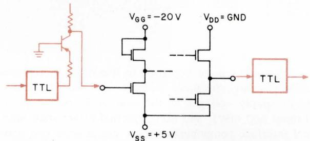
With  $V_{SS}$  equal to +5 V, a high threshold MOS RAM chip can drive TTL directly. However, the input does require level shifters.
