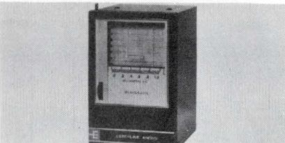
The Minigraph recorder offers a choice of 14 chart speeds ranging from 1/8 in. to 60 in./h. Accuracy is  $\pm 2\%$  and full scale response is 1 s. Sensitivity is 10  $\mu$ A full scale. The Minigraph has four basic movements—from 0 to 10  $\mu$ A, 50  $\mu$ A, 100  $\mu$ A and 1 mA. The six dc ranges range from 1 to 500 V. The ac ranges are 150, 300 or 600 V. \$99.50 and up. Esterline Angus, div. of Esterline Corp., Box 24000, Indianapolis, Ind. 46224.
