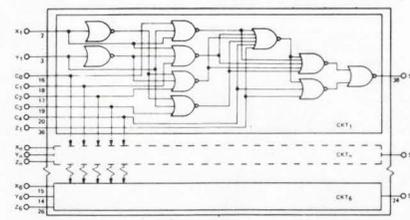
This family consists of the EA 1800 universal logic array, EA 1801 control array, EA 1802 register array and EA 1803 carry array. Features include power dissipations ranging from 180 to 200 mW/package and typical propagation delays of 150 to 500 ns. Electronic Arrays, Inc., 501 Ellis St., Mountain View, Calif. 94040. (415) 964-4321.
