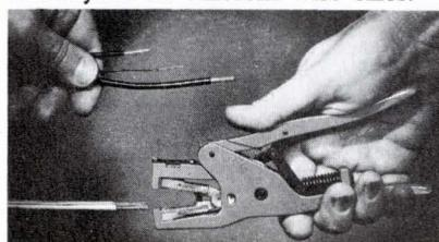
This new tool (ABMK-1) is completely self-adjusting to the point where it is not necessary to know the wire size. Different diameter wires can be stripped consecutively without changing or adjusting the stripping jaws. The tool takes wire dia. from AWG #30 through #12, both copper and aluminum. \$28.00. The Thomas & Betts Co., 36 Butler St., Elizabeth, N.J. 07207. (201) 354-4321.
