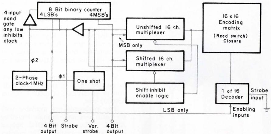
**Keyboard encoding is based on this circuitry.** The binary counter operates continuously. Any Low input to the 4 input NAND gate feeding it (other than the clock input) will inhibit the clock and effectively stop the counter at a particular 8-bit code.
