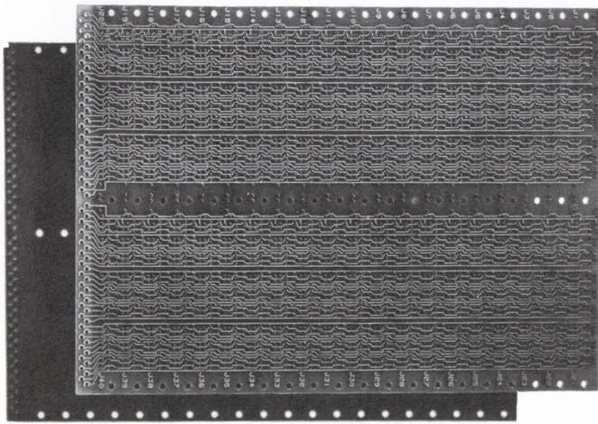
High-density circuit board, made with the NT-1 process.
