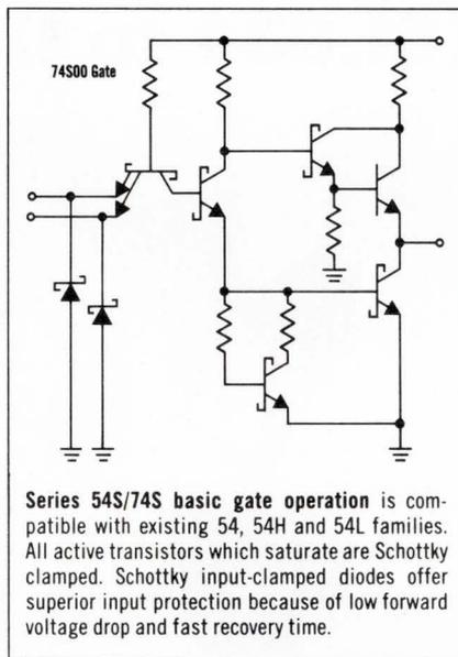
Series 54S/74S basic gate operation is compatible with existing 54, 54H and 54L families. All active transistors which saturate are Schottky clamped. Schottky input-clamped diodes offer superior input protection because of low forward voltage drop and fast recovery time.
