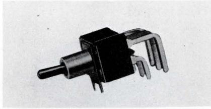
Series 7200A switch, when mounted in vertically stacked pc panels, protrudes outward, making the toggle easily accessible. The 7200A measures only 1.250  $\pm$  0.015 in. from end-of-toggle to end-of-deepest-pole (absolute length). Contacts are made on the opposite side to which the toggle is thrown. C&K Components, Inc., 103 Morse St., Watertown, Mass. 02172. (617) 926-0800.
