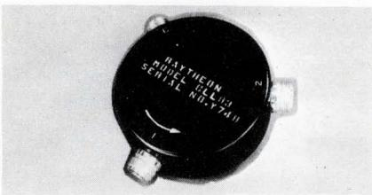
Three-port L-band, Model CLL 83 operates in freq. range of 1200-1400 MHz, with a max. input vswr of 1:20. Maximum insertion loss is 0.3 dB, and min. isolation is 20 dB over the band. It is  $3\frac{1}{8}$  in. in dia. and 1-5/32 in. long, excluding connectors. It comes in either Y- or T-configurations. Raytheon Co., 190 Willow St., Waltham, Mass. 02154.
