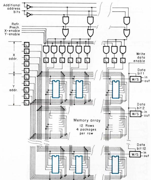
Fig. 2. Using 256-bit static MOS chips to construct a 1024-Byte (1024 x 8) memory.
