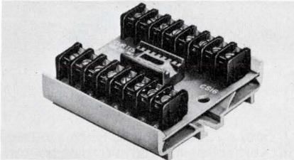
New CS16 assemblies are for testing, breadboarding and packaging 16-pin DIL modules. They feature a PC design, a 16-pin DIL socket, and SE Series barrier terminal blocks. Up to 21 sockets can be mounted to a 48 in. length of prepunched track. \$2.85/assembly, including track, in lots of 1000. Curtis Development & Mfg. Co., 3250 N. 33rd St., Milwaukee, Wis. 53216.
