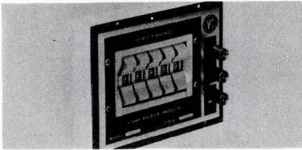
These resistance decades are very accurate ( $\pm 0.005\%$  at the terminals) with a long-term stability up to 5 ppm/yr. They can be used at incoming inspection stations, in the stds. lab. and for component evaluation.
