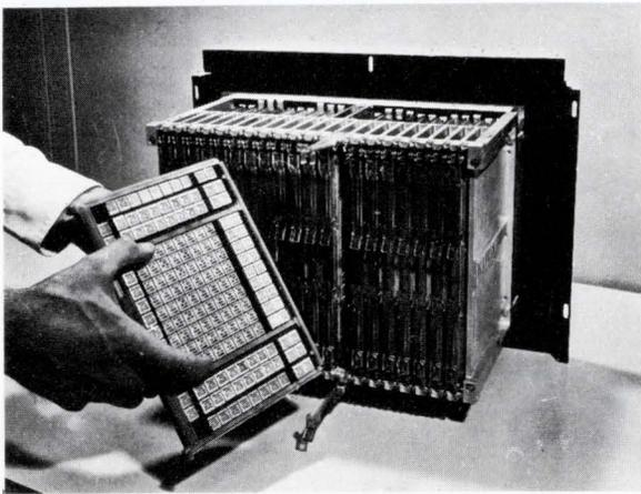
This bipolar IC memory is used as a buffer memory in the IBM 360/85 and 360/195. The memory chips store 64 bits each and have a read time of 7 ns and a write time of 12 ns. The complete memory stores 2048 words of 72 bits each—a total of 147,456 bits—and has an access time of 40 ns. (Courtesy of IBM Corp., Essex Junction, Vt.)
