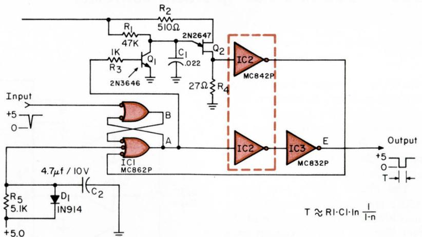
on  $Q_1$  and shuts off the oscillator causing  $V_E$  to become high again. Thus, the output pulse width is determined by  $T$  and is free of the effects of erroneous trigger noise.
