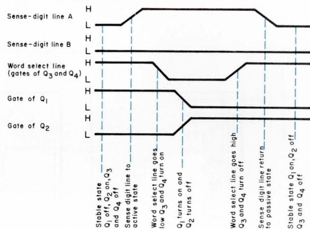
**Fig. 2b.** Timing diagram for the write operation of Fig. 2a.
