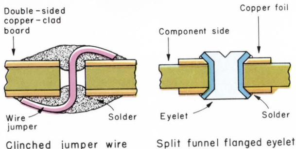
**Mechanical interconnections for doubled sided boards.** Although largely superseded by plated-through holes, these methods are still used for prototype boards and in some military applications.
