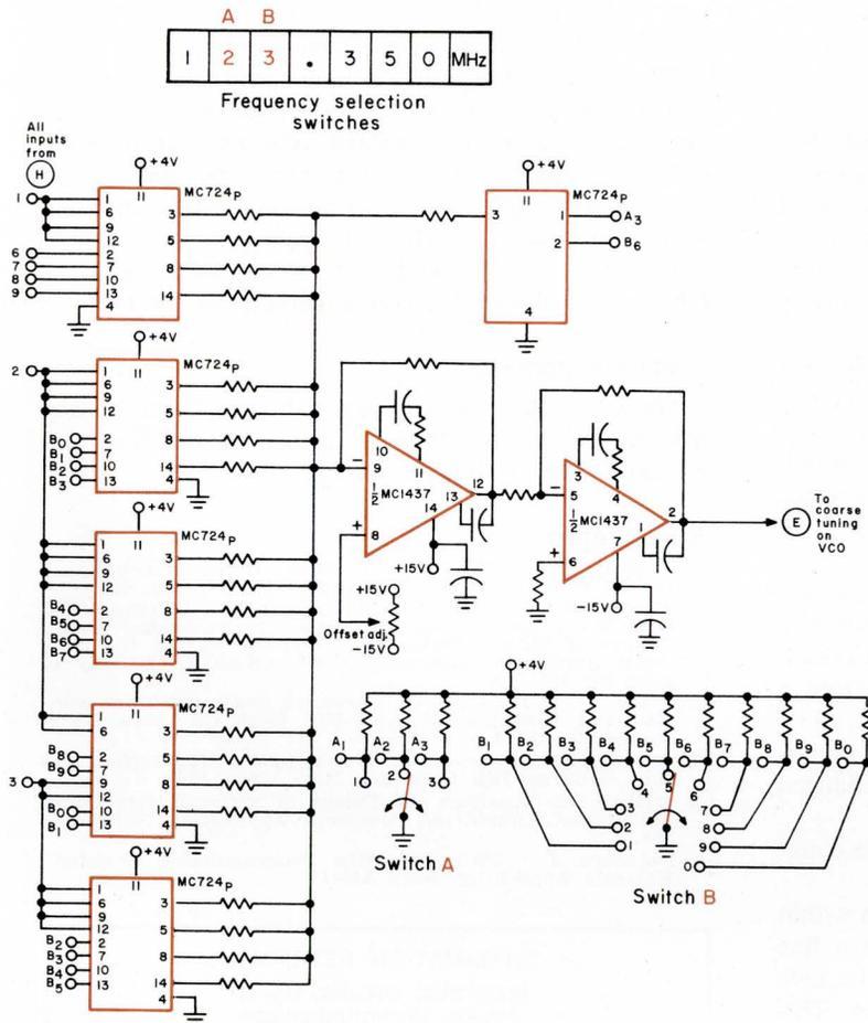
**Fig. 7: D/A converter** is a weighted resistor configuration. The input is obtained from the selector switches that program the variable counter.
