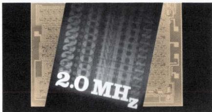
With features like these, the two registers are ideal used for delay lines or circulating data storage. And their dc operation holds your data without needing constant refreshment.
