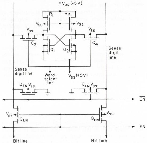
Fig. 8. The storage cell used in the 8-k memory module.
