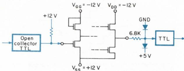
By connecting  $V_{SS}$  to +12 or +15 V, you can use an open collector TTL to drive the high threshold MOS RAM. The resistor and diodes on the output protect the TTL from overdrive.
