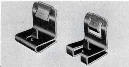
Eight variations of this Speed Clip® fastener accommodate the full range of hardware uses in PCB rack applications. The clips snap to the board rack flanges without tools. Tabs on the clips engage mounting holes in the flanges, and, once installed, the clips remain in place if the connectors must later be removed. Tinnerman Products, Inc., Box 6688, Cleveland, Ohio 44101.
