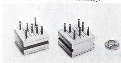
Miniature 10 x 10 solderless boards, grooved for lock-in assembly, provide any number of groupings consisting of 100 terminal holes on 0.100 in. centers. Each "Miniboard" module is 0.147 in.<sup>2</sup> and 27/32 in. thick. Units mount on aluminum framing rails. Contact rating is 3 A. Voltage rating is 300 Vdc max. Programming Devices Div., Selectro Corp., 225 Hoyt St., Mamaronck, N.Y. 10543.
