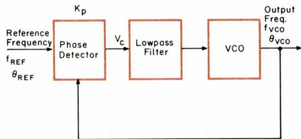
Basic phase-locked loop system.
