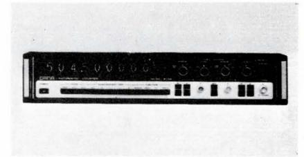
Model 8134 is an 8-digit counter that measures frequencies to 500 MHz (with 500  $\mu$ V sensitivity) and time intervals with 100 ns resolution. All front panel controls can be programmed with TTL-compatible BCD codes. Dana Laboratories, Inc., High Frequency Div., 2401 Campus Dr., Irvine, Calif. 92664. (714) 833-1234.
