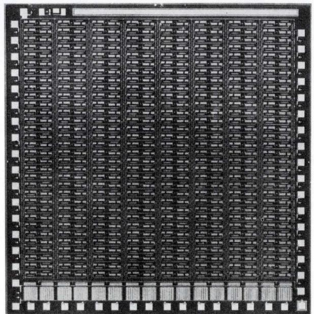
Fig. 7. This 256-bit MOS storage array is one of 32 such chips used in the 8192-bit module.
