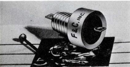
Series 800 units filter ac and dc lines in aircraft, aerospace and industrial avionic systems, power supplies, communication, navigation and guidance equipment. Models are available with ratings from 50 Vdc to 120 Vac, 400 Hz., and from 40 mA to 15 A. A typ. 50 Vdc, 40 mA unit would display an insertion loss of over 80 dB at 1 MHz. About \$12 ea. Filters & Capacitors, Inc., 425 N. Fox St., Box 1272, San Fernando, Calif. 91341.
