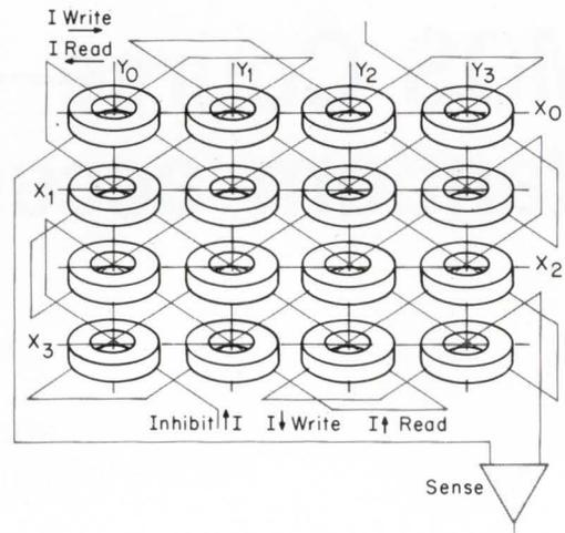
**One plane of a 3-D organized random access core memory.** Each core in this plane stores the same bit for each word in the memory. This plane is repeated for each bit in a word so that the number of planes equals the word length.
