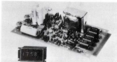
Model 281 is a self-contained converter that operates on 115 Vac. Basic input sens. is 199.9 mV with conversion made at 0.1% of signal  $\pm 1$  digit. Model 282 Numeric Display is usable with the 281 where visual readout is needed. It displays 3 full digits, decimal point, overrange and error indicators. United Systems Corp., 918 Woodley Rd., Dayton, Ohio 45403.
