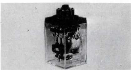
RGP series plug-in type is available in SPDT, DPDT, TPDT with coil voltages of 6 to 230 V. The RGO is the open type. Both series have contact ratings of 10 A resistive with silver cadmium oxide contacts for a min. of 1 million operations at rated load. RMC series min. relay is for PCB mounting. It comes with SPDT, 3 A contacts and coil voltages from 6 to 48 Vdc. Syracuse Electronics Corp., Box 566, Syracuse, N.Y. 13201. (305) 488-4911.
