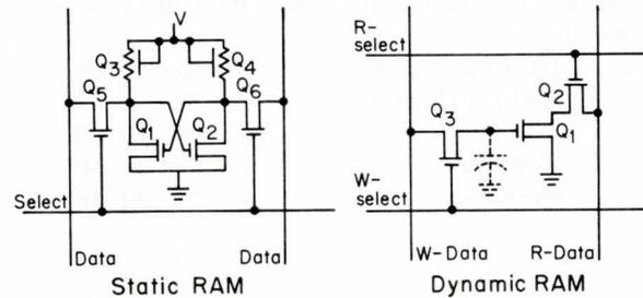
Fig. 1. Storage cells used in MOS RAMs.
