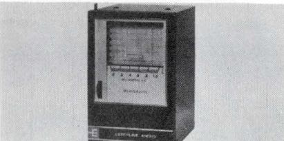
The Minigraph recorder offers a choice of 14 chart speeds ranging from  $\frac{1}{8}$  in. to 60 in./h. Accuracy is  $\pm 2\%$  and full scale response is 1 s. Sensitivity is 10  $\mu$ A full scale. The Minigraph has four basic movements—from 0 to 10  $\mu$ A, 50  $\mu$ A, 100  $\mu$ A and 1 mA. The six dc ranges range from 1 to 500 V. The ac ranges are 150, 300 or 600 V. \$99.50 and up. Esterline Angus, div. of Esterline Corp., Box 24000, Indianapolis, Ind. 46224.
