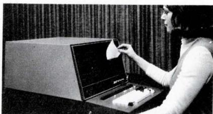
Fast, high quality hard copy output for CRT terminals is available as an integral feature of the '45' desk-top CRT Data Terminal. The electro-optical printout process produces a 5 x 5 in. photoprint of the data displayed on the CRT in  $< 7$  s after pressing the print button, with additional copies at 2 s intervals. \$15,000. Photophysics Data Systems, 1255 Terra Bella Ave., Mountain View, Calif. 94040.
