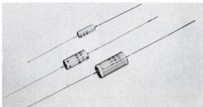
A positive hermetic glass-to-metal seal on this wet anode tantalum electrolytic capacitor prevents electrolyte leakage. The new TLW capacitor has voltage ratings of from 6 to 125 V and a capacitance of 560  $\mu$ F at 6 V to 25  $\mu$ F at 125 V. P.R. Mallory & Co. Inc., 3029 E. Washington St., Indianapolis, Ind. 46206. (317) 636-5353.
