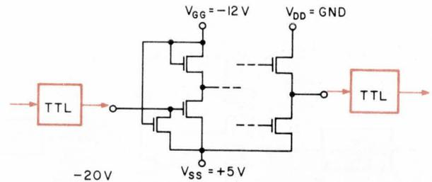
Chip interface for a memory with full decode and low threshold voltage.
