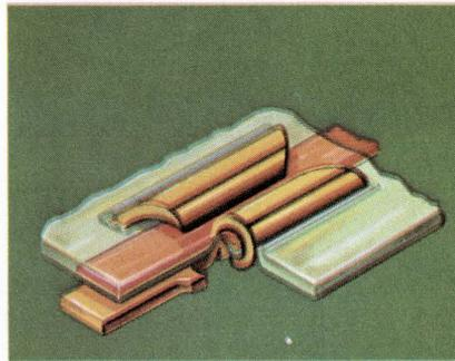
**Up to 3,400 terminations an hour.** Honest. With a 29 position cable you can really get 3,400 finished terminations an hour. With a 19 position cable you get 2,700. Absolutely no cable preparations — just cut and terminate. It's all done automatically with our precision engineered machine that you can use in your own plant.
