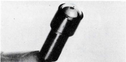
Connected to key circuit elements, these microminiature fault isolation indicators respond to a fault signal—transient or continuous—by a color transfer of its display mode. The display latches into place magnetically until reset. Reset is accomplished by momentarily energizing a reset coil. They are for pulse operation and do not require continuous power. The A. W. Haydon Co., 232 N. Elm St., Waterbury, Conn. 06720.
