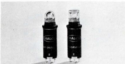
This subminiature transistorized light, specially designed for ICs, needs no power supply and interface circuitry. It operates directly from std. TTL, DTL, and RTL micrologic modules. Signal level requirements and power supply voltage for these units are completely compatible with ICs. All driving circuitry is within the indicator light itself. Dialight Corp., 60 Stewart Ave., Brooklyn, N.Y. 11237. (212) 477-7600
