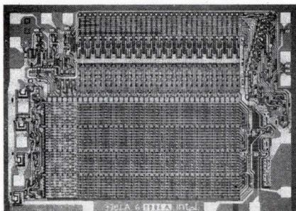
Intel's Model 3301 has been in volume production since December 1969. It's a Schottky-process bipolar ROM with 60 ns maximum access. Supplied in 16-lead DIPs that combine to form memories storing 1024 words of any length. Intel can deliver custom 3301's to match your truth table in 4 to 6 weeks at a price of about 2¢ per bit in production quantities.
