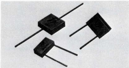
These capacitors come in eight different series which include 22 styles. Available in a range of 0.24 pF through 10,000 pF, they have tolerances of either  $\pm 0.1$  pF or  $\pm 1\%$ . All styles have failure rates of  $< 0.15\%$ /1000 h at a 90% confidence level at rated temp. and voltage conditions. Vitramon, Inc., Box 544, Bridgeport, Conn. 06601. (203) 268-6261.
