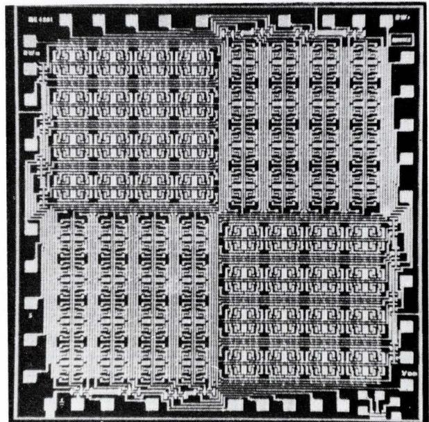
Microphotograph of a high-speed RAM.
