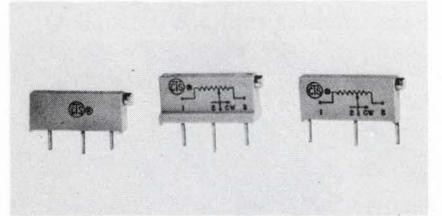
Series 190  $\frac{3}{4}$  inch rectilinear 20-turn units come in three types: Type 190, 0.100 in. wide and 0.500 in. length pin spacing; Type 191, 0.200 and 0.500 in., and Type 192, 0.100 and 0.700 in. All have low  $\pm 150$  ppm/ $^{\circ}\text{C}$   $\tau_c$  for most values,  $\frac{1}{2}$  W rating at  $85^{\circ}\text{C}$  and clutch stops. Standard range is from 50  $\Omega$  to 500 k $\Omega$ . Under \$1.00 (in quan.). CTS of Berne, Ind. 46711. (219) 589-3111.
