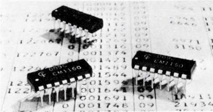
The CM1150 dual transmitter and CM1160 dual receiver meet EIA RS232B/C and Mil-STD-188B specifications. The  $\pm 1.25$  V noise margin at the inputs of the CM1160 receiver is the highest currently available. Price for both devices is \$8.45 ea. in 100 pc. quantities. Cermetek, Inc., 660 National Ave., Mountain View, Calif. 94040. (415) 969-9433.
