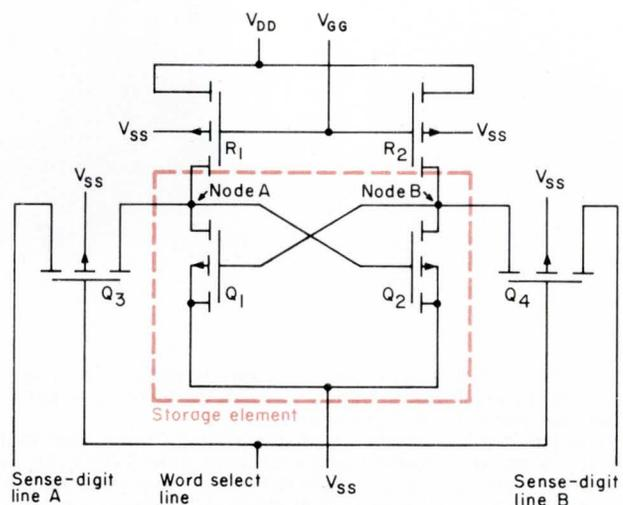
Fig. 1. The basic MOS storage cell. The two p-channel transistors, identified as  $R_1$  and  $R_2$ , are biased on by  $V_{DD}$  and act as resistors. The cross-coupled combination of  $Q_1$  and  $Q_2$  forms the actual storage element and  $Q_3$  and  $Q_4$  act as switches to connect or isolate the individual cell and the sense-digit lines.
