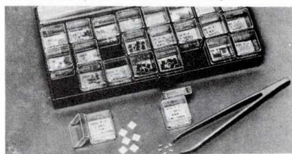
AlSiMag® kit contains both single layer and multi-layer capacitors. Diced chip capacitors range from 18 pF to 1500 pF in sizes from 0.020 in.<sup>2</sup> to 0.350 in.<sup>2</sup> Multi-Cap® capacitors range from 10 pF to 0.085 µF in sizes from 0.085 x 0.055 in. to 0.220 x 0.250 in. Materials range from TC to high K. Tolerances are ±5%, ±10% and ±20%. \$50. American Lava Corp., Chattanooga, Tenn. 37405. (615) 265-3411.
