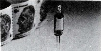
The A297 lamp is made with 7mm electrodes enclosed in a glass envelope which is much longer than necessary for an ordinary neon lamp. The long envelope with shorter electrodes eliminates the possibility of a change in characteristics of the device due to sputtering. Breakdown rating is 215 V max. and a maintaining voltage 128 to 148 V. Design current is 5 mA. Signa-lite Inc., 1933 Heck Ave., Neptune, N.J. 07753. (201) 775-2490.
