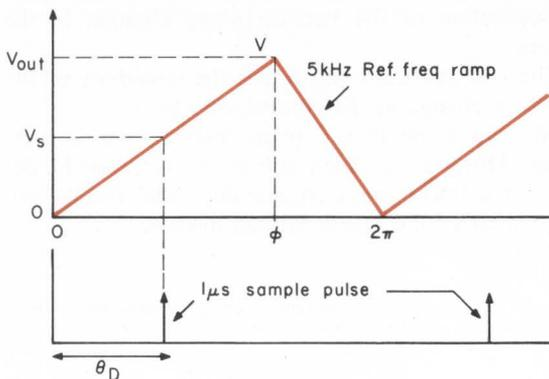
Fig. 4: Sampling timing diagram.
