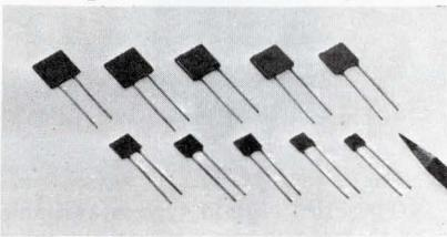
Lead spacings of these single-film silvered mica capacitors are interchangeable with those of normal ceramic disc capacitors. Thus you can have the advantages of silvered mica dielectric without having to completely revise PC boards. Type 91M capacitors come in 45 ratings ranging from 10 pF to 68 pF at 500 V. Sprague Electric Co., 233 Marshall St., North Adams, Mass. 01247.
