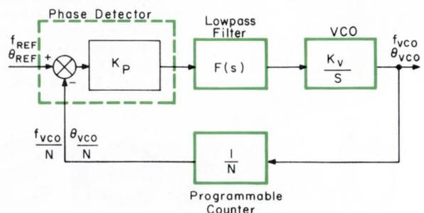
Fig. 1: Linearized phase-locked loop model.
