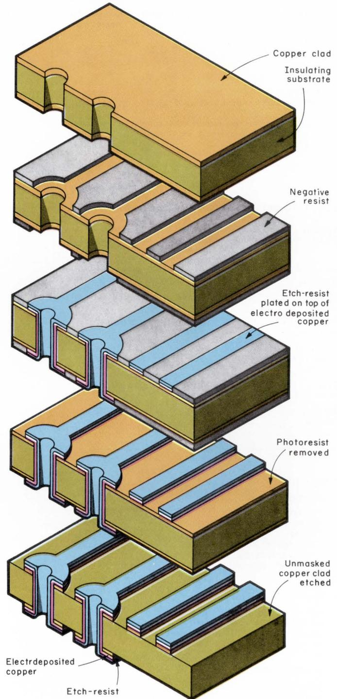
**Conventional plating of holes, for a double-sided board,** starts by sensitizing the holes of a punched board with a chemical that provides a base for copper. The second step applies resist to those areas where copper will not go. Electrodeposited copper adheres to the holes' walls and is built up to about 1 mil. Both the resist and the unwanted copper are then removed.
