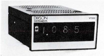
Features of the VT 300 include automatic zero, overrange indicator, internal calibration voltage, BCD output, end of measurement signal output, and an external trigger input. Accuracy is  $\pm 0.1\%$  of reading,  $\pm 0.1\%$  of full scale. \$199 with delivery from stock. Dixon, Inc., Box 1449, Dept. 227, Grand Junction, Colo. 81501. (303) 242-8863.
