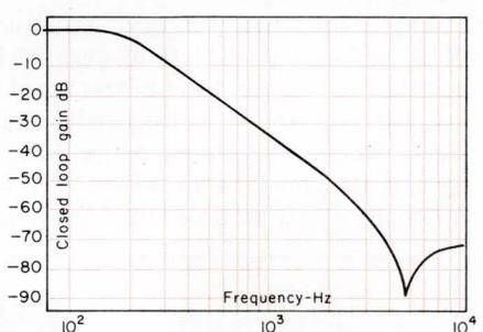
**Fig. 10: Actual measured closed loop response.** The measured damping coefficient of 0.55 indicates that very little overshoot is present, giving rise to a stable system with excellent transient response. Lock-up time is about 2 ms.
