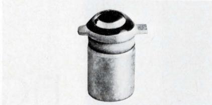
New silicon planar Darlington light sensor is suitable for use where the available light is below normal industry stds. At irradiance of 1 mW/cm<sup>2</sup>, the Type OP 300 phototransistors will generate light currents of over 10 mA. Peak spectral response is between 0.80 and 1.0  $\mu$ m. Maximum power diss., 50 mW. \$3.95 ea. (1-99); \$2.65 ea. (100-999). Optron, Inc., 1201 Tappan Circle, Carrollton, Tex. 75006. (214) 242-6571.
