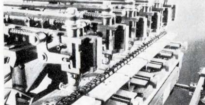
Multi-spindle engraving machine has solved the problem of how to permanently mark concave typewriter keys with up to 3 lines of identification. The machine is operated pneumatically on the tracer-guided principle. An operator without any previous experience can engrave 36 keys with one setup. New Hermes Engraving Machine Corp., 20 Cooper Sq. New York, N.Y. 10003. Booth IB12.
