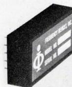
Series 100 filters are unity-gain and non-inverting. Standard models have 2—6 pole—low pass, high pass, band-pass or band reject—Butterworth, Bessel, Tchebyscheff or Twin-T transfer functions. Specs include  $\pm 0.02$  dB passband gain tol.,  $\pm 5\%$  cutoff freq. accuracy, 100 k $\Omega$  typ. input imp. 10  $\Omega$  output imp. and adj. volt. offset. Frequency Devices, Inc., 25 Locust St., Haverhill, Mass. 01830. (617) 372-6930.
