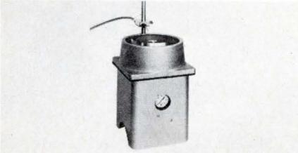
Model SC45 cleans silicon wafers prior to the deposition of epitaxial layers or diffusion processes. The unit uses a high energy "scrubbing" action while the surface is rinsed and cooled by a clean pure fluid. Process cycle time is 10-15 s and the wafers are ready for immediate processing. Headway Research, Inc., 3713 Garland, Tex. 75040. (214) 272-1566.
