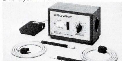
Model 150 autospulse soldering system features two newly developed micro point hand soldering probes. The power supply has a continuous range from 0 to 60 W of instant pulse heating energy. Plug-in hand probes feature soldering tips as small as 0.010 in. in dia. \$175.00. Browne Engineering Co., 1120 Coast Village Circle, Santa Barbara, Calif. 93103. (805) 969-2268.
