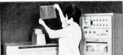
Slo-Syn Photo Artwork Generator eliminates manual drafting and photo reduction of PCB artwork. Working from a grid paper sketch, the tape can be programmed manually, by a digitizer or by computer. It produces, on film, an accurate circuit pattern to finished board size without the need for photo reduction. The Superior Electric Co., Bristol, Conn. 06010. (203) 582-9561. Booths 3B03-3B07.
