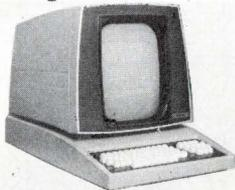
As a communications terminal, the PDS-1 system can replace any on-line, electromechanical device without modifying the central system nor the present communications facilities. It can function from 1 to 9600 baud using any bit structure or code level. PDS-1 is also a mini-processor. Imlac Corp., 296 Newton St., Waltham, Mass. 02154. (617) 891-1600.
