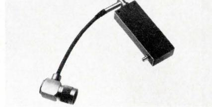
Model 2424-1 low pass filter passes the 200-400 MHz communications band with < 0.3 dB loss and rejects 520-1500 MHz, 60 dB. Power capability is 50 W average. The 3 3/8 x 1 1/4 x 3/4 in. filter mounts one SM connector (Microdot #51-258) and one type N elbow. \$150.00. Microwave Filter Co., Inc., 135 W. Manlius St., East Syracuse, N.Y. 13057. (315) 437-4529.
