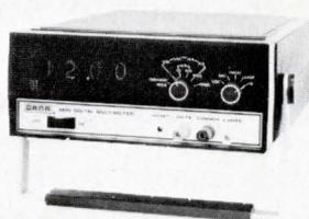
Model 3800 has full multimeter capability; 5 dc, 4 ac, 6  $\Omega$ , and 6 dc current ranges, and BCD output as an option, and sells for \$425. Model 3860 provides dc and ohms measurement capability for \$350. Both instruments have a dc accuracy of 0.1% of measured reading. Dana Laboratories, Inc., 2401 Campus Dr., Irvine, Calif. 92664. (714) 833-1234. Booths 2H39-2H47.
