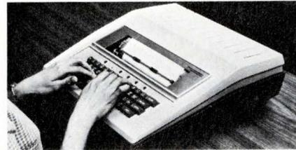
Series 720 terminals are compatible with KSR (keyboard send-receive) 33 to 35 teletypewriters. They are offered in USASCII and BCD codes and in keyboard and receive-only models. The new data terminal models (15, 20, 21, 22, 30 and 31) are almost silent at speeds up to 40 char./s. All models use a 5 x 7 matrix pattern. Texas Instruments Incorporated, Box 66027, Houston, Tex. 77006. (713) 526-1411.
