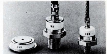
Series 101KL40S20 and 101KLR-40S20 units meet the need for fast recovery diodes occupying a position between devices now available at 35 and 250 A. They are available with reverse recovery times of 1.5  $\mu$ s and 2.0  $\mu$ s with up to 100 A at from 400 to 1300 V. Applications include inverters, SCR assemblies and other areas requiring hf fast recovery rectification. \$25 ea. (1 to 9). International Rectifier, Semiconductor Div., 233 Kansas St., El Segundo, Calif. 90245. (213) 678-6281.
