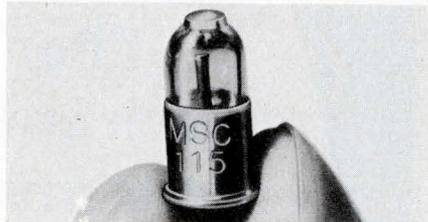
The MSC 115 Vac lamp operates at 105-125 Vac or 150 Vdc, providing high intensity brightness adequate for most applications of midget lamps. Lamps with built-in current limiting resistors are available in three types featuring average life of 1500, 10,000 and 25,000 hrs. They meet all applicable requirements of Mil-E-5272. Master Specialties Co., 1640 Monrovia, Costa Mesa, Calif. 92627. (714) 642-2427.
