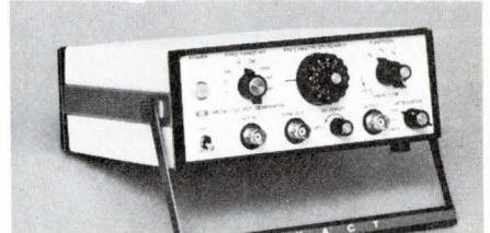
This unit has voltage controlled frequency over a 1000:1 ratio. The Model 123 gives you sine, square and triangle waveforms, and a sync pulse. Frequency is  $\pm 2\%$  accurate and the external voltage control can either be dc programming or ac frequency modulation. \$345. Delivery, stock to 30 days. Exact Electronics Inc., Box 160, Hillsboro, Ore. 97123. (503) 648-6661.
