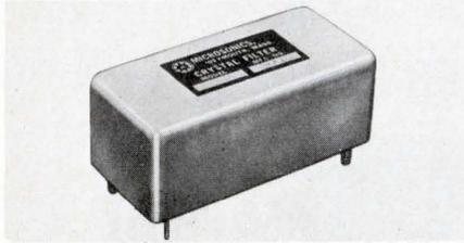
Model SB56A filter has a carrier freq. of 5.0 MHz with 3 dB high and low bandwidth of  $\pm 3.5$  kHz and  $\pm 300$  Hz respectively. Carrier rejection is 20 dB min. Temperature range is  $-20^{\circ}\text{C}$  to  $-71^{\circ}\text{C}$  and a ripple of 2 dB max. Filter dimensions are 2.38 x 1.03 x 1 in. Microsonics, 60 Winter St., Weymouth, Mass. 02188.
