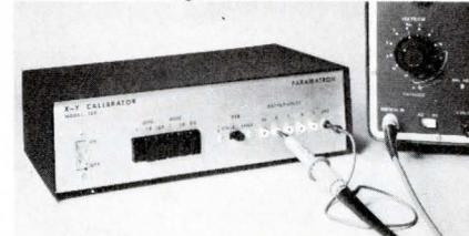
Model 132 gives you a dc or square wave output up to 1.0 MHz from 0.10 to 10.0 V. A crystal oscillator and ic dividers provide time base calibration with  $\pm 0.005\%$  accuracy. Rise and fall times are  $< 40$  ns when 10X scope probe is used. Price, \$99.50 in kit form or \$198.50 assembled. Delivery, 30 days. Paramatron Corp., Box 9207, Rochester, N. Y. 14625.
