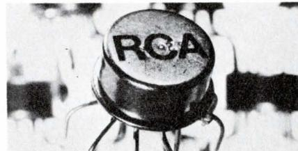
The CA3064 makes AFT practical for receivers with low-level if output. The device has a built-in input amplifier for a 20 dB improvement in sensitivity. Operating range is  $-40$  to  $85^\circ\text{C}$ , and it's in a 10-lead TO-5 package. Price is \$1.40 ea. in 1000 unit quantities. RCA/Electronic Components, 415 S. 5th St., Harrison, N. J. 07029. (201) 485-3900.
