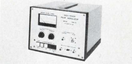
This series includes standard units with peak outputs of 3.5 kV at 3 A, 5 kV at 2 A, and 100 V at 100 A. Pulse regulation is held to ±1.0% for ±10% line variation and zero to maximum duty cycle variations. Pulse-to-pulse amplitude jitter is 0.05% max. \$985. Bertan Associates, Inc., 15 Newtown Rd., Plainview, N. Y. 11803. (516) 293-5340.
