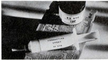
SS-570 ink can be silk screened directly onto matrix boards and ceramic wafers to provide conductive paths. It can also be sprayed or brushed on for shielding and grounding applications. Advantages include low-temp. cure cycles (94 $^{\circ}$ C-160 $^{\circ}$ C), thermal and environmental stability, ease of application, and low resistivity ( $< 0.01$   $\Omega$ -cm). Rogers Corp., Rogers, Conn. 06263.
