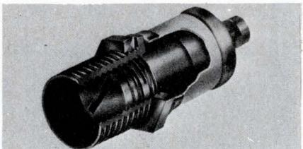
An improved and simplified drive mechanism has increased the Q of these air trimmer capacitors over other std. air units. Typical readings are 5000 at 10 pF and 10,000 at 3.5 pF. This series includes self resonant freq. above 6 GHz and low dynamic noise during adjustment. Johanson Mfg. Corp., 400 Rockaway Valley Rd., Boonton, N. J. 07005.
