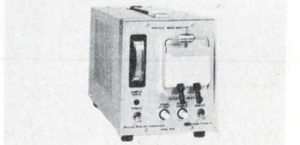
The Model 3200 monitors the airborne particle mass concentration directly. Instead of the hours required by filter type samplers, the instrument gives you the aerosol mass concentration in minutes. Concentration range is 1-100,000 micrograms/meter<sup>3</sup>. Thermo-Systems Inc., 2500 Cleveland Ave. North, St. Paul, Minn. 55113. (612) 633-0550.
