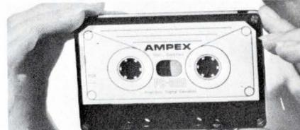
Series PC-800 precision cassette was designed specifically for cassette tape drives used as computer peripheral devices. It uses a precision metal plate, steelbearing mounted fixed hubs, and a four-point tape path system. Other features: self-aligning precision rollers, new pressure pads and a new hub construction principle. Ampex Corp., 401 Broadway, Redwood City, Calif. 94063. (415) 367-4151.
