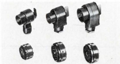
Series UW waterproof connectors are now available with 4, 9, 14, 19, or 30 contacts whose current ratings range from 11 to 41 A. They are for power and control circuit uses in mobile radar, radio, teletype, and related communications equipment. Both plugs and receptacles, which are polarized to prevent mismatching, can be fitted with either pin or socket contacts with solder turret terminations. Elco Corp., Willow Grove, Pa. 19090. (215) 659-7000.
