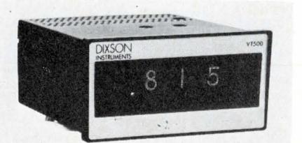
The manufacturer uses LSI circuitry in this full 3-digit meter with 0.5% accuracy. The instrument has an automatic zero, internal calibration voltage, and 100 μV resolution. You can operate it on either 117 Vac or 12 Vdc. The VT 500 costs \$139 and is available from stock. Dixon Inc., Box 1449, Grand Junction, Colo. 81501. (303) 242-8863.
