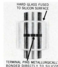
With the silicon die metallurgically bonded between terminal pins of the same thermal coefficient, the hard glass sleeve is fused to the entire outer silicon surface. Result — a voidless, monolithic structure.
