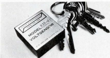
The "-01" series VoltSensors have a max. drift of  $< 0.1$  mV/ $^{\circ}$ C (typ. 0.05 mV/ $^{\circ}$ C), hysteresis specified  $< 1$  mV (typ. 0.5 mV) and an output rise and fall time of  $< 1$   $\mu$ s. The "-01" VoltSensors come in single set point, dual set point and dual set-dual out. California Electronic Mfg. Co., Box 555, Alamo, Calif. 94507. (415) 932-3911.
