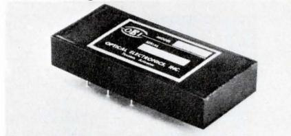
The Model 5636 gives you an output voltage equal to the instantaneous product of load voltage and load current. Sensitivity is  $\pm 10$  V full scale output for 10 mW of load power and it has a typical accuracy of  $\pm 0.3\%$ . Price is \$125 ea (1-9), \$102 (10-29), with immediate delivery. Optical Electronics, Inc., Box 11140, Tucson, Ariz. 85706. (602) 624-8358.
