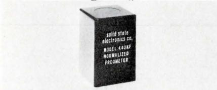
Normalized Freqmeter will linearly convert freq. or rep. rate of signals to a proportional dc voltage. This is done with four models over an input freq. range extending from 0 to 100 kHz—Model 410KF, 0 to 100 kHz; Model 420KF, 0 to 1 kHz; Model 430KF, 0 to 10 kHz; Model 440KF, 0 to 100 kHz. Solid State Electronics Corp., 15321 Rayen St., Sepulveda, Calif. 91343. (213) 894-2271.
