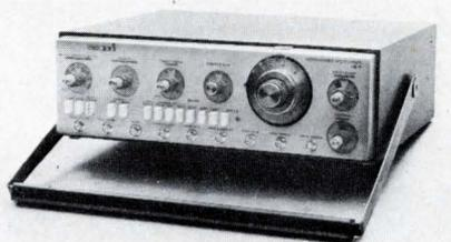
The F55 is the top-of-the-line unit in Interstate Electronics Corp.'s new line of five function generators. All units have a frequency range of 0.0005 Hz to 10 MHz and variable pulse width is standard. The F55 includes phase lock and sweep in the same unit. Sweep limits are set right at the frequency dial.
