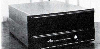
Model M200C is a fast access, head-per-track type mass memory. It is available in four capacities ranging from 426,000 to 3,408,000 bits. Average access time is 8.7 ms. The number of data tracks varies from 16 to 128 with 26,624 bits/track. Three timing tracks are included providing a bit clock, sector and origin pulse. Applied Magnetics Corp., Computer Memories Div., 75 Robin Hill Rd., Goleta, Calif. 93017. (805) 964-4881.
