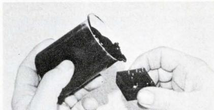
New two-component Epo-Tek 920-FL epoxy compound is a smooth-flowing paste when mixed, with a viscosity at 79°F of 14,000 cps. It has an 8 hr. pot life, and cures in 1 to 2 hr. at 60°C, and in 30 min. at 80°C. Thermal conductivity by the comparative method is 7.55 BTU in/ft² hr. °F. Dielectric constant at 1 MHz is 6.07, with a diss. factor of 0.021. Epoxy Technology, Inc., 65 Grove St., Watertown, Mass. 02172.
