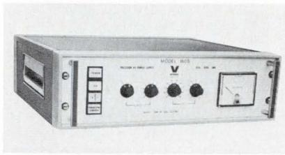
These precision supplies feature low ripple and accurate digitally-selectable output voltage. Output is continuously adj. from 1 kV to 20 kV at 3 mA on the Model 160, and from 10 kV to 30 kV at 1 mA max. on the Model 170. Accuracy of the output is within 0.25% of the selector switch settings. Output voltage is line and load regulated to within 10 ppm. Velonex, 560 Robert Ave., Santa Clara, Calif. 95050. (408) 244-7370.
