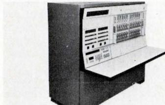
New AD/five 10 V-reference computer is a totally modular system that permits ease of expansion at a relatively low cost. It can be "married" to any digital computer to form a single hybrid system. When not serving as a multiple-console hybrid, it can function as a stand-alone analog computer. Applied Dynamics, Box 1488, Ann Arbor, Mich. 48106. (313) 971-4444.
