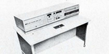
New tester is for automatic functional checkout of ICs, arrays, PC cards, and complete subsystems. Model 4400 generates and monitors up to 20,000 tests/s, enabling up to eight different test stations to be multiplexed. It performs Go/No Go testing and alternately acquires parametric readings of either current or voltage at any pin or bias supply within the system. Datatron Inc., 1562 Reynolds Ave., Santa Ana, Calif. 92705.
