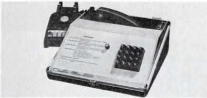
New terminal operates on six ordinary batteries and weighs only 7½ lbs., including its attache carrying case. Designed for use with computer-controlled voice response systems, it converts an ordinary dial telephone into a remote I/O terminal. \$230. Technitrend, Inc., 7300 N. Crescent Blvd., Pennsauken, N. J. 08110 (609) 665-4910.
