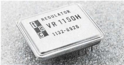
VR series regulators come with fixed voltage outputs (variable by an ext. pot) of positive 5, 6, 9, 12, 15, 18, 22, 24, 28, 32, and 36 V and negative 12, 15, 24, 28, 32 and 36 V. They have: foldback current limiting, 0.01% line and load reg., 0.005%/°C TC, and up to 40 V input. \$56.00. Transformer Electronics Co., Box 910, Boulder Industrial Park, Boulder, Colo. 80302. (303) 442-3837.
