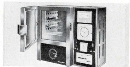
Small, economical thermal cycling chamber is good for handling about 1/2 lb. workloads of such items as modules and chips. Offering a temp. range from -65°C to +200°C, it has a SS indicating control instrument with two pots for cycling from high to low temp. and back again. Blue M Engineering Co., 138th & Chatham St., Blue Island, Ill. 60406. (312) FU 5-9000.
