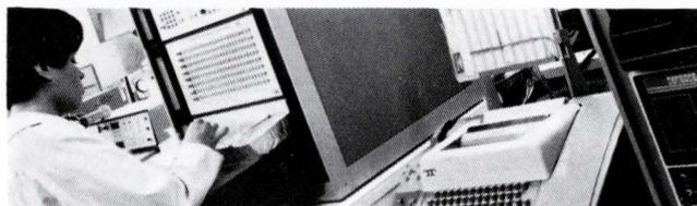
National's array of J259's handle the testing of its digital IC's smoothly and economically. For its linear-IC testing, National has turned to Teradyne's J263 computer-operated linear-IC test system.
