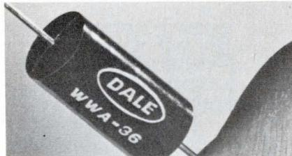
New precision bobbin wirewound resistors come in six models, 0.15 through 0.50 W. They meet requirements of Mil-R-39005 and Mil-R-93. Feature non-inductive winding, complete welded construction and good moisture resistance. They are available in a tol. range from 0.05% to 1%. Resistance range is from 10Ω to 5.4 MΩ. Dale Electronics, Inc., Box 609, Columbus, Nebr. 68601.
