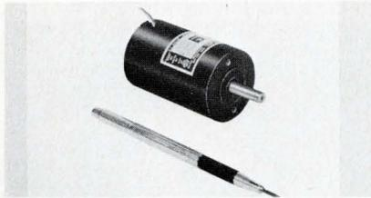
Type CFC line includes 3 hysteresis-synchronous versions with output speeds of 1200, 1800, and 3600 rpm, and 3 induction types producing 2.5 oz. in. at 3050 rpm, 2.0 oz. in. at 1400 rpm, and 1.0 oz. in. at 800 rpm. All motors operate on 115 Vac, 600 Hz, single phase. Weight is 11.5 oz. \$58.00. Globe Industries Div., of TRW, Inc., 2275 Stanley Ave., Dayton, Ohio, 45404. (513) 228-3171.
