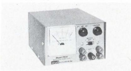
Model PS-30 provides a regulated (0.01%) continuously adjustable output covering the range from 0 to 30 V at currents from 0 to 1 A. Output voltage and current are monitored by a front panel meter and are isolated so that either terminal may be grounded. AUL Instruments, Inc., 139-30 34th St., Flushing, N.Y.
