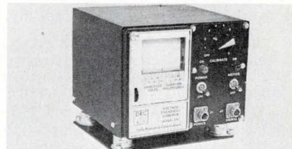
Recorder provides a long term, permanent record of the amplitude, duration, and time of occurrence of any power line voltage transient. Transients ranging from 5  $\mu\text{s}$  to  $>128$  ms in duration and 1 to 100 V in amplitude can be detected and recorded. Detection accuracy is  $\pm 1\%$  for amplitude detection and  $\pm 3\%$  for duration detection. Data Research Corp., 2601 E. Oakland Park Blvd., Ft. Lauderdale, Fla. 33306.
