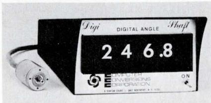
These SS shaft to digital converters, convert any shaft input into four character BCD information. Their output corresponds directly to the shaft angle. They simultaneously provide a 4 digit, 0 to 359.9° display, with a resolution of 0.1°, and an accuracy of ±0.1°. They can make 400 conversions/s. Computer Conversions Corp., 6 Dunton Ct., E. Northport, N. Y. 11731.
