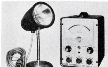
New SS Model 932 is for industrial inspection work where machine speeds exceed the rate the eye can follow. Large speed readout meter; four scales — 0-1000, 3000, 10,000 and 30,000 rpm. High sensitivity input (200 mV pk-pk). Power Instruments, Inc., 7532 N. Lawndale Ave., Skokie, Ill. 60076.
