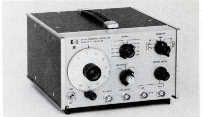
The Hewlett-Packard Model 3310A (\$575) voltage-controlled function generator features ramp and pulse functions in addition to sine, square, and triangle, plus dc offset. It provides 15 V pk-pk output into 50 $\Omega$ . Frequency range is 0.5 mHz to 5 MHz.
