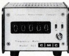
Model 905 is a 15-MHz counter which incorporates a 1-MHz crystal oscillator and a 5-digit readout. The unit comes in a 3½ x 5 x 7 in. package with tip-up stand for easy visibility in bench work. It sells for \$395. Computer Measurements Co., 12970 Bradley Ave., San Fernando, Calif. 91342. Booths 1006-08.
