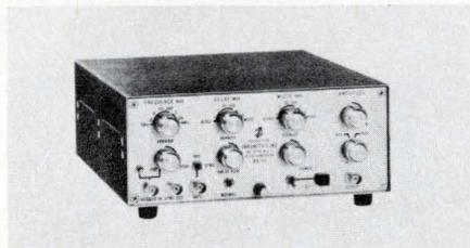
Model PG-11 provides single (delayed) pulses, pairs, sync pulses, and manual single-shots at amplitudes to ±15 V, and with 4-ns rise-times. Repetition rates are variable from 10 Hz to 20 MHz; pulse widths from 30 ns to 10 ms; delay from 40 ns to 10 ms. Chronetics, Inc., 500 Nuber Ave., Mt. Vernon, N.Y. 10550. Booth 1419.
