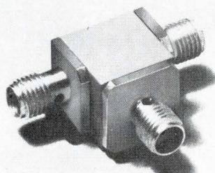
New compact coaxial circulator (MA-7K164) has high isolation of 20 dB minimum, with  $\sim$  low loss of 0.3 dB maximum over the frequency range of 8.5 to 9.6 GHz. Peak power is 1 kW and VSWR 1.2 maximum. Microwave Associates, Burlington, Mass. 01803. (617) 272-3000.
