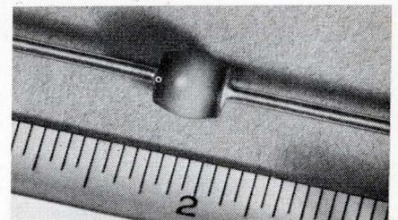
This is one of the new 3-A rectifiers showing the "Metoxilite" encapsulation prior to painting and marking. It is 0.165 in. long and 0.180 in. at the widest point.
