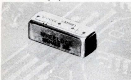
Series 442S 5-V relays require about 60 mW per pole to operate. They occupy only 0.05 in<sup>3</sup>/pole, and are only 0.258 in. high. Available in 1- to 4-pole models with contacts rated at a full 7 W, they weigh 1.9 g/pole. Operating temp. range is -65° to +85°C. Wheelock Signals, Inc., 273 Branchport Ave., Long Branch, N. J. 07740. (201) 222-6880.
