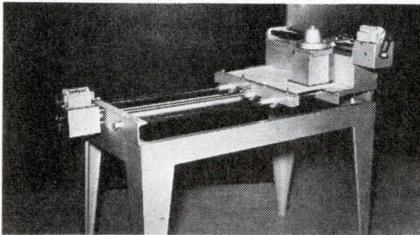
This printer makes it practical for small quantity users to make their own high quality multiple silk screen positives for PC boards. Using a negative or Mylar film, it prints five automatic exposures per minute on a roll of paper or film. Klann Inc., Box 2398, Waynesboro, Va. 22980. (703) 942-8351.
