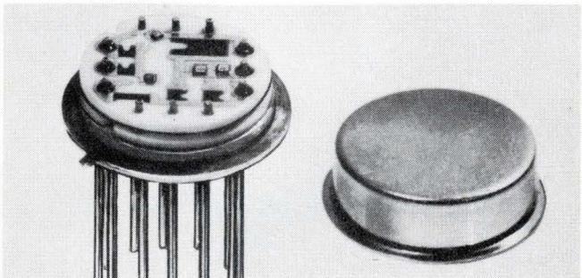
Useable also as a dual-gate function, these hermetically sealed TO-8 devices operate between 4 and 35 V. Control inputs may be DTL or TTL. Series 850 provides 700 mA output; Series 851, 350 mA; both operate  $-55^{\circ}$  to  $125^{\circ}\text{C}$ . CTS Microelectronics, West Lafayette, Ind. 47906.
