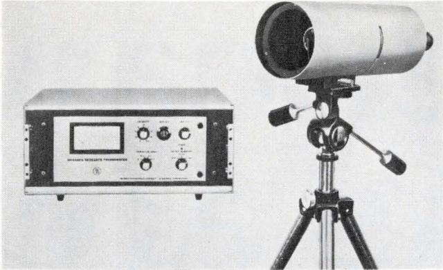
This infrared thermometer can measure the temperature of objects both near and far. It will also monitor fast-moving objects, or transient heat phenomena as short as 3 ms (55 Hz). Total temperature range is from  $-20^{\circ}$  to  $3200^{\circ}\text{C}$ , in four overlapping ranges. Sensitivity at  $20^{\circ}\text{C}$  is  $0.5^{\circ}\text{C}$ ; absolute accuracy is  $\pm 1\%$  o.f.s.
