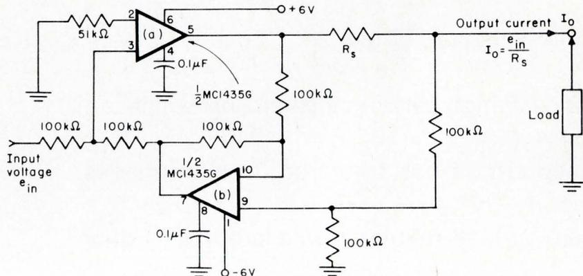
current and governs the output voltage of amplifier (a) for regulation. Output-current linearity vs input control voltage is good, with errors of less than 1%. Frequency response is limited to that of the open-
