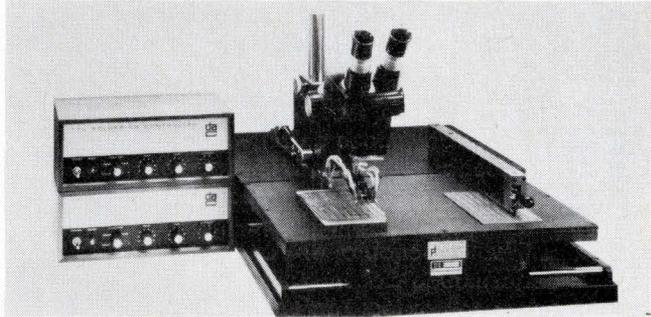
A visible tooling template gives fast positioning of the circuit board (to 8 x 8 in.) under the soldering head. There is a magnetic transfer system for placement. Dual power supplies. \$4900. Development Associates Controls, 725 Reddick Ave., Santa Barbara, Calif. 93103.
