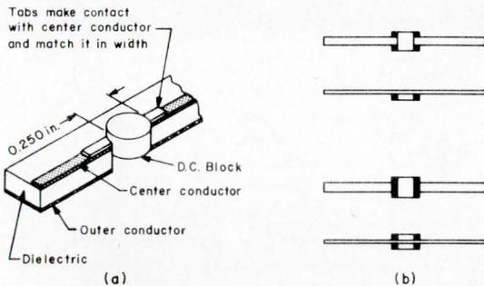
**Fig. 2: Discrete passive device (dc block) mounted on stripline (left).** This type device has soft copper tabs which match the stripline's center conductor. The tabs can be either soldered or spot welded. Low inductance is inherent in the design and the insertion loss is typically 0.25 dB max. from 0.5 to 4 GHz. VSWR is typically 1.1:1 up to 4 GHz. Discrete devices for microstrip dc blocks (right).
