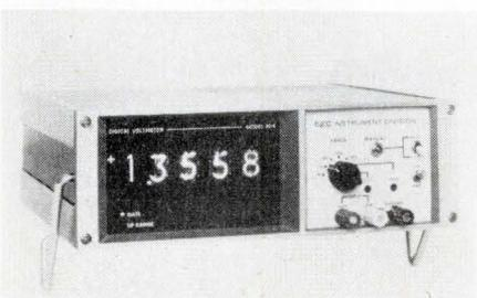
Four dc voltage ranges span 1 to 1000 V. Sensitivity, 1-V range, is 100  $\mu$ V. Resolution, 0.01% f. s. Accuracy, 0.02% reading  $\pm 1$  digit at 0-100% f. s. Overranging, 130%. Model 404, \$595. Tyco Labs., Bear Hill, Waltham, Mass. 02154.
