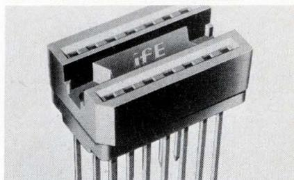
These 14-lead sockets have large tapered entry channels for quick lead insertion into dual leaf contacts. Polysulfone body provides anti-rotate pockets for hex nuts for easy assembly to the chassis. Contacts are beryllium copper with std. gold and tin contact plating. Plastic Mold and Engineering Co., 265 Wampanoag Trail, Box 4265, East Providence, R. I. 02914.
