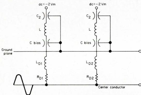
**Fig. 8:** This circuit overcomes the problems found in the circuit of Fig. 7. The capacitor ( $C_{Bias}$ ) resonates with the self-inductance of the diode at the transmitting frequency, resulting in an effective rf resistance. A low impedance path now exists between the center conductor and ground.
