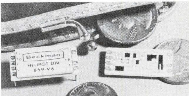
Series 809 (positive output), Series 859 (neg.) have fixed outputs from 5-28 V. Load regulation, 0.003%/mA. Ripple attenuation, 34 dB. I/O differential, 2 V min. \$13.50 ea. Tech. Info. Sect., HeliPot Div., Beckman Instr., 2500 Harbor Blvd., Fullerton, Calif. 92634.
