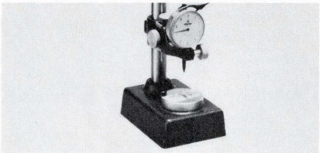
The S-1097 has a total thickness range of 0.025 in. and an accuracy compliant to all Federal regulations. Its contact point is hardened, precision-ground and plated tool steel. Flat, serrated, and domed anvils. Starnetics Co., 10639 Riverside Dr., North Hollywood, Calif. 91602.
