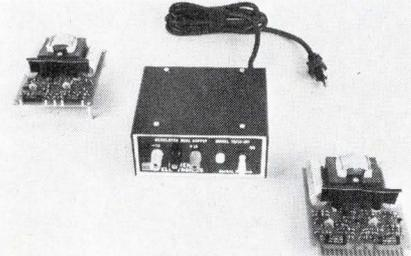
Model SEI-15/15-100 is an all silicon SS device. Basic unit provides 100 mA on each output; is short circuit proof; has 1-mV pk-pk ripple voltage; and is regulated to  $\pm 0.01\%$  line, 105 to 125 Vac 60 Hz, and  $\pm 0.02\%$  load, no load to full load. Salient Electronics, Inc., Blue Barns Rd., Rexford, N. Y. 12148. (518) 393-4590.
