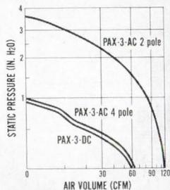
Globe's economical PAX-3 fans are the only units this size available for 28 v.d.c. We also make 200 v.a.c., 400 cps units in 2 and 4 pole versions. We specialize in custom design; we'll meet your specs. A servo ring at each end permits easy mounting in a 3 1/16" dia. hole for airflow in either direction. PAX-3 blowers meet MIL specs. Request Bulletin PAX.
