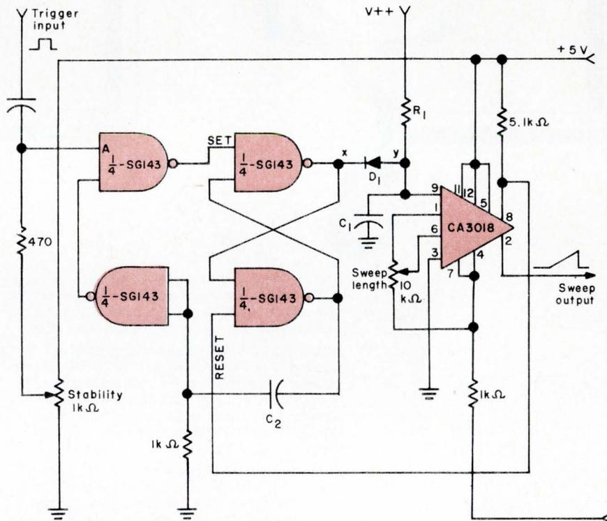
If you set the stability control so that input A of the first NAND gate is just below threshold, the circuit free-runs. It gives you a continuous train of sweep pulses, each with a period equal to the sweep time plus the hold-off interval.
