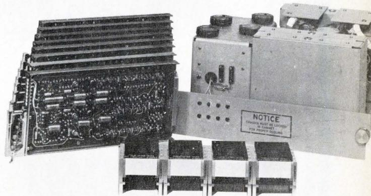
**Fig. 5. Packaging evolution of an electronic subsystem.** At the upper right is the initial design, while at the upper left it's seen redesigned into transistor page-card modules. The foreground unit shows its final repackaging into Standard Hardware Program modules by NAFI engineers.
