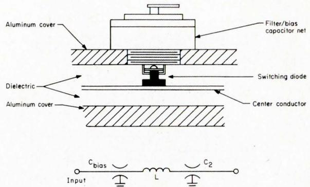
**Fig. 9:** Filter/bias capacitance network is used to achieve  $C_2$ ,  $L$ , and  $C_{Bias}$  (top). It is essentially a low-pass filter with a closely controlled input bias capacitance (bottom).
