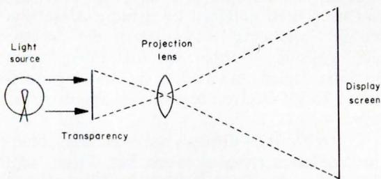
Fig. 2: A very basic display technique is the projection of a photographic transparency. This is a 2D system for non-real-time data.
