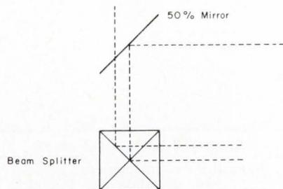
Fig. 9: With the addition of 50% mirrors the arrangement in Fig. 8 can be used to project six overlay images.
