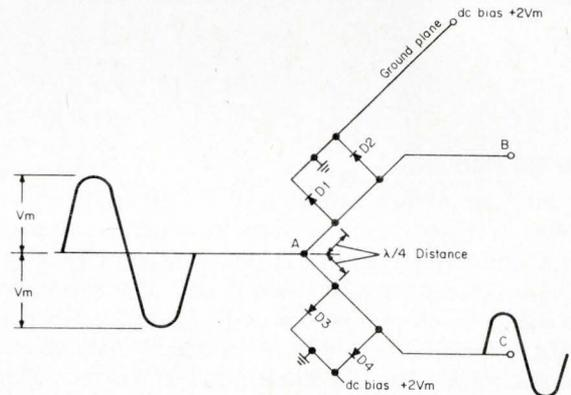
**Fig. 6: Simple parallel diode switch.** D1 and D2 in leg AB are forward biased and will conduct. Ideally, in this state, they will short any signal in leg AB to ground. D3 and D4, on the other hand, are reverse biased and, as such, will not conduct. In this state D3 and D4 are ideally an open circuit, and the signal will be transmitted through leg AC.
