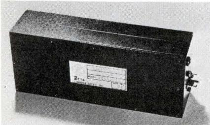
Model 4202 transmitter provides 200 mW output at 9.0 GHz. Frequency stab. is  $\pm 0.003\%$  over temp. range of  $-20^\circ$  to  $+65^\circ\text{C}$ ; input is 7 W at 28 V. All spurious and harmonic outputs are 75 dB below the carrier. Zeta Laboratories, Inc., 616 National Ave., Mountain View, Calif. 94040. (415) 961-9050.
