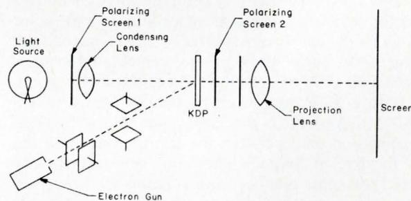
Fig. 5: Pockel electro-optical system most often uses KDP as the "optical" material. Electrical charges on the surface of KDP control the light passing through.
