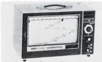
Omnigraphic™ Model 10, a 10-in. recorder, offer's 17 input ranges as standard, with the ability to read dc, mV, V, Ω, μA, and mA. Five chart speeds range from 0.05 to 20 in./min. Houston Instrument, 4950 Terminal Ave., Bellaire, Tex. 77401. (713) 667-7403.
