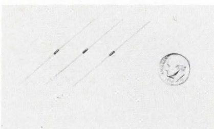
Type MRE-1/20 molded resistor conforms to all environmental requirements of MIL-R-10509F in tolerances to ±0.1% and temp. coeff. as low as 0 ±25 ppm/°C. Resistance range is 25Ω to 25 KΩ. Wattage rating is 1/20 W at 100°C and 1/40 W at 125°C. American Components, Inc., Eighth Ave. at Harry St., Conshohocken, Pa. 19428. (215) 828-6240.
