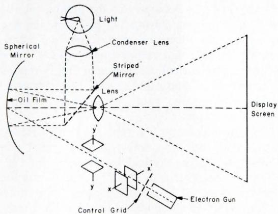
Fig. 3: This shows, basically, the Eidophor oil film display system. Because of the vapor pressure of the oil, a vacuum must be maintained.
