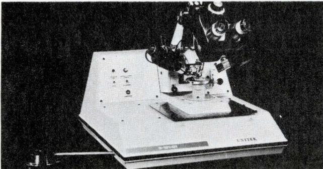
Model 8-151-01 has manual search control for multi-level bonding, adjustable wire looping, and a micromanipulator (x, y, and rotation). Patented bonding mechanism assures flat tool delivery. \$3400 fob. Unitek, Weldmatic Div., 950 Royal Oaks Dr., Monrovia, Calif. 91016.
