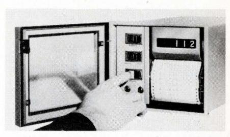
Input voltages, 0-1, 0-10, 0-50 mV. Three-digit print-out, plus two spaces for channel call-out, four for time, three more for external data. Options available. Model DL-1210, \$1575. Entex, Box 770, Friendswood, Tex. 77546.
