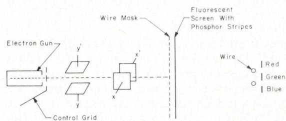
Fig. 12: The Lawrence color tube uses a single gun and deflection system. A potential on the wires in the grid determine which color is activated.
