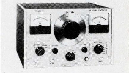
Model 61's frequency range is 85-135 MHz; additional band with adapter, 1-35 MHz. Short-term stability, 0.005%. Output level, 0.1  $\mu\text{V}$ -to-3 mV, metered. \$695. Radio Research, 189 Mt. Pleasant Ave., Rockaway, N. J. 07866.
