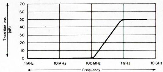
**Fig. 10:** Typical insertion loss curve of filter/bias capacitor network.
