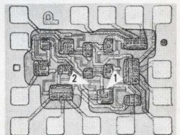
Hardened IC shows SiO<sub>2</sub> dielectric (1) and tantalum thin-film resistor (2).
