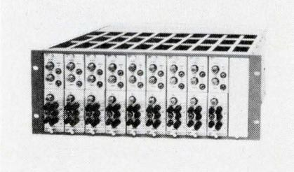
The thermocouple conditioning module plugs in, has bridge completion and calibration network cards. Ten channels, side by side. Switches for power, input/output, remote/local, etc. Incor, 29 Newtown Rd., Plainview, N. Y. 11803.
