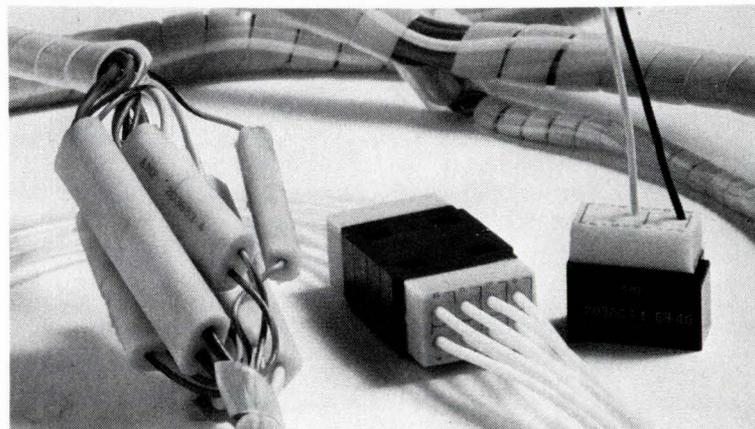
Terminal junction modules provide feedback or a feedthru capability for terminating wires; splices are also available. (Photo courtesy of AMP, Inc.)
