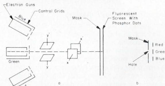
Fig. 11: Colored CRT displays are becoming common for presenting data. This sketch shows the basic elements of an RCA color tube, such as used for TV.
