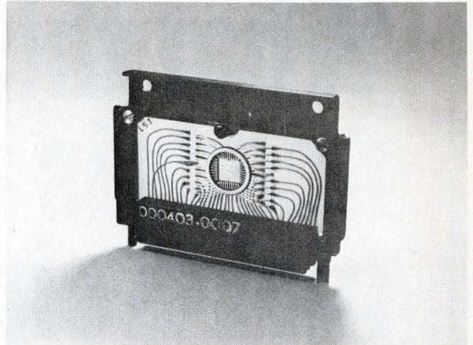
**Fig. 4. Not technology-limited,** the modules' circuit construction can take any form. For instance, this view of a module's innards shows an LSI device used to fulfill a specified function, whereas the module of Fig. 1 uses ordinary discrete components and PC board construction.
