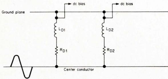
**Fig. 7:** Diodes  $D_1$  and  $D_2$  are represented by the series inductance and series resistance. The inductive reactance ( $X_{L,D1}$  and  $X_{L,D2}$ ) increase with increasing frequency and result in a high impedance path to ground, rather than in a short circuit. The circuit which overcomes this problem is shown in Fig. 8.
