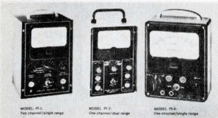
Measurements are accurate to 1% of range (0-500°F, single-channel; 0-500°F, -60 to 140°F dual-channel). Uses 100- $\Omega$  CP sensors. Recorder output. Prices start at \$120. RdF Corp., 23 Elm Ave., Hudson, N. H. 03051.
