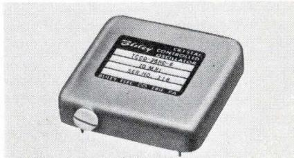
Two oscillators for std time base frequencies at 1 MHz (Type TCCO-26M-5) and 10 MHz (Type TCCO-26NC-6) have guaranteed stab. of 2 ppm over 0-60°C range. Low cost std module has pin terminals for PC board mounting and operation on 12 Vdc supply. Biley Electric Co., 2545 W. Grandview Blvd., Erie, Pa. 16512.
