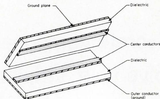
termed "microstrip"—essentially one-half of the stripline. Microstrip is the basic building block for what is often referred to as "MIC's" or Microwave Integrated Circuits (thin-film hybrids, thick-film hybrids, or monolithic integrated circuits).
