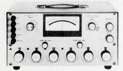
Model 1000 gives dc accuracy of  $\pm 0.0025\%$  of reading as a differential voltmeter;  $\pm 0.001\%$  as a decade voltage divider; dc ratio to  $\pm 0.001\%$ . Reference source and null detector. Precision Standards, Box 8361, San Marino, Calif. 91108.
