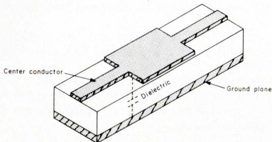
**Fig. 3: Stripline method for achieving the rf short.** The center conductor's width is increased and the rf short is essentially the capacitance between the center conductor and the outer conductor (ground plane). In this approach, due to the large separation between plates (typically 0.0625 or 0.125 in.) and the dielectric material's low dielectric constant (2.5-3.0), the capacitance attainable is small.
