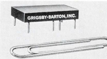
Input of the 14-pin GB811 is 5 Vdc for direct transistor logic drive. Package contains a reed relay, and a diode to suppress back emf. Contact rating is 3 W and breakdown volt. 200 Vdc. Electrostatic shielding is provided between coil and reed switch. Grigsby-Barton, Inc., 107 N. Hickory, Arlington Heights, Ill. 61312. (312) 392-5900.
