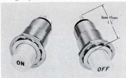
New line of miniature switches are 1½ in. from the front of the panel to the rear of the contacts. They come in momentary action up to SPDT and operate with either 115 Vac or 30 Vdc at 1 A res. or ½ A ind. Lens take either a std. T1¾ or ALC-100 neon bulb. Electro-Mech Components Inc., 1039 East Valley Blvd., San Gabriel, Calif. 91776. (213) 283-9213.
