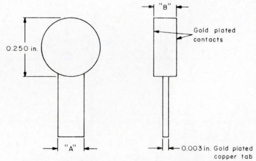
**Fig. 5: Discrete rf termination electrically and mechanically matches the stripline.** Typical dimensions are  $A=0.080$  in. and  $B=0.125$  in.
