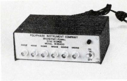
Frequency stability and accuracy are 0.005%. Model SS400 gives sync pulses at 200, 400, 800, 1600, and 9600 Hz. Options available include frequency changes. \$98, from stock. Polyphase Instrument Co., Bridgeport, Pa. 19405.
