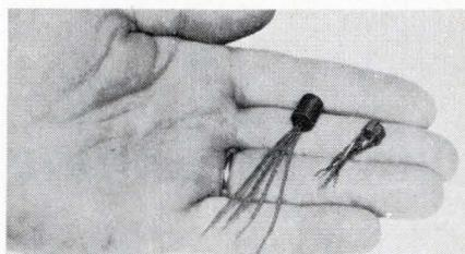
Pico transistor transformers and reactors have about 900 configurations available. Each features high efficiency plus a wide range in freq. response (-5 dB to -4 dB at 300 Hz, and +0.5 dB to +1.5 dB at 50 kHz). Essex International, Inc., Controls Div., Stancor, 3501 W. Addison St., Chicago, Ill. 60618.
