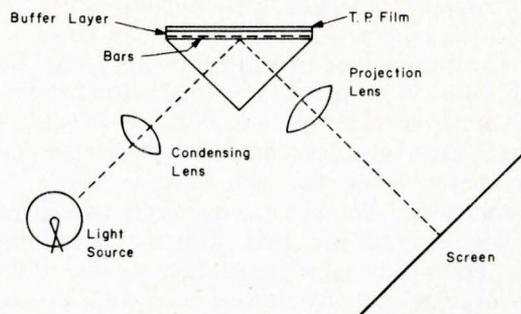
Fig. 4: The GE thermoplastic film projection system is similar in idea to the Eidophor system.
