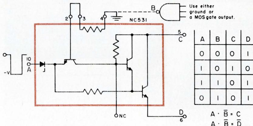
the zener provides the necessary logic levels (noise immunity): logic 0,  $\leq 6$  V; logic 1,  $\geq 6.5$  V.
