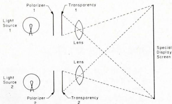
Fig. 7: This is a basic 3D optical projection system that has been used for both slides and movie projection. There has been very little use of this in displays, but it would increase information content in some applications.
