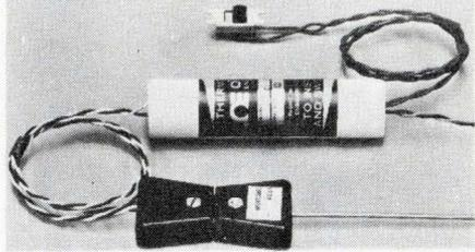
Self-powered thermocouple junction eliminates the need for ice baths and ovens. A pair of external "switch" leads provides instantaneous operation. Model XCJ comes in 16 different calibrations. Cases are cylinders 3 in. long by 3.4 in. in dia. All leads are 14 in. long. Omega Engineering Inc., Box 4047, Stamford, Conn. 06907.
