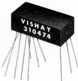
Because this network . . . and only this network . . . offers this spec combination: ■ TC Tracking:  $\pm 1.5$ -ppm/ $^{\circ}\text{C}$ . (using Vishay Resistors externally) ■ Absolute TC:  $0 \pm 1$ ppm/ $^{\circ}\text{C}$ . ■ Shelf Stability: 25ppm/yr. ■ Noise: Non-measurable. ■ Other specs include — Rise Time:  $< 10$  ns. . . Settling Time:  $< 100$  ns. . . Non-inductive (no ringing.)
