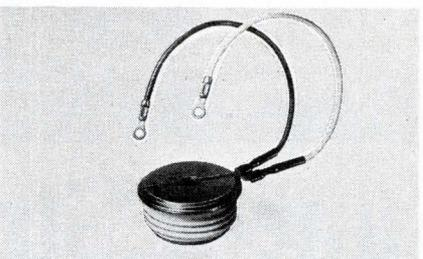
Type 282, "Full Capacity" thyristor is to replace parallel SCRs. Because of the all-diffused design, the thyristor's full inherent capacity is realized. Characteristics include a guaranteed  $dv/dt$ , low thermal imp., high surge current capability (to 7000 A), and high transient voltage capability. Westinghouse Semiconductor Div., Youngwood, Pa. 15697. (412) 255-3693.
