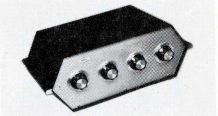
Three units (four decades ea.) provide ranges of 1-9999, 10-99,990, 100-999,900  $\Omega$  with 1% accuracy. Dielectric strength, 2 kV. Dissipates 100 W intermittently. Dale Electronics, Box 609, Columbus, Neb. 68601.
