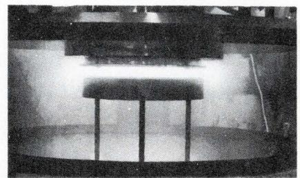
Physics of the plasma has been changed to intensify the generation of ions which cause the sputtering process. Three advantages are higher deposition rates, greater uniformity in coating and films, and a "getter" effect which enhances film purity and process equilibrium. Materials Research Corp., Scientific Instruments Div., Orangeburg, N.Y. 10962.
