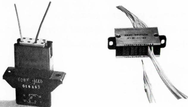
Weight and volume savings rendered by terminal junctions (when compared with terminal strips) become appreciable as the wire becomes finer. The protective grommet's sealing action on the terminal junction (right) eliminates the contamination and shorting hazards of the exposed terminals. Terminal junctions on relay offer fast connection and environmental protection. It is the first step towards an integrated termination system. (Photo courtesy of Deutsch-Filters.)
