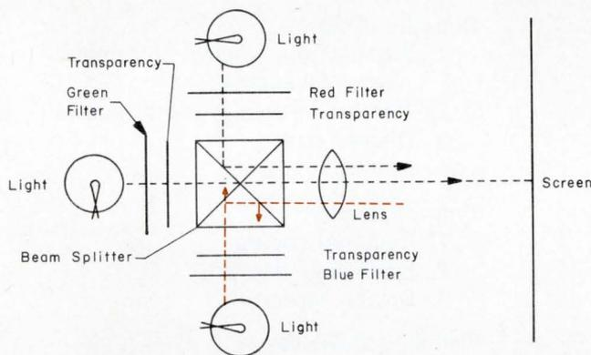
Fig. 8: Optical overlay for converting black and white transparencies to color, and displaying several sources on the same viewing surface.
