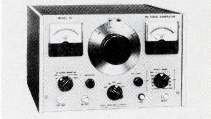
Model 61's frequency range is 85-135 MHz; additional band with adapter, 1-35 MHz. Short-term stability, 0.005%. Output level, 0.1  $\mu$ V-to-3 mV, metered. \$695. Radio Research, 189 Mt. Pleasant Ave., Rockaway, N. J. 07866.
