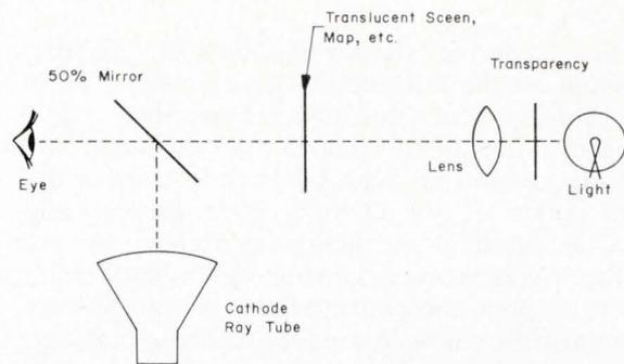
Fig. 10: An electronic TV type display can be combined with a projected display, map or a drawing board, etc. With this system changing information can be combined with more permanent data.
