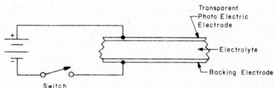
Fig. 6: An experimental system by Varian has a new photographic film or paper whose latent image is developed electrically.
