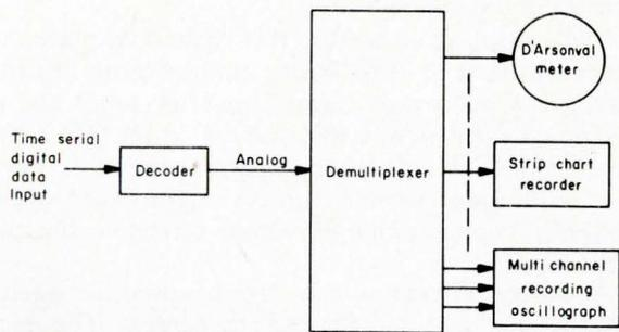
Fig. 1: Here are the elements of a conventional multiple display system that you can expect to see with some systems.
