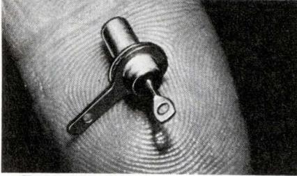
Metal diodes protect elements in applications where fast firing, low leakage current, and relatively low firing voltage are needed. Inherent firing voltage is 80 to 89 V. While the puncture voltage of MOS-FETs is generally lower than 85 V, this 85-V diode protects lower puncture voltages by appropriate biasing of the diodes. Victoreen Instrument Div., 10101 Woodland Ave., Cleveland, Ohio 44104.
