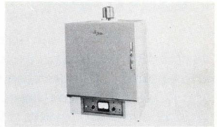
New LST (Low Skin Temperature) ovens have a safe ext. temp. of <50°C even when operating at 300°C. The ovens provide over 5 ft<sup>3</sup> of load area in a stainless steel chamber. The Temp. range is from 40° to 350°C. Electronic control is accurate to within  $\pm$ 0.15%. Hotpack Corp., 5137 Cottman Ave., Philadelphia Pa. 19135. (215) 333-1700.
