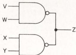
Now  $Z = (V W + X Y)'$  and if we let  $V = C$ ;  $W = D$ ;  $X = \bar{C}$ ;  $Y = D$  then  $Z = (C D + \bar{C} D)'$  =  $C \bar{D} + \bar{C} D$  which is the desired input function,  $B(J)$ .
