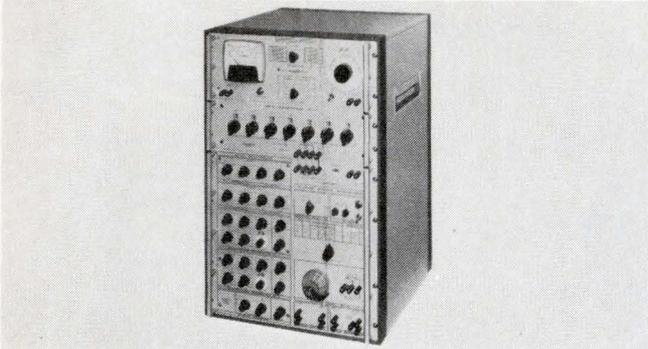
This instrument shifts/measures phase angle to an accuracy of  $0.015^\circ$  at most frequencies within the equipment's range. Model 311/RT-1/717 isn't affected by harmonics. Self-calibrating principle. 125-Vrms max. out. Dytronics, 4800 Evanswood Dr., Columbus, Ohio 43229.
