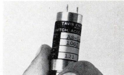
Model AS-1 instantaneous acceleration switch is for use with 12- to 40-Vdc supplies. It combines a basic inertial element with integral SS logic circuitry. Circuits are opened or closed within 1 ms, when peak acceleration exceeds the set point. Tavis Engineering Co., Bootjack Rd., Mariposa, Calif. 95338.
