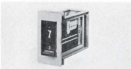
Sodeco ES4, a single-digit, high-speed impulse counter, has a 10-pos. readout switch, a transfer contact, a zero reset contact, and a predetermining switch. It performs many functions including programming, impulse storage, predetermining, counting, and control. Landis & Gyr, Inc., 45 W. 45th St., New York, N.Y. 10036. (212) 586-4644.
