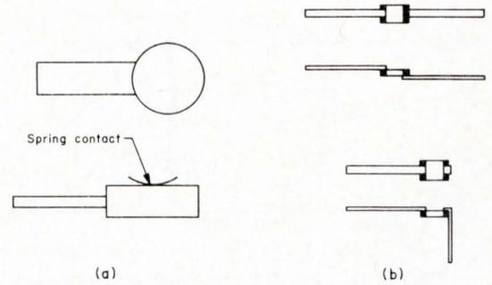
**Fig. 4(a): Two discrete rf shorts (one encapsulated and one not encapsulated) for stripline (left).** They have low inductance, high capacitance spring contacts or tab terminals to the ground plane, and are much smaller than the stripline approach. (4b) Some rf shorts for microstrip (right).
