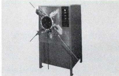
Type 852 sorter, operating with suitable test equipment, automatically tests and sorts over 5000 DIL ICs/h, magazine to magazine. Devices fed from the magazine are transferred to an index table, then advanced to a probe station for dc or dynamic testing. Daymarc Corp., 40 Bear Hill Rd., Waltham, Mass. 02154. (617) 894-2105.
