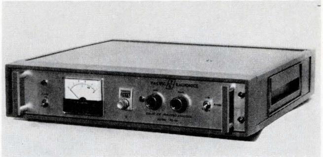
Model PR-101 analyzer measures dielectric constant and loss factor of sample materials that have an E of 26 or less. Accuracies are better than 2% absolute and 0.2% relative. Direct-reading output. Pacific Radionics, 581 Division St., Campbell, Calif. 95008.
