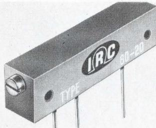
Type 60 has many features of the more expensive MIL types. It meets MIL Std. 202 tests for load life, humidity, shock, and vibration. It has a res. range from 10  $\Omega$  to 50 k $\Omega$ ; tol. is  $\pm 10\%$  with a power rating of 1 W at 70°C, derated to 0 at 125°C; temp. range is -55° to +125°C. IRC Div., TRW Inc., 2801 72nd St., N., St. Petersburg, Fla. 33733.
