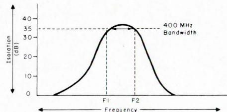
**Fig. 11:** Typical isolation per diode pair of switch using the filter/bias capacitor network.
