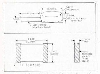
Competitors. Delevan inductor (top) is basically a coil on a tab with leads. Nytronics device is formed of two ferrite halves bonded together into a chip. Delevan also has a series of 0.065-inch high inductors with Qs of 35-45.
