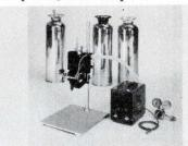
Model 410 Microshot dispenser has precision-machined metering cylinders that deliver 0.5 to 15 g/shot of twocomponent thermosetting plastics. Stainless steel containers  $(2\frac{1}{2} \text{ gal.})$ deliver components under constant pressure to the metering system. Fluidyne Instrumentation, 3685 Mt. Diablo Blvd., Lafayette, Calif. 94549. (415) 284-5824.
