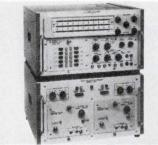
This microwave sweep system consists of the Model 650 sweeper, any combination of up to ten 650 series plug-in oscillators (250 MHz-40 GHz), the 9510 push-button control, and the 9511 plug-in container unit. Alfred Electronics. Booths 2C12 and 2C14.
