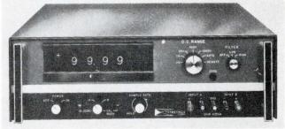
This automatic-ranging digital voltmeter has a sample rate of 10 samples/s, 10 µV sensitivity, with a readout accuracy of 0.01% over its five dc ranges. The display neither blinks nor has running numbers.
