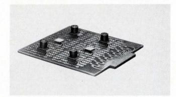
Larger inductors are being modified and improved for use with integrated circuits. These inductors are designed for flat mounting on pc boards with ICs.
