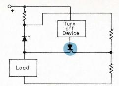
Fig. 5: This under-voltage circuit works on the same general principle as the circuit shown in Fig. 3. It operates as a bridge consisting of a zener, an output voltage, and two resistors. Decreases in load voltage make the gate positive with respect to the cathode, causing the SCR to turn on.
