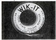
Wik-It desoldering tool is speciallytreated (with Mil Spec chemicals) tinned braid that quickly draws up solder when heat is applied with an ordinary soldering iron. It acts as a heat sink to protect delicate components, and leaves the joint resolder-ready. It cuts costs of equipment down-time, rework, trouble shooting, quality control and prototype building. It is sold as service kit or spool rolls; a sample is available on request. Wik-It Electronics Corp., Box 414, Fremont, Calif. 94537.
