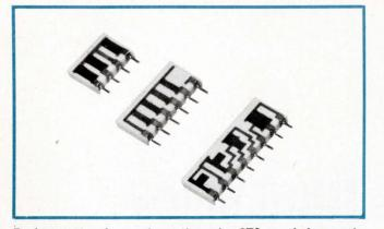
**Resistor networks,** such as these by CTS are being made by various manufacturers to meet the needs of integrated circuits. This type of packaging is only one of many types, such as flat pack and dual in-line, that are available.
