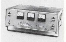
Type 2885 changes input watts to output dc volts. Linearity is  $\pm 0.02\%$ , dc to 2 kHz; 0.1% to 10 kHz. Circuit procedure allows use with power factors from unity to zero, with less than 0.02% degradation. A 150-V, 5-A input for 1-V out is standard; other ranges are available. Output to be fed to 5- or 6-digit DVM, or dc potentiometer. From \$1500. Hallmark Standards. Booths 2E07-09.
