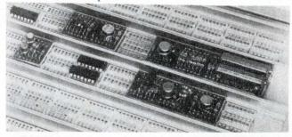
This high-density packaging system is specifically for DIP packages, and discrete packages mounted on plug-in cards. Six styles of plug-in modules are: Style A, PC card direct mounted; Style B, PC card with receptacles; C, platemounted receptacles without covers but with two position wire-wrap; D, same as C except with cover; E, same as D but with three position wire-wrap; F, PC card with receptacles, back-to-back.
