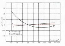
tance element, which is of all-metal composition deposited on a ceramic substrate. Resolution is infinite and CRV (contact resistance variation) is low—2% of RT or 20  $\Omega$ , whichever is greater. This is significant for trimmers used in balancing circuits and in circuits related to the input of high-gain op amps.
