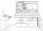
This system for RFI/EMC testing and spectrum monitoring is fully programmable. It consists of the Fairchild Spectrum Surveillance System Model FSS-250, interfaced with a Hewlett-Packard Model 2116B computer. It covers the freq. range of 20 Hz to 1000 MHz. Fairchild Electro-Metrics Corp., 88 Church St., Amsterdam, N.Y. 12011. (518) 843-2600. Booths 2D03-05.
