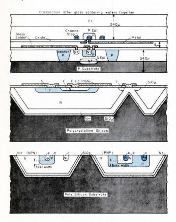
in the bulk material, where higher voltages can be accommodated. The company uses an anisotropic etch instead of Radiation's splash etch—to facilitate deep device structures in high-resistivity material. Signetics also uses FET current sources and thin-film resistors in its new linear ICs.
