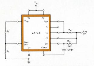
High-voltage floater. Base-emitter junction of current-limit transistor is zenered and added to  $V_{\rm rer}$  to form a pre-stabilized  $\pm 14V$  supply. This eliminates need for extra floating supply.
