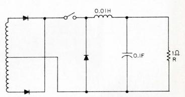
Fig. 7: A typical rectifier LC filter with resistive load. When the switch is closed, resonant charging will overcharge C, which will then discharge to normal level into load R. Since the diodes present reversal of the resonant portion of the current, there will be no undershoot at turn on.
