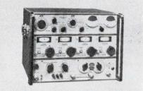
For testing all types of fm receivers, Model 2006 covers a total range of 4 to 1000 MHz with plug-in oscillators. Crystal calibrator with visual indication of zero-beat; counter output of 100 mV/50  $\Omega$  to 600 MHz, 50 mV to 1000 MHz. FM noise less than 40 Hz flat (12 Hz FIA); microphony less than 12 kHz at 0.5 g acceleration. Output variable from 0.1  $\mu$ V to 100 mV/50  $\Omega$ . Marconi. Booths 2D02-08.
