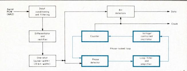
Bit synchronizer. To establish bit timing, the PCM input signal is conditioned and filtered to compensate for variations in amplitude, baseline offset and bandwidth. Passing the signal through a nonlinear element (such as a zero-slicer and /or rectifier) develops a frequency component at bit rate. The phase of this component is compared with the phase of pulses from the voltage-controlled oscillator (VCO). The error
