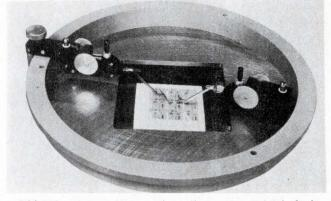
This 30-point probing station allows sequential indexing and testing of similar circuits on a single substrate, either manually or automatically. Actual contact with the item under test is through a newly developed probe positioner on the master probe station. You can adjust the pressure at the probe tip from a few tenths of a gram to 20 gm. (The company plans to market the probe positioner separately, as well as with the master station.)
