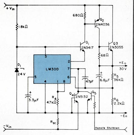
compensation terminal). This clamping action switches the regulator into a current mode, which protects the IC.  $(R_{sc} = V_{bc4}/I_{sc})$
