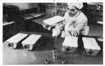
rendition without breakup at the slow speeds at which the astronauts will move. This scan rate can be easily converted to 60 fps for viewing on home TV receivers. A 320-line scan was chosen to obtain nearly equal vertical and horizontal resolution. The 10 fps mode will provide about 250 discernible lines on a home TV set, good enough for viewing.
