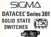
These new opto-electronic switching devices use a sealed-in lamp and photo conductive cells to drop.resistances from 10 ohms to 500 ohms. Smooth, non-mechanical turn-on means no interference, no transients, no bounce. Available with 1, 2 or 4 poles in 6, 12, 24 and 150V types.
