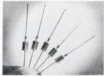
The TransZorb® 704-34 transient suppressors were designed mainly airborne applications where for large voltage transients, as described in MIL-STD-704A, endanger voltagesensitive circuits or components. It comes in the standard DO-13 package, has a clamping voltage of 34 V, and requires only  $1\Omega$  source impedance. Price in 100 piece quantities is \$3.25. General Semiconductor Div., Silicon Transistors Corp., Box 3077, Tempe, Ariz. 85281. (602) 966-7263. Circle 237 on Inquiry Card
