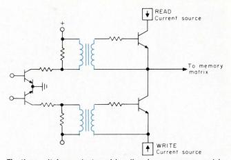
Floating switches select a drive line in a memory matrix, allowing either the read or write current to flow, each in its own direction. They "float" when the (read or write) pulse rises, because the inductive kick it produces in the drive lines must be isolated from the selection matrix. Pulse Engineering Inc., Santa Clara, Calif., puts four pulse transformers in a module designed for floating switches.
