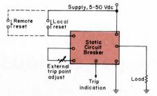
connecting an external resistor to it. Thus, you can select the exact current level at which you desire protection.
