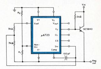
**Negative voltage regulator** accepts minus-input power supply. Breakdown of the pnp series pass elements limits the input voltage.
