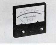
The Ultimeter has a 1% linear meter movement and a 0.5% linear pot, both calibrated to the meter scale. Set pointers operate the pot contact wipers. User's circuitry (IC op amps, Schmitt triggers, etc.) triggers a control action whenever signal level equals set-point value, even if meter movement fails. API Instruments. Booth 2G34.
