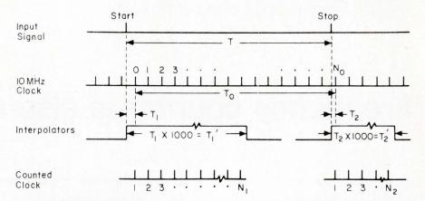
Fig. 2. The time-interval measurement sequence uses interpolation techniques to determine the usually uncertain times  $T_1$  and  $T_2$ . Computing circuits solve the equation for the unknown period as  $T = T_0 + T_1 - T_2$ .
