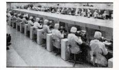
P&B also produces aero-space and military relays which are assembled, tested and sealed in a spacious clean room where all production is under our Intensified Control and Reliability Program.
