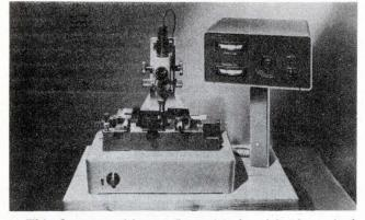
This fixture positions 1.5- or 2-in.<sup>2</sup> reticles in a single segment slide for use in the company's 4M mask-making machine.
