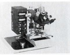
Bonding by thermocompression wobble-tool action is adaptable to semi-automatic setups. The operator aligns the die's beam leads with the leads of the workpiece, then pushes a button on the chessman x-y manipulator. The motor-lowered heated tool presses the beam leads against the workpiece. Then the top end of the tool tilts 1° and rapidly rotates twice, applying a uniform, controllable pressure sequentially to all leads.
