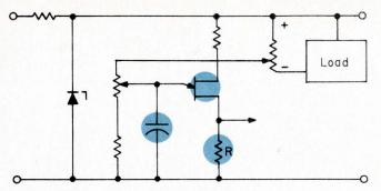
Fig. 4: Under-voltage circuit. This circuit is similar to that of Fig. 1, but opposite in the sense that decreases in load voltage raise the UJT emitter, sending a current pulse from C into R.
