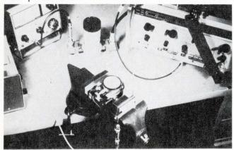
**X-band stripline test.** Vise applies a constant clamping force to the test fixture, which is a critical factor in obtaining reproducible results. For accuracy, a force gage is used.
