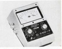
The GVM30 is a small lab meter that measures dc currents from 30 pA (f.s.) to 300 µA; voltages, 1 mV to 300 V; resistances, 1 k $\Omega$  to 300 M $\Omega$ . Both inputs are floating. The unit runs off of six type-C batteries, and has a recorder output. The London Co. Booth 2H26.
