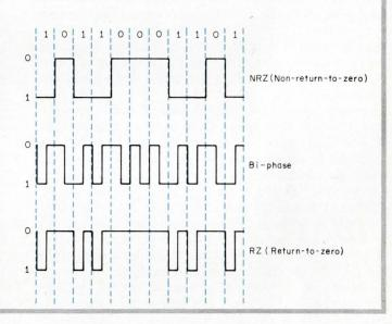
the effects of adjacent bits (intersymbol cross-talk). In practice, bit decision errors occur because the bit synchronizer cannot track the input signal precisely. When choosing system hadware, pay special attention to clock and vco (voltage-controlled oscillator) stability.
