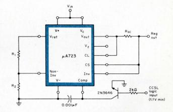
**Remote-shutdown regulator.** Complementary current-sinking logic from external digital elements lets regulator be turned OFF remotely. If you do not need current limiting, ground the CL pin and drive the CS input with 1 mA. This lets you use the internal series-pass device for shutdown.
