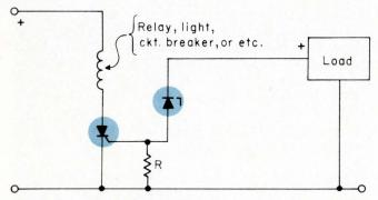
Fig. 3: This simple over-voltage circuit uses the zener voltage plus the SCR gate-cathode voltage as a standoff. When sensed output exceeds that sum, zener current flows into the SCR gate to fire the SCR.
