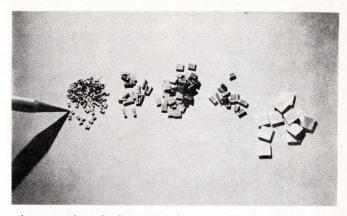
shows packaged glass capacitors by Corning, while this photo shows chip capacitors made by Vitramon for hybrid integrated circuits.
