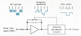
Integrate-and-dump method for coherent bit detection. The signal (with noise) is integrated over exactly one bit period. The logic circuits sample the signal at the end of the integration period to determine its binary state. If the integration period is not in phase with bit period, there will be crosstalk between adjacent bits.
