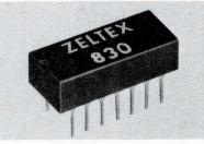
Model 830 fully-compensated op amp is the first in a series. Specs are: volt. gain of 300,000, drift of 20  $\mu$ V/°C, input bias current of 15 pA, slew rate of 6 V/ $\mu$ s common mode volt. of 10 V, and output of 10 V at 5 mA. Zeltex, Inc., 1000 Chalomar Rd., Concord, Calif. 94520. (415) 686-6660. Booths 2C06 and 2C08.
