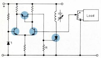
Fig. 2: This over-voltage circuit is more accurate than the one shown in Fig. 1. Here a differential amplifier operates as a level detector. When the sensed output voltage exceeds the level of the reference zener, Q1 and Q2 switch, turning on amplifier Q3 which furnishes a gate signal to an SCR, or driver power to a relay. Interchanging the base connection of Q1 and Q2 changes this circuit into an undervoltage detector.
