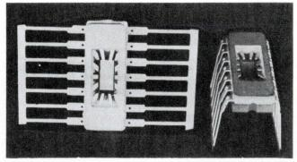
This DIP housing for ICs has a rugged, monolithic alumina ceramic base. In addition, a  $200-\mu$  microinch goldclad heat spreader gives excellent die-attach properties. The lead tips are coplanar for faster, more reliable lead bonds. Sealing preforms and lids are available for this TO-116 package, as is a 16-lead version. Mitronics, Inc., 132 Floral Ave., Murray Hill, N. J. 07974. (201) 464-3300.
