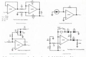
Like the recently introduced LM101A, this op amp offers input current advantages: a guaranteed 100-nA bias current with a 20-nA offset current, over the full military temperature range. And, the manufacturer claims, with no sacrifice in drift or offset voltages. These are also guaranteed over the full temperature range: 3-mV offset, and  $15-\mu V/°C$  offset voltage drift.
