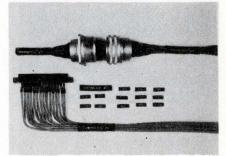
To permanently install the markers in skin-tight fit, simply slip them over the objects to be marked and apply moderate heat. Average shrink range runs from 35% to as much as 50%, depending upon material used. Heat needed for shrinking may be supplied by heat guns, contact tools, infra red radiation units, or ovens. Satisfactory shrink is achieved in 5 seconds with 450°F applied. E.C.P. Corp., 4726 Superior Ave., Cleveland, Ohio 44103. (216) 391-0444.
