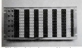
With this packaging scheme, a module can have any combination or arrangement of 14-, 16-, or 24-pin sockets and transistor-discrete component receptacles. You may use several interchangeable modules in multiple to achieve a specific optimal configuration.
