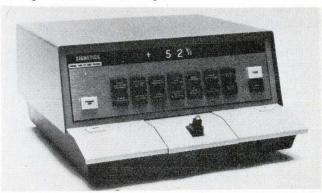
Model 1410 is primarily an op amp tester for preproduction testing: it is automatic and simple to program and operate. Its three modes of operation tell the operator what tests are programmed for pass/fail indication, whether a unit passed or failed, and how well that unit passed or failed as a percentage relative to the programmed limit for that test.
