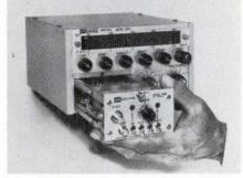
Model 5008-1 plugs into company's Model 5000 sweeper, covers 100-500 MHz with fundamental-frequency oscillator. Has 0-20 mW output, with calibrated power dial; is internally leveled to 0.2 dB. Harmonics, 27 dB down; non-harmonics, 60 dB down. \$1390. Kruse-Storke. Booth 2K29. Circle 286 on Inquiry Card
