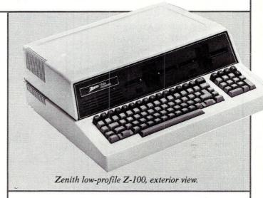
Video. The built-in video board (as mentioned above) can be used as a VT-52 cursor control compatible terminal, or as a high-resolution graphics display of 640 by 225 pixels. Composite monochrome video, composite sync, horizontal sync, vertical sync, and RGB video signals are generated for use with different monitors. We were provided with a Zenith 15" RGB monitor for our tests, and the display was quite good, with excellent linearity and color.
