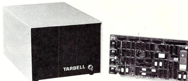
Tarbell 5-inch hard disk subsystems with amazingly low cost per megabyte are available in 5, 10 or 16 megabyte formatted configurations.
