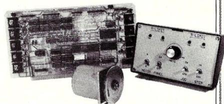
significant features of the system include motor ramping, automatic limit sensing, and internal or external step pulse count functions.
