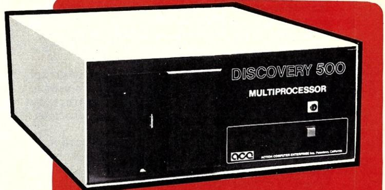
The DISCOVERY 500, a fully integrated desktop computer with 5 1/4" hard and floppy disks, supports up to 7 users. It is the ideal, low cost turnkey business system. The full size DISCOVERY supports up to 16 users with a wide variety of disk and tape subsystems. And remember, all DISCOVERY users have their own dedicated memory and 8-bit or 16-bit CPU, running CP/M-80\* or CP/M-86\*. Action's own multiuser multiprocessor operating system, the **dpc/os** † makes it easy.
