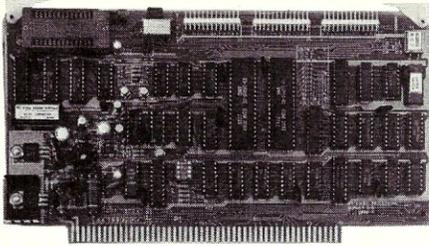
Our BURNER I/O has a complete EPROM programmer, two serial ports, one parallel I/O port with handshaking and memory management.
