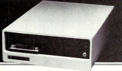
S-100 bus compatibility, Z80 CPU, high-density 5¼" Winchester disk, dual floppy disk capability, expansion to 1024 K RAM, 27 MB hard disk, and 20MB streaming tape cartridge drive. It comes with CP/M; Oasis and MP/M are available for multiuser support and may be upgraded for 8 users.
