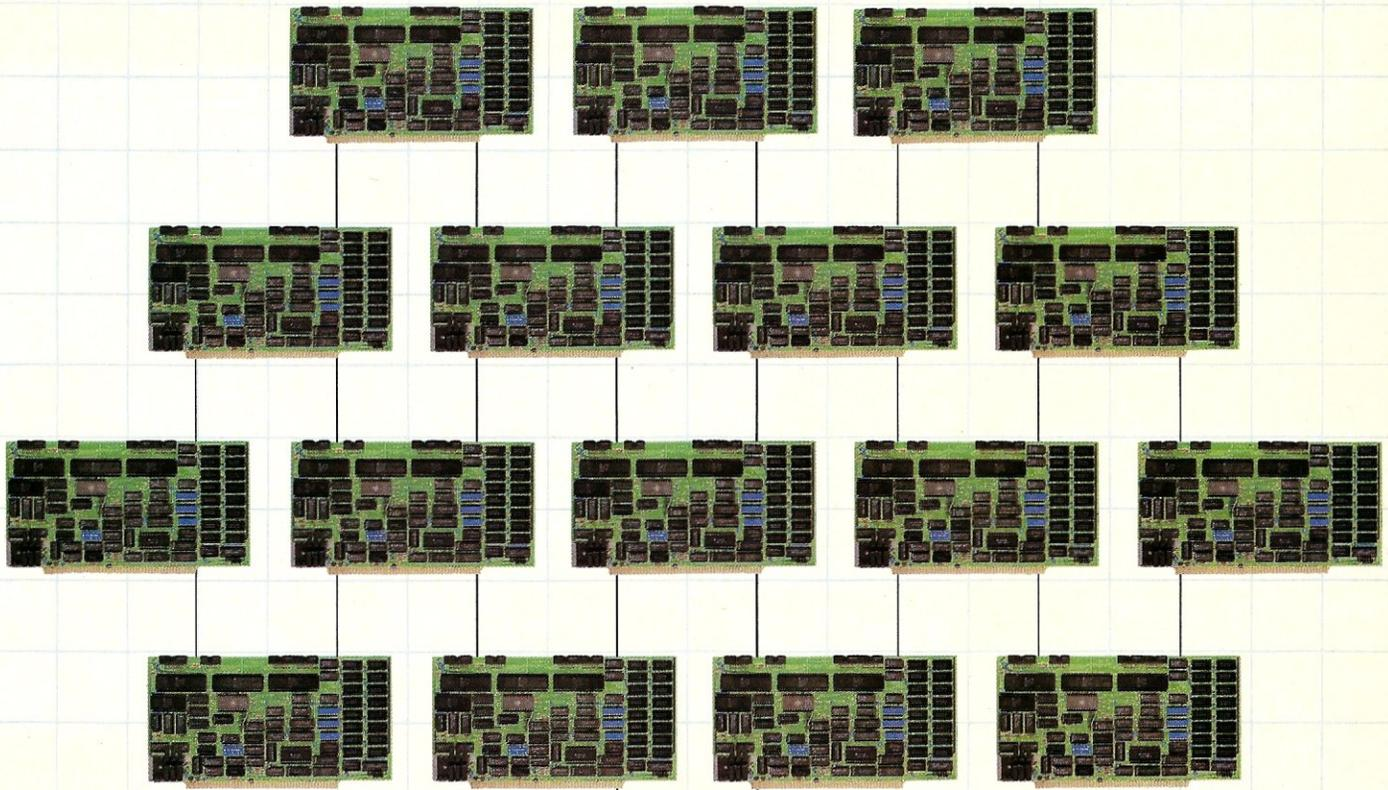
**SBC-1** (Above) A multiprocessing slave board computer with Z-80 CPU (4 or 6 MHz), 2 serial ports, 2 parallel ports, and up to 128K RAM. Provides unique 2K FIFO buffering for system block data transfers. When used with TurboDOS or MDZ/OS the results are phenomenal!
