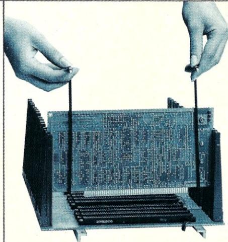
hook. When the entire hook is covered, shrink the tubing. Then make a 90° bend at (B) and a 180° bend at (C) and (D). To finish the card extractor, slide a 2" piece of heat-shrink over each half of the Tee-handle and shrink the tubing.
