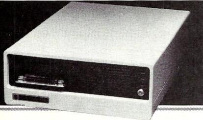
S-100 bus compatibility, Z80 CPU, high-density 5¼" Winchester disk, dual floppy disk capability, expansion to 1024 K RAM, 27 MB hard disk, and 20MB streaming tape cartridge drive. It comes with CP/M; Oasis and MP/M are available for multiuser support and may be upgraded for 8 users.
