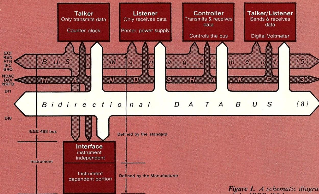
Figure 1. A schematic diagram of the IEEE-488 bus.
