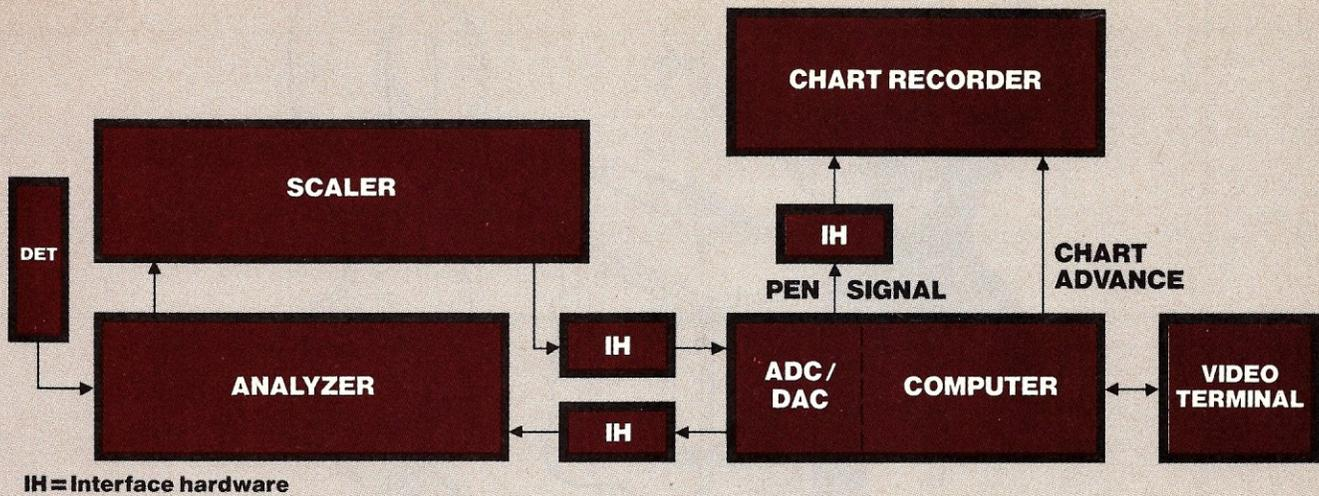
**Figure 1. Gamma scintillation spectrometer**
