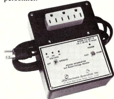
Connecting to the AC line with a standard 3-prong plug, the self-reset power interrupter can accommodate a 15-amp resistive load or a 10-amp inductive load.
