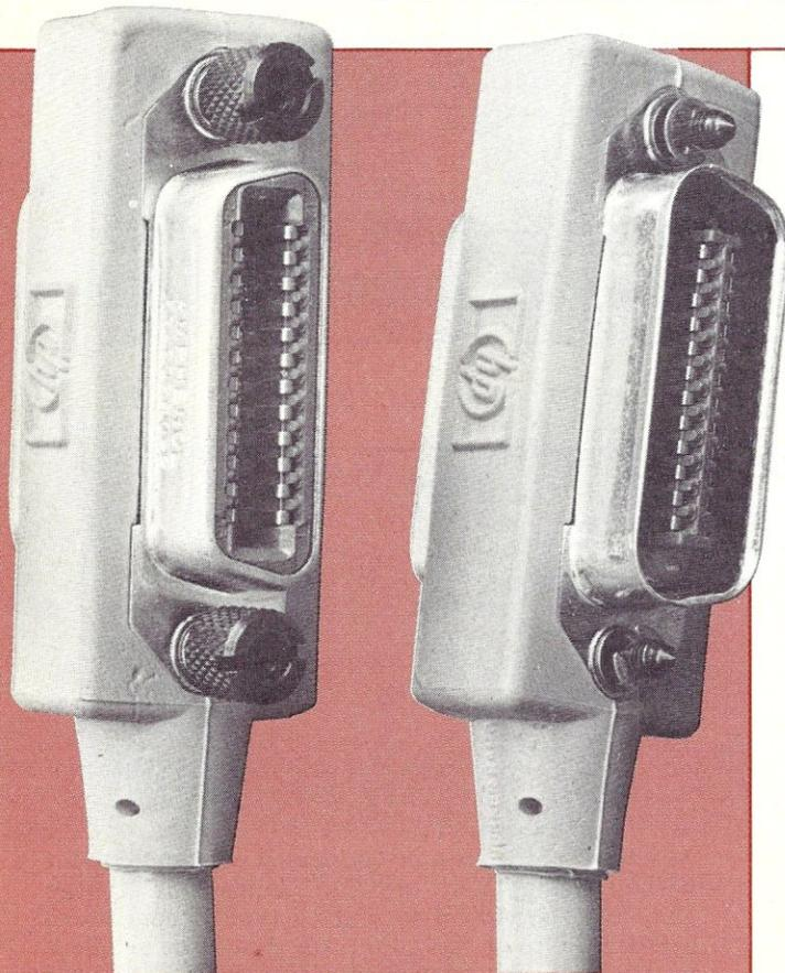
**Figure 2.** Typical 488 bus cabling and connectors. Note that the cables have male and female connectors on each end. This allows them to be "stacked." The cable has 24 conductors, in 12 twisted pairs, each pair being individually shielded. There is also a common shield around the whole cable. (Photo by J. Helton.)
