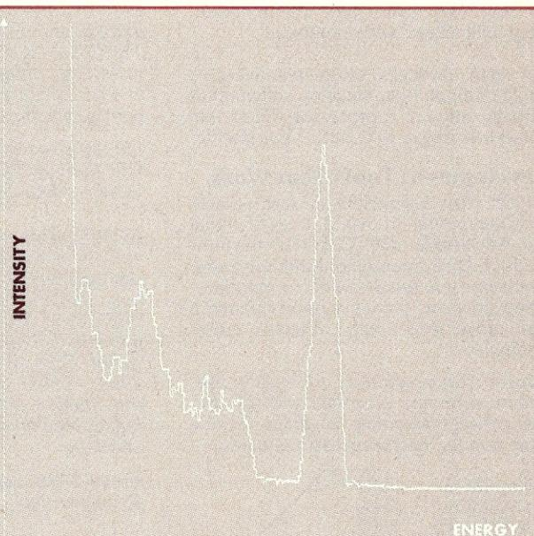
**Figure 2. Cs<sup>137</sup> spectrum replotted from disk. "Steps" are a result of using an 8-bit analog-to-digital converter.**
