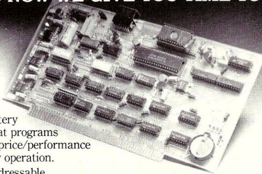
TimeEPROMmer, the S-100 CP/M\* compatible programmer that's useful every second of every day. A real time calendar/clock with lithium battery and an EPROM programmer that programs all popular eproms. Unbeatable price/performance ratio. Features designed for easy operation.
