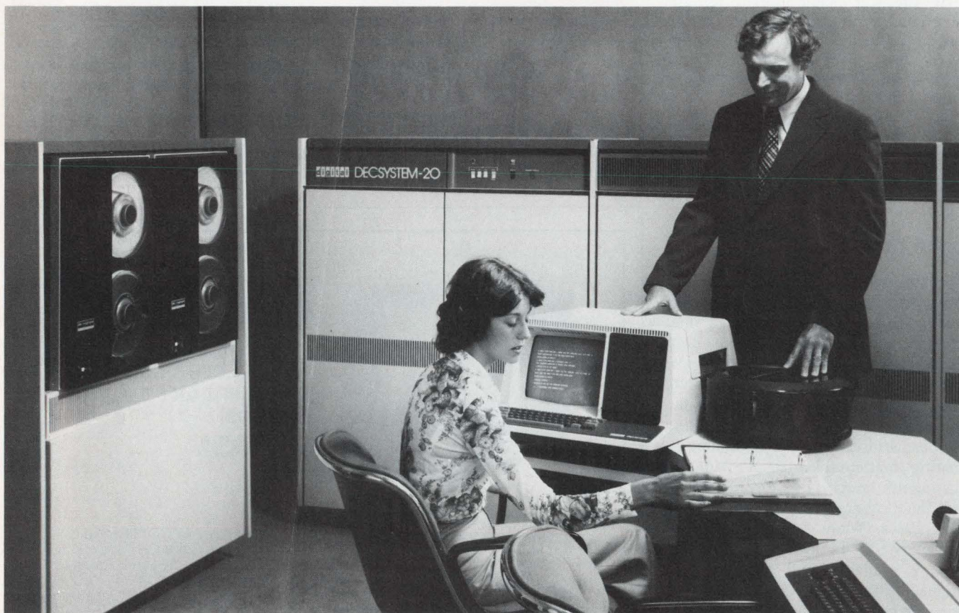
Digital Equipment's new DECsystem 20 features a PDP-11 utility processor as well as a new ECL-version of the processor contained in the largest DECsystem 10s. The 36-bit word length computer closes the gap between DEC's smallest and largest product lines.
