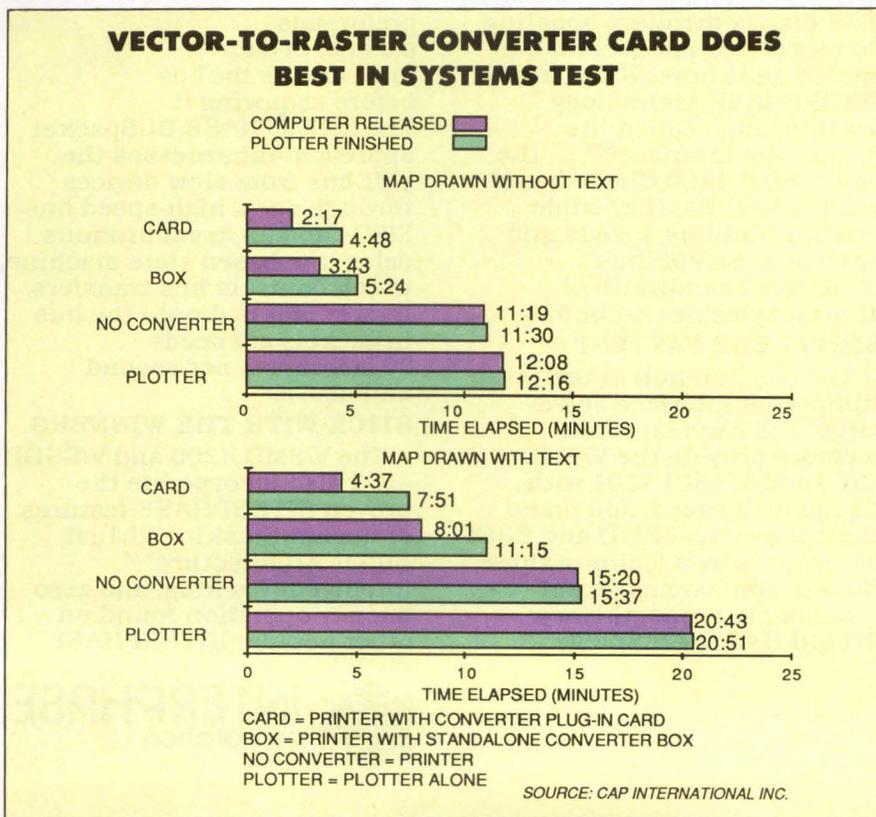
Running an election-analysis mapping program on an IBM Corp. PC/AT, a dot-matrix printer system equipped with a vector-to-raster converter card (CARD) performed best in a test, especially klobbering a plotter system.
