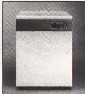
Ridge's proven RISC design provides superior architecture. Plus high performance integer and floating point calculations. 128mb real memory and 4GB virtual memory address space. A UNIX operating system. 18mb/sec input/output. Up to 8GB of file storage. And measured mean time between failure of 16 months.\*
