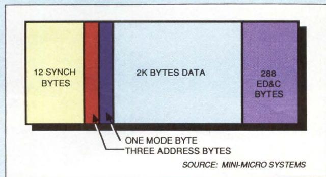
**This example of a CDROM physical format uses spiral-track recording with the data arranged in packets consisting of 12 synchronization bytes, three address bytes, a mode byte and 2K bytes of data, followed by 288 bytes of error-detection and correction.**
