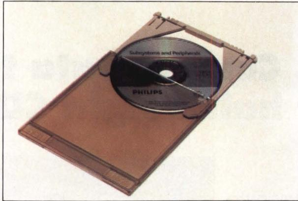
**Laser Magnetic's CDROM caddy** features a protective cartridge that is removable once the disk is in the drive. A sleeve holds the disk in place, allowing the drive to be mounted either vertically or horizontally.
