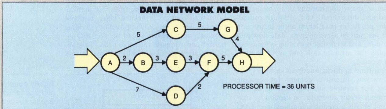
One technique of linking multiple processors in a single machine is to assume a data-networking operation (above). In this approach, each node
