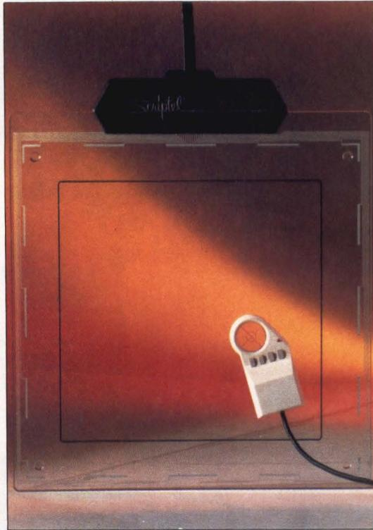
**Combining a transparent digitizer tablet and Chase Systems' ACAD Partner software enables novices to tap the power of Autodesk's AutoCAD package. More than 200 AutoCAD commands are accessible simply by moving the digitizer's stylus and pressing the button.**
