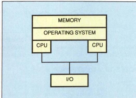
**Tightly coupled, homogeneous architectures** contain identical processors that share a common operating system and memory (left). One such system is the Balance 8000 from Sequent (below).
