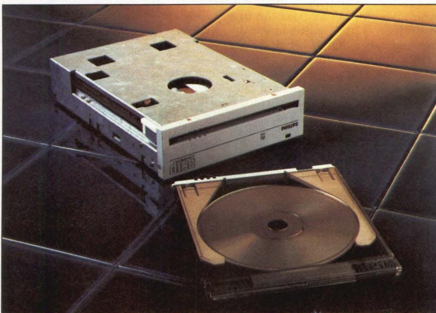
**One Laser Magnetic** half-height CDROM drive comes with a proprietary interface; the other with SCSI. Both read digital and audio disks.
