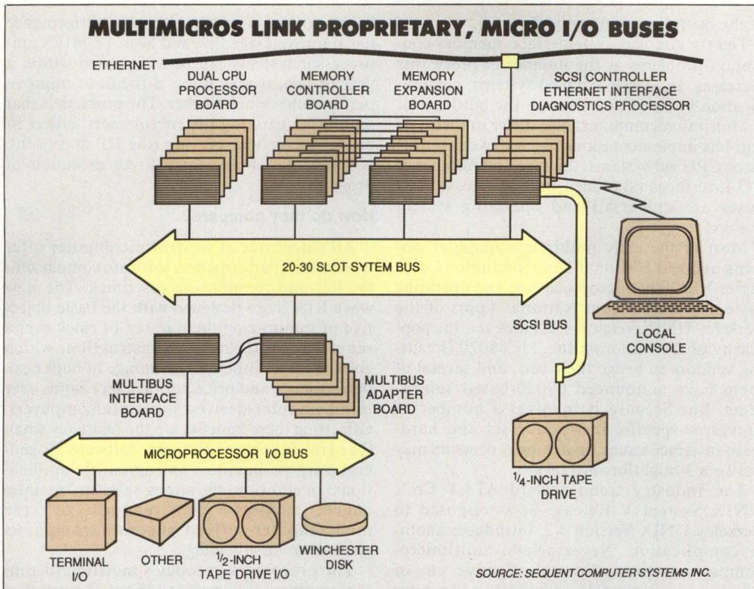
**Multimicro-computer super-minis** connect 20 to 30 processors, I/O and memory subsystems via proprietary system backplane buses, but utilize standard micro-processor buses, such as Multibus and VMEbus, for I/O.
