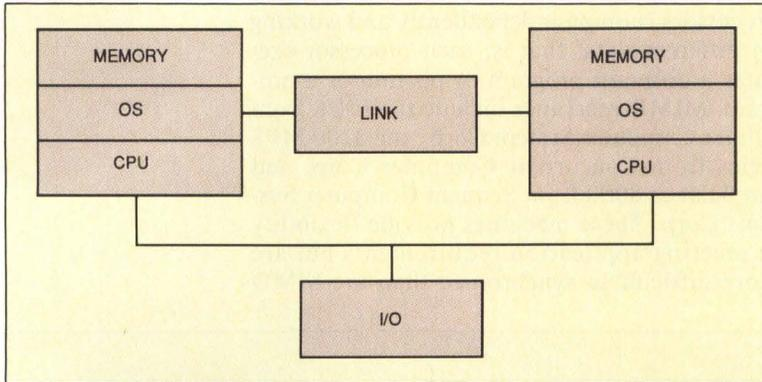
**Loosely coupled architectures** contain self-sufficient processors (above). Diagrammed below is the loosely coupled iPSC from Intel.
