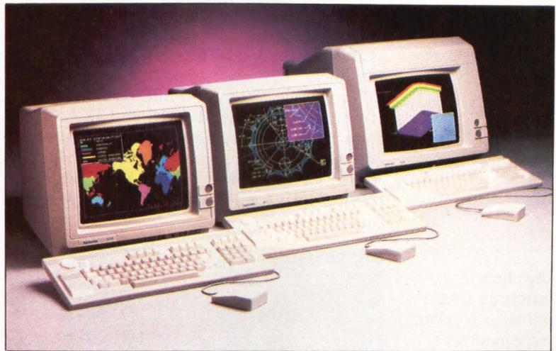
by CGA systems, writing 350 lines for EGA systems requires 21.85-kHz horizontal-scan signals. PGA controllers, featuring 560 raster lines, sweep at 30.48 kHz.
