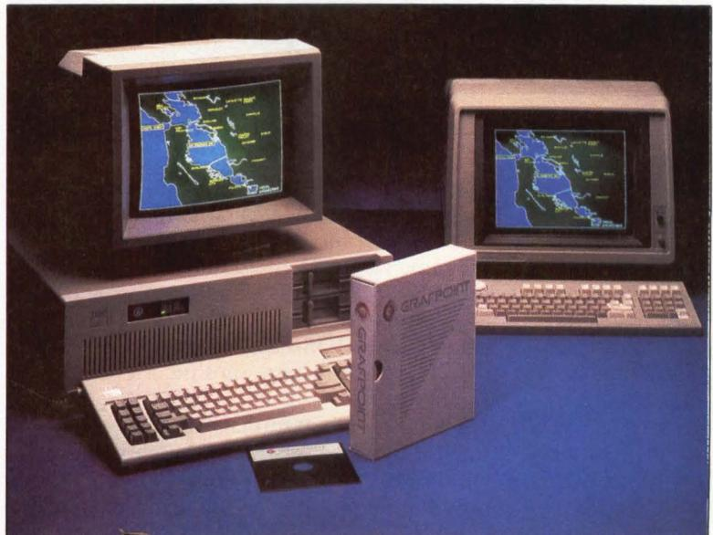
**A 4107 emulator**, Grafpoint's TGRAF-07 allows IBM PCs to access demanding main-frame and minicomputer graphics applications. Here, a map of San Francisco is shown on a PC running the TGRAF-07 package (left) and a Tektronix 4107 graphics terminal (right).
