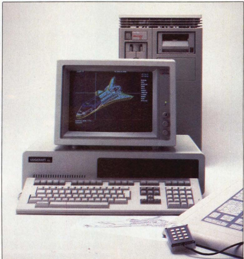
*In a novel twist, the Grafvax from Logicraft allows users of DEC VAX minicomputers to access IBM PC graphics facilities. In combining a terminal emulator with a PC-compatible computer, Grafvax may indicate the evolution of emulators.*
