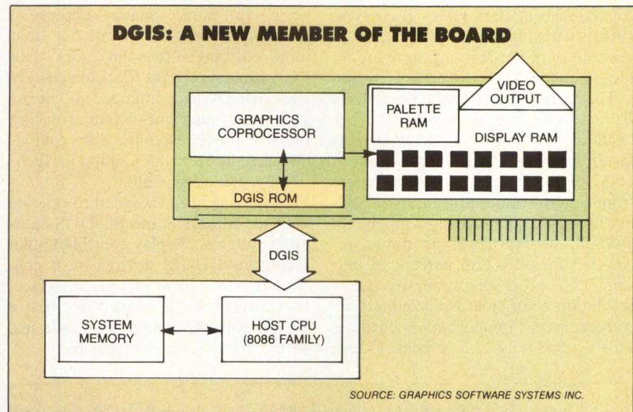
**DGIS is a board-level interface that resides in ROM and works with a graphics coprocessor in IBM PCs and compatibles.**
