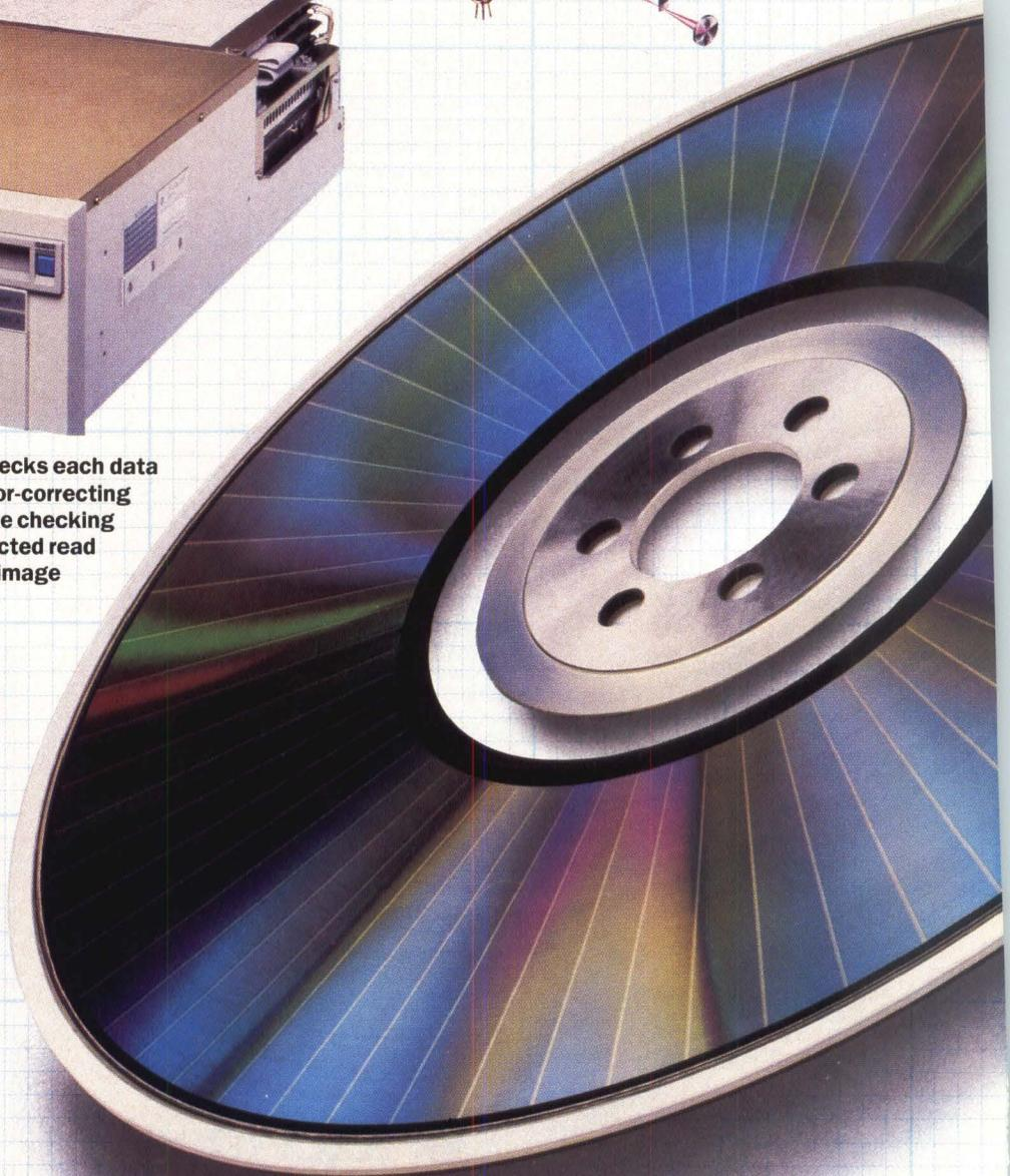
■ The 301's formatter/controller implements either the industry-standard SCSI interface or a GP-IB (IEEE-488) interface, which enables the disk subsystem to be used with a wide range of computers. The unit includes its own memory buffer to speed data transfer between a host computer and the disk drive, which has a 250 millisecond average access time.
