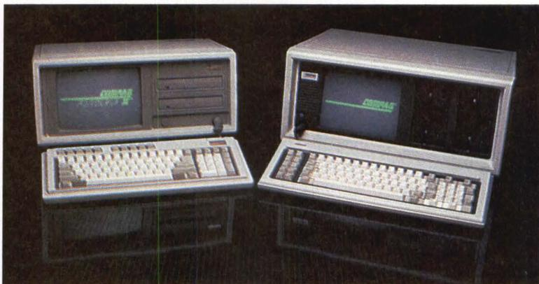
**Incorporating all of the performance and PC-compatibility of the Compaq Portable 286 is the Portable II, smaller and 17 to 20 percent lighter than the earlier machine, depending on the configuration.**
