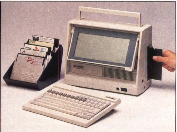
portables (right). The battery-operated laptop contains a Z80 processor and ROM-based software that provides a variety of applications.
