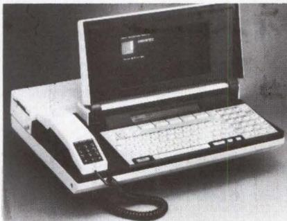
Terminal emulations for TTY, DEC VT100 and IBM-3270 are included in the software. The unit can be hooked to a mainframe computer and is available in three models, and in OEM-quantity prices. \$4,000, The Executive; \$5,000, The Professional and The Secretary. **In-system Inc.**, 450 N. Lakemont, Winter Park, Fla. 32792, (305) 671-2057.
