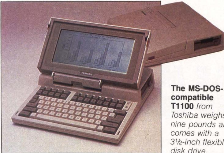
**The MS-DOS-compatible T1100** from Toshiba weighs nine pounds and comes with a 3½-inch flexible disk drive.
