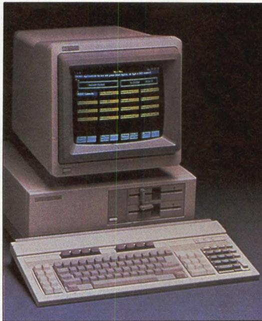
**Offering IBM PC software compatibility,** Hewlett-Packard's Vectra PC is also compatible with HP's minicomputer line.
