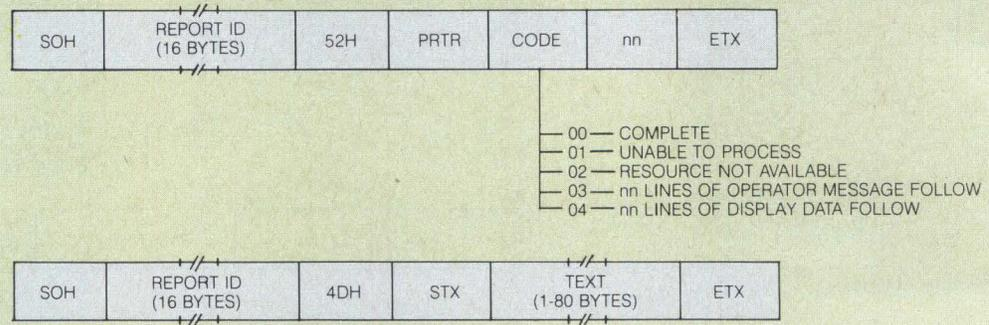
Once a message is sent to the print server, the associated driver processes the command and sends a status response (top) to the IBM PC originating the request. This response tells the originator whether
