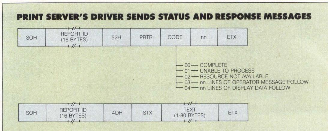
Once a message is sent to the print server, the associated driver processes the command and sends a status response (top) to the IBM PC originating the request. This response tells the originator whether
