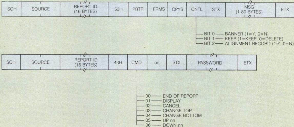
Shipping a file to the server requires a header block (top) to define the source of the file, the report identification and the printer destination. The command for-
