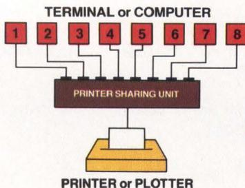
Our 4 or 8 port Printer Sharing Units work automatically. No cable switching or knobs to turn. Software changes are usually unnecessary since they use standard Ready/Busy or XON/XOFF handshaking.
