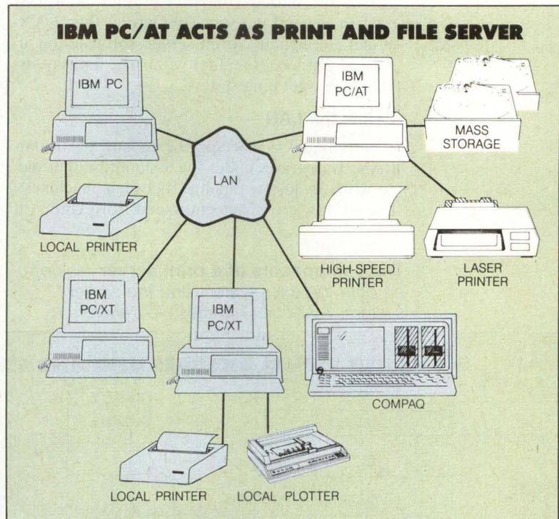
**A typical IBM PC-based network consists of individual PCs acting as intelligent workstations. Each PC can possess local resources, such as rigid disk drives or printers, or, in the case of the IBM PC/AT, act as both a print and a file server.**
