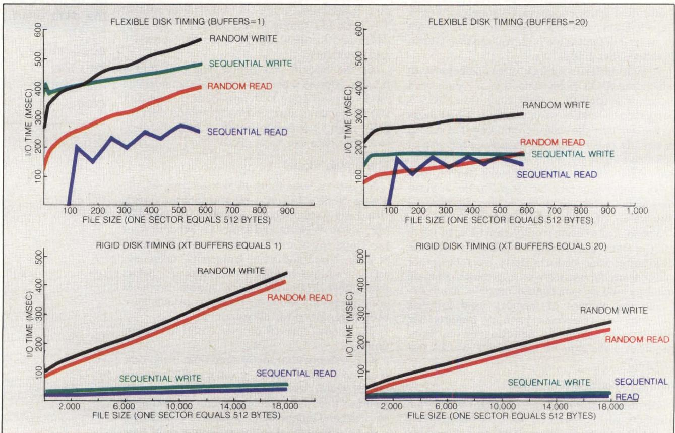
**A change in disk buffer size can affect disk I/O times.** As shown, on an IBM PC/XT with BUFFERS set at 1, I/O processing is slow. Adjusting the BUFFER to 20 speeds
