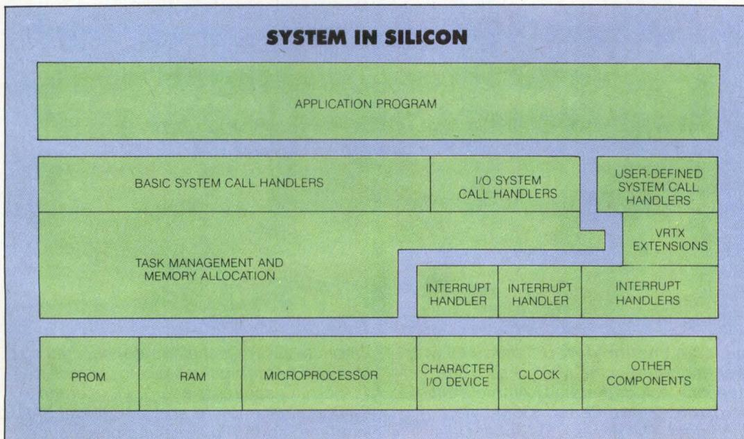
**Fig. 2. The VRTX operating system, embedded in silicon, provides interfaces to user-defined system calls and VRTX extensions. Moreover, VRTX can work as a standalone supervisor by using system event timers and adding user-established controls, such as doing backup while the system isn't being accessed.**
