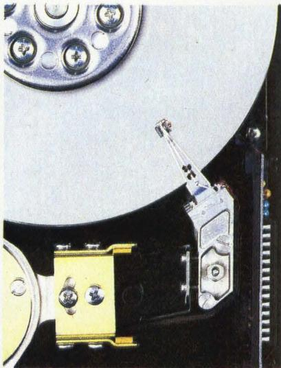
Our new 6190 fixed-disk drive can send the coolest computer pro into raptures. It is easy to see why: A thin-film metal circuit developed by BASF and mini Winchester heads combine to provide a capacity of 94 MB at highest data safety. Thanks to the rotary positioning system, also newly developed, extremely fast data access is assured, together with correspondingly high processing speed to meet severest demands in multi-user/multi-task applications.
