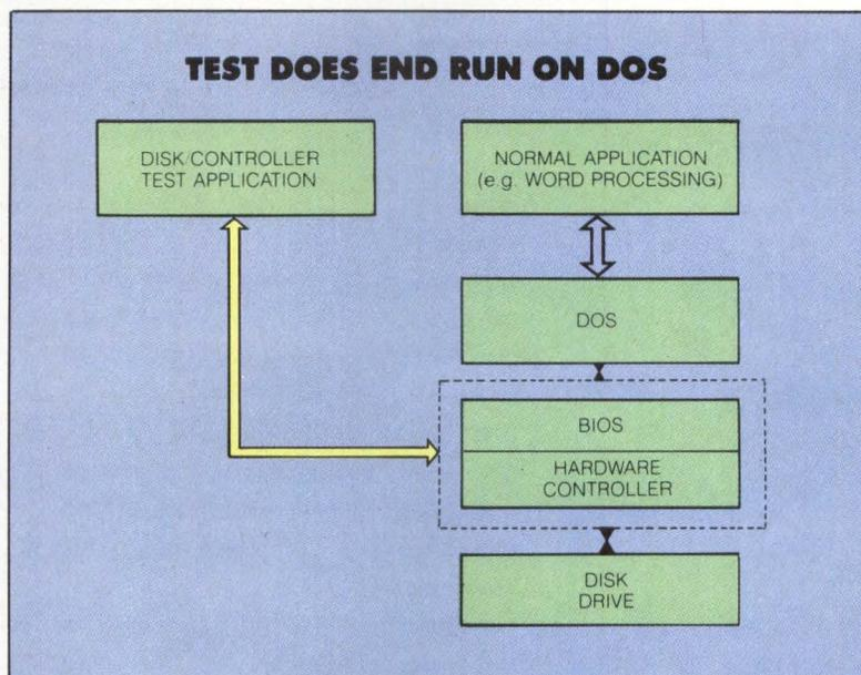
**The disk/controller-test software** bypasses DOS by making direct calls to interrupt 13, the disk-handling routine in the BIOS on the controller ROM. In contrast, a normal application—such as word processing—is filtered through DOS, which makes the BIOS calls.
