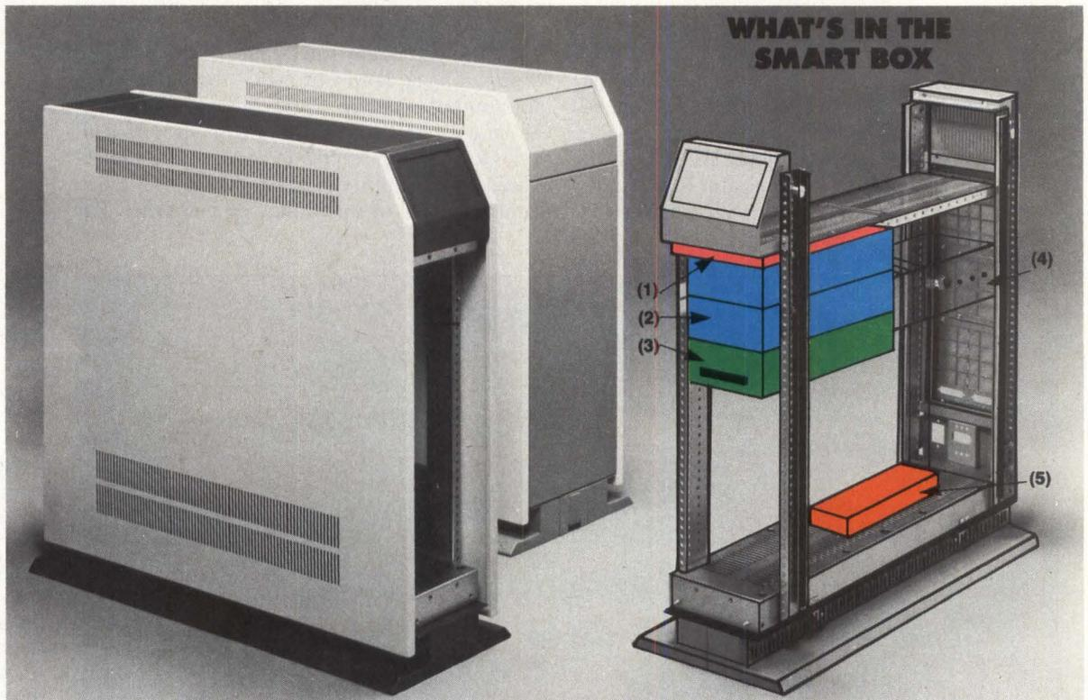
**This is an interior view** of Trimm's OEM tower enclosure in the MMS Smart Box configuration. Included are: (1) Ampro's Little Board/186; (2) two Pertec 330M-byte, 8-inch rigid disk drives; (3) Cipher Data
