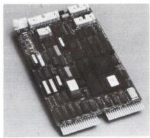
Disk controller interfaces with DEC Q-bus
