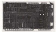
ry. Features include parity checking, EPROM capacity and an 8087 numeric data-processor socket. \$1,800, 128K-byte version; \$2,000, 256K-byte version; \$2,200, 512K-byte version; \$2,550, 1Mbyte version. **Central Data Corp.**, 1602 Newton Drive, Champaign, Ill. 61821-1098, (217) 359-8010.
