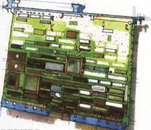
PERTEC tape drives for start / stop and streaming applications. The V/Tape also supports GCR as well as 1600 bpi operations and has ultra fast bus transfer rates at up to 200 ips. Advanced features like 128KB Tape Cache and an on-board 68000 family processor mean it can communicate directly with the INTERPHASE V/SMD 3200 disk controller...cutting your BUS usage in half.
