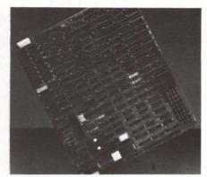
300 dpi, it allows no overlays. Employing the 10-MHz, MC68000 CPU, it includes 384K bytes of DRAM, 32K to 128K bytes of ROM and RS232 serial and Centronics parallel interfaces. Capabilities include pixel addressing, dynamic status monitoring and Qume, Epson MX-80 and Diablo 630 printer emulation. \$500, Q10,000; \$540, Q2,000-5,000. **Electronic Machine Corp.**, Suite 500, 417 S. Hill St., Los Angeles, Calif. 90013-1169, (213) 687-9681.
