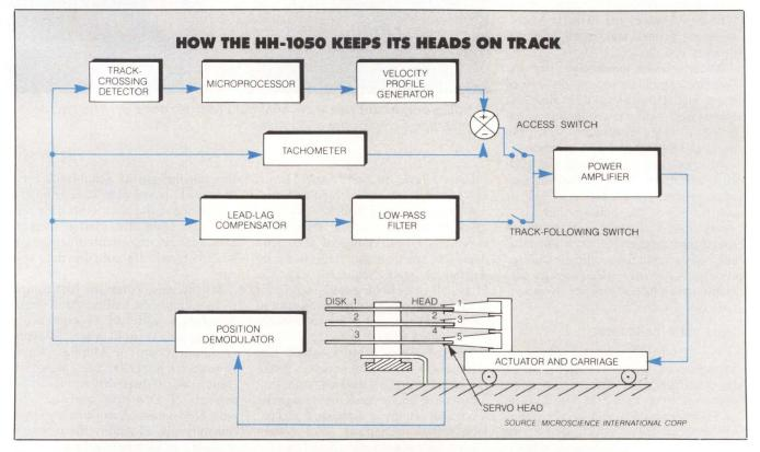
provides a continuous flow of track-positioning data between a dedicated servo on the underside of disk 3
