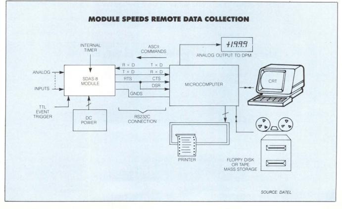
IEEE-488 links relieve system integrators of the task of developing separate interfaces for each connected device. link, the steel-cased 4-by-6-by-0.4-inch unit includes a 12-bit A/D converter, a crystal-controlled clock and direct thermocouple input and linearization. Input data can be transmitted using a TTL trigger, by host ASCII command or controlled by the autostart interval timer. The module also comes as an add-on board with power supply.
