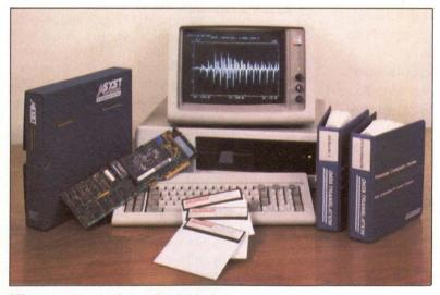
**Microcomputer-based** add-in boards implement real-time data acquisition, analysis and process-control functions under the control of vendor-supplied packages.
