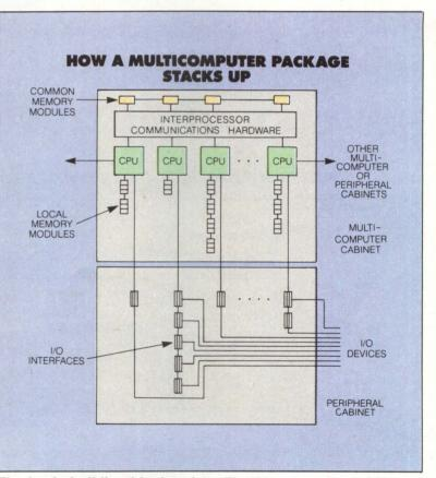
**The basic building blocks** of the Flex/32 are configured for intercommunication. CPUs, computer cards, shared resources and common memory cards are all directly linked by common buses. Individual computers and their local memory modules are connected by local buses. The entire multicomputer system features several individually configurable VMEbus I/O interfaces.
