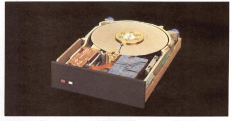
**A voice-coil motor** helps the 50M-byte Microscience HH-1050 achieve an average access time of 35 msec.
