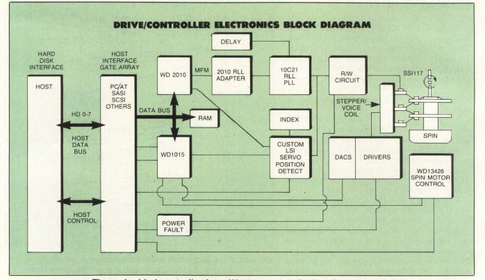
**The embedded controller from Western Digital** combines drive-interface logic and control on a single board. The WD2010 Winchester controller and WD10C20 self-
