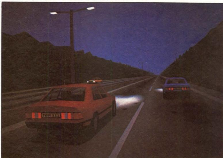
**The Evans and Sutherland CT-5 simulator generated this real-time scene for Daimler Benz of Germany. The simulator provides automobile operators with the ability to test vehicles.**
