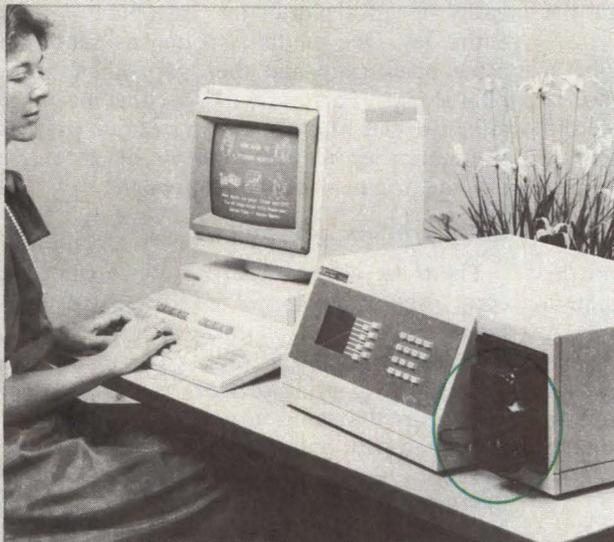
**Using vector technology,** the HP 7510 Color Film Recorder offers a resolution of 16,344 by 10,896 addressable points per 35mm frame. Camera (circled) shown mounted on the HP 7510 is optional.
