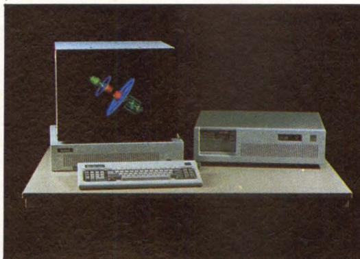
**Ramtek's 2020 display generator**—shown here with an IBM PC-AT—has a 1,280-by-1,024-pixel resolution and interfaces to Apollo, DG, DEC and Control Data computers.
