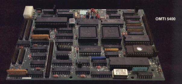
Our OMTI 5400 SCSI (SASI) controller offers Winchester, floppy and tape support all on a single 54" footprint PC board. By using our proprietary VLSI chip technology, we were able to squeeze all these functions onto a board size that most controller companies are still using for single function controllers. This means increased capability and improved cost-effectiveness in your application.
