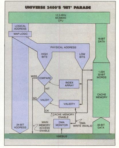
ture and operational capabilities. The characteristics of the VMEbus are well-known in the industry, and CRDS' choice was made easier by the company's extensive experience in using a 32-bit data path. (Its existing products are based on the VMEbus predecessor, the VERSAbus.) The VMEbus' reliability has led to its wide-
