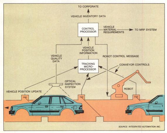
In a typical plant, local controllers drive mechanical devices to control various machines. Information from sensors and other operatorcontrolled inputs helps control the process. The system stores this information and generates reports to management for analysis and transmission to other host computers.
