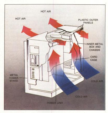
When the Universe 2400 is mounted on its tower stand, its fans draw cool air into the box through filtered vents near the floor. Air is drawn directly over the power supply, through the card cage and out and through the slots near the top of the outer case.
