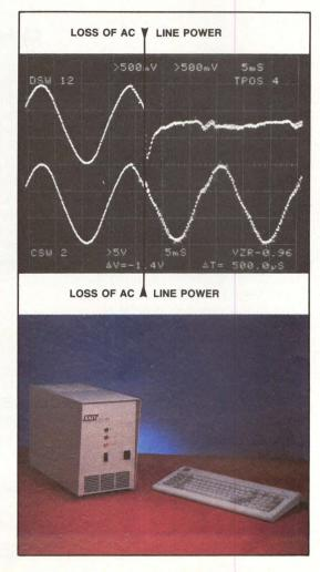
**Transferring** from interrupted AC line power (shown in top trace) to backup battery power in less than 0.5 msec. SAFT America's 1K-VA SPS-1000 standby power system produces voltage-regulated and current-limited sine-wave output (bottom trace) to support the load when a power failure occurs.
