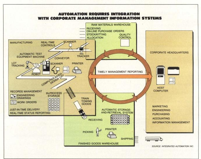
In the "factory of the future," factory scheduling and database interfaces will fit smoothly with installed MIS equipment. Companies often use an area host computer to coordinate plant operations, including controlling production lines, robots and numerically controlled machines. Driven by information generated from the raw materials warehouse, manufacturing facility and finished goods warehouse, the central corporate computer can provide a daily log of company-wide activity.
