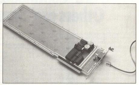
**With Intel's 82588** controller, here's all the circuitry needed to connect an IBM PC to a Starlan network. The chip supports network standards proposed by both IBM and AT&T.
