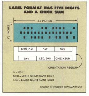
A bar-code reader uses line-by-line scanning to build an image of a label. The label includes a five-digit code, a checksum digit and an orientation region that enables the scanner to recognize the label's position.
