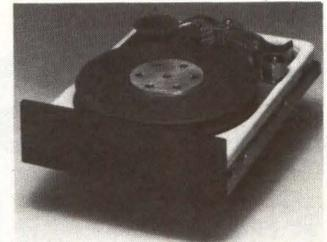
closed-loop servo positioning system. With a track density of 720 tpi, the drive stores 20M bytes. With a recording density of 9,036 bpi, the drive achieves an 85-msec average access time and a 5M-bps transfer rate. The printed circuit board includes four LSI devices and two 8-bit microprocessors. The read/write head is positioned with a stepper motor/band actuator system. \$500, OEM quantities. **Shugart Corp.**, 475 Oakmead Pkwy. Sunnyvale, Calif. 94086 (408) 733-0100. **Circle No 308**
